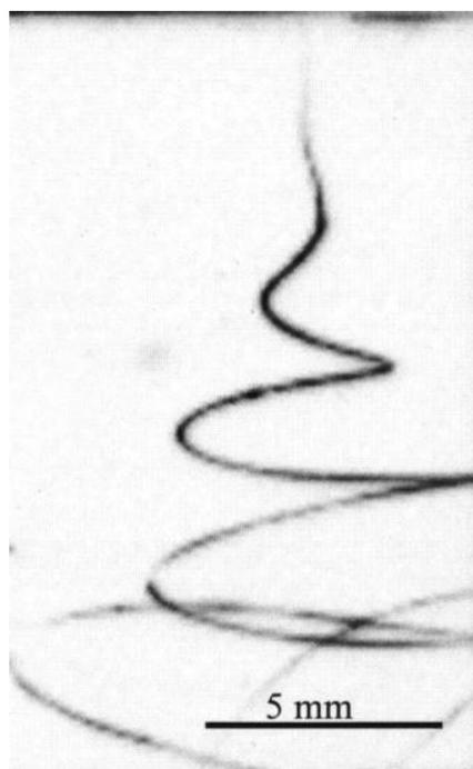
**Figure 3-6 Charged jet bending under instability [83].**
