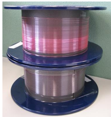
Fig. 5-2 (b). Photo of dye-doped POFs where the fibre in the top reel is doped with Rh640 and the bottom reel with LDS751.
