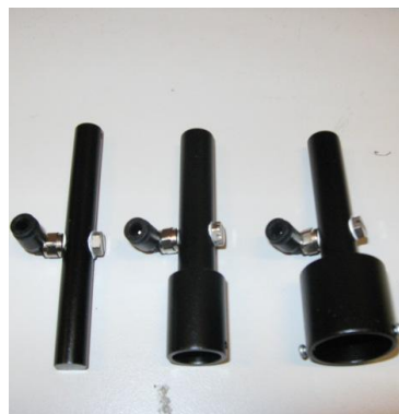
Fig.4-4. Photo of preform adaptors with different sizes, integrated with gas fittings.
