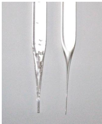
Fig. 3-2. Photo of (left) preform with MMA:BMA ratio of 90:10 and (right) preform with MMA:BMA ratio of 75:25.
