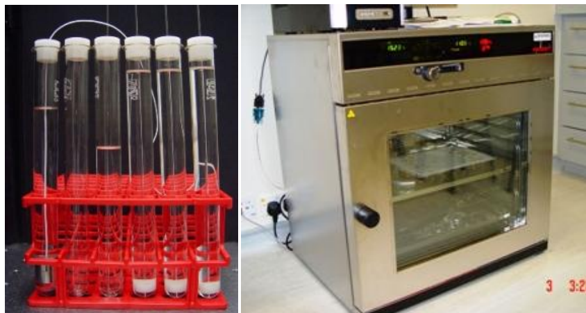
Fig. 3-7. Photo of (left) glass test filled with monomers mixture and (right) computer controlled oven.
