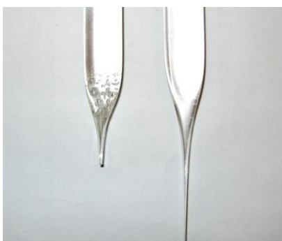
Fig. 4-11. Photo of (left) preform under too high furnace temperature and (right) preform drawn with suitable temperature.
