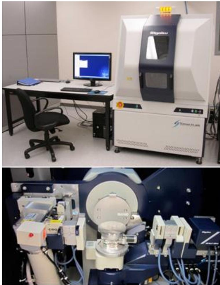
Fig. 2.6 The Rigaku automated multipurpose Smartlab X-ray diffractometer.
