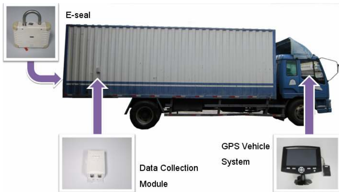
Figure 4.6 Deployment of RFID-based Tracking and Monitoring System
