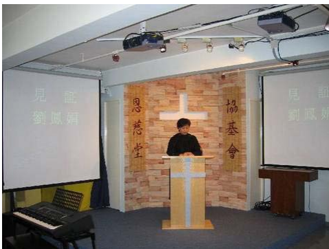
Figure 4.46 Use of two projection screens on the sides could solve the problem of covering the cross in the middle. (Retrieved on 1 July 2007, http:// www.yantze-church.org )
