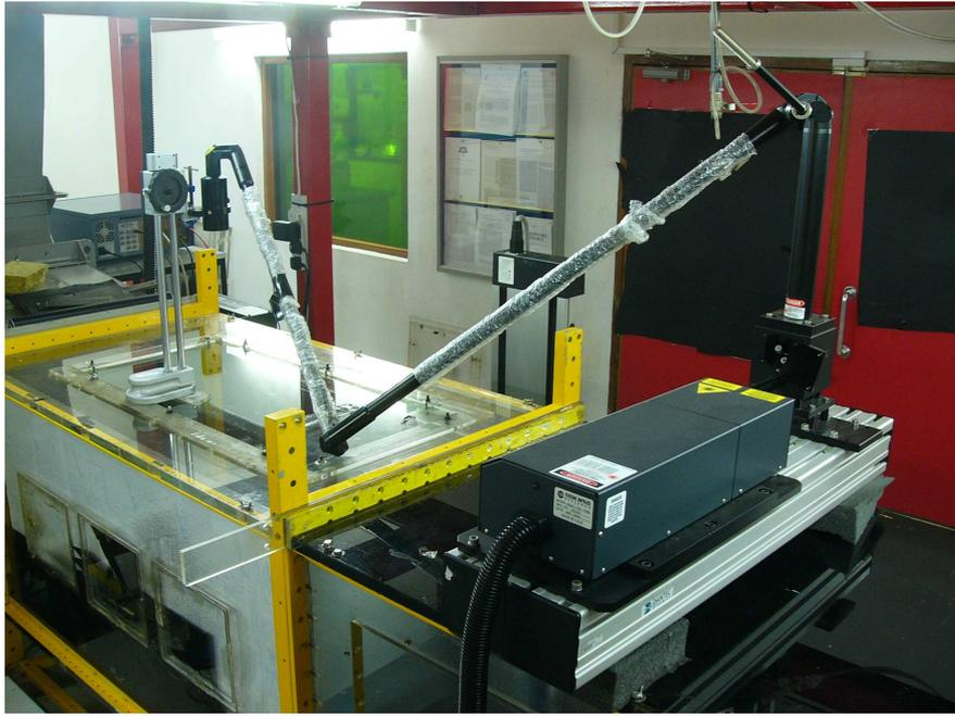
Figure 3.9(a) Laser and optical arm used to deliver the light sheet into the wind tunnel for the illumination of seeding particles.
