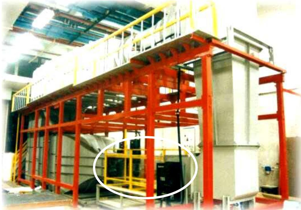
Figure 3.1 Closed circuit wind tunnel facility used for the present research. The circled yellow rectangular frames with transparent acrylic walls are the test section.
