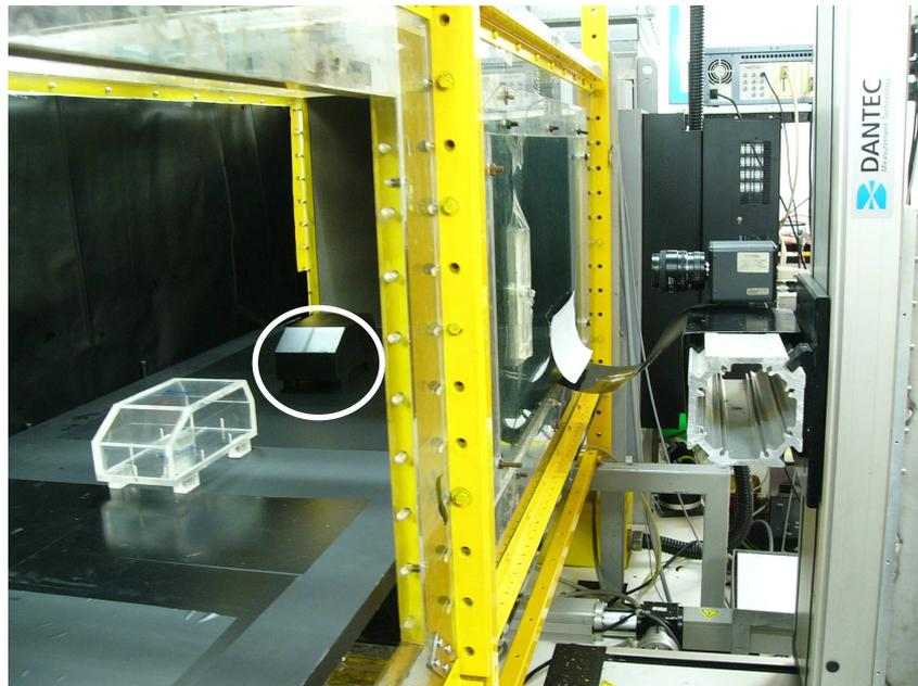
Figure 3.9(b) A CCD camera was placed outside the test section of wind tunnel to capture the images of a two-dimensional flow field around the last vehicle, V1 (enclosed by the white circle) which was painted in black to minimize its noise laser reflection.
