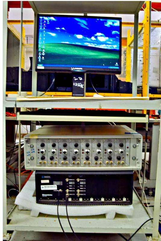
Figure 3.14(a) Dantec StreamLine hot-wire anemometer (the bottom black box) and the cold-wire anemometer (the upper silver box) used in the present study.
