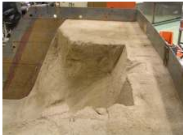
(d) global failure surface after failure mass is removed
