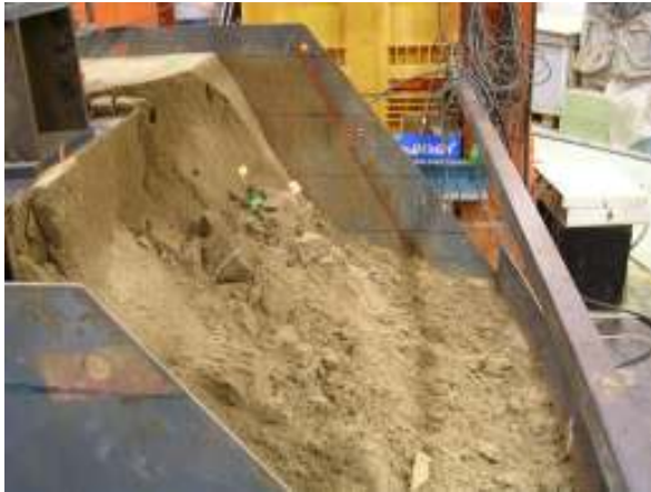
(1) Lab test of slope without soil nail
