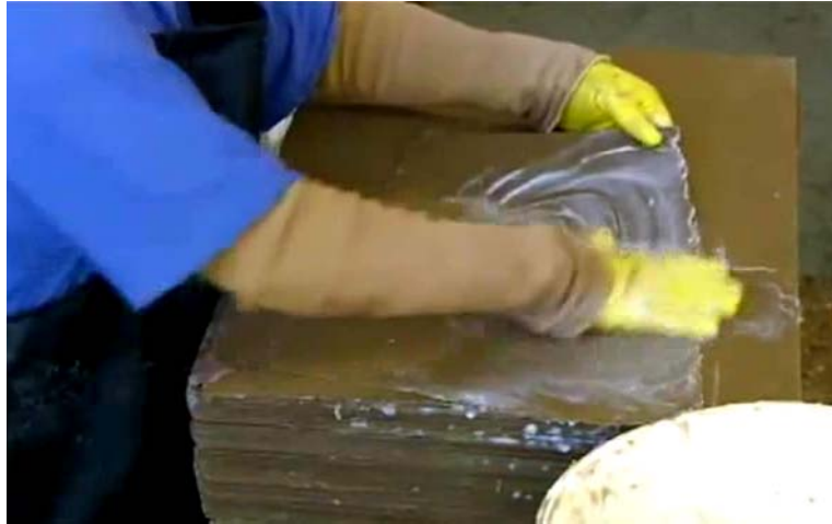
Figure 2-15. Coat the wet card boards with plaster and glue.
