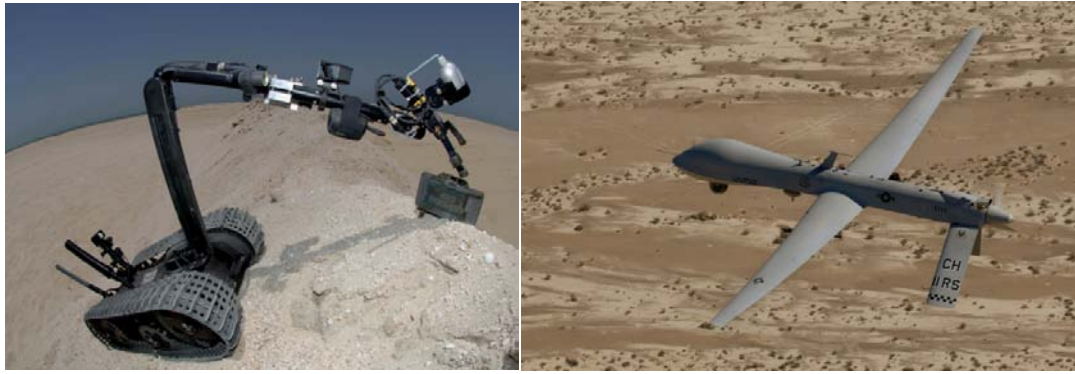
Figure 2-24. Left: A Talon 3B robot unit removes a mine. Right: A MQ-1 Predator equipped two laser-guided Hellfire anti-tank missiles.
