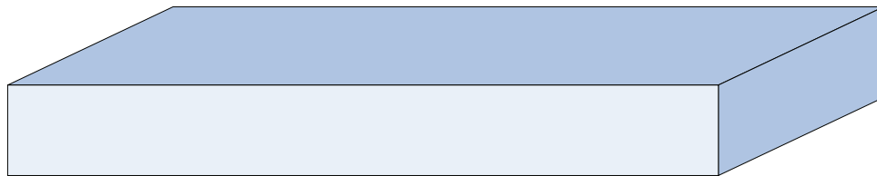
(a) Ceramic duplexer 5.5 \times 24.5 \times 5 : 674mm^3
