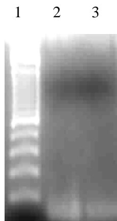
Figure 3.16 Gel electrophoresis image of the amplification results of CFPCR with different durations using syringe pump. Lane 1 is DNA size marker; lanes 2 and 3 are CFPCR of 32 and 20 min, respectively.
