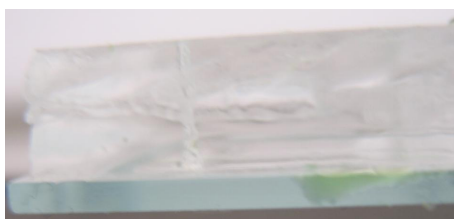
Figure 3.8 A photograph showing the leakage of PCR reagents during the CFPCR. The green PCR reagents leaked out through the space between the glass and PDMS.
