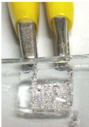
Figure 3.1 A photograph showing the gas bubbles generated by the electrolytic pump.
