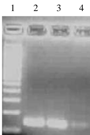
Figure 3.14 Gel electrophoresis image of the amplification results of CFPCR with dynamic passivation using different concentrations of BSA. Lane 1 is DNA size marker; lanes 2, 3, and 4 are CFPCR with 2, 0.5, and 0 \mu\text{g}/\mu\text{L} BSA.
