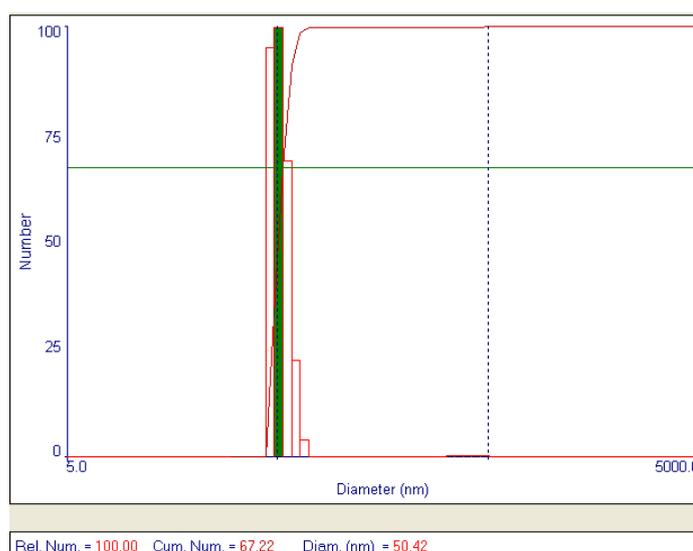
Figure 4.2 Particle size distribution of SF nanoparticles dispersed in ethanol
