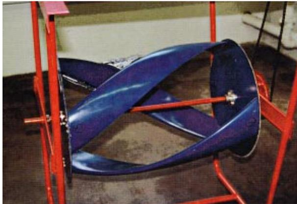
Figure 2.36 Helix or helical Darrieus tested by the Gorlov (2001)
