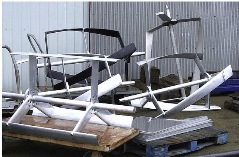
Figure 2.38 The straight and helical Darrieus rotors tested by the Kirke (2011)
