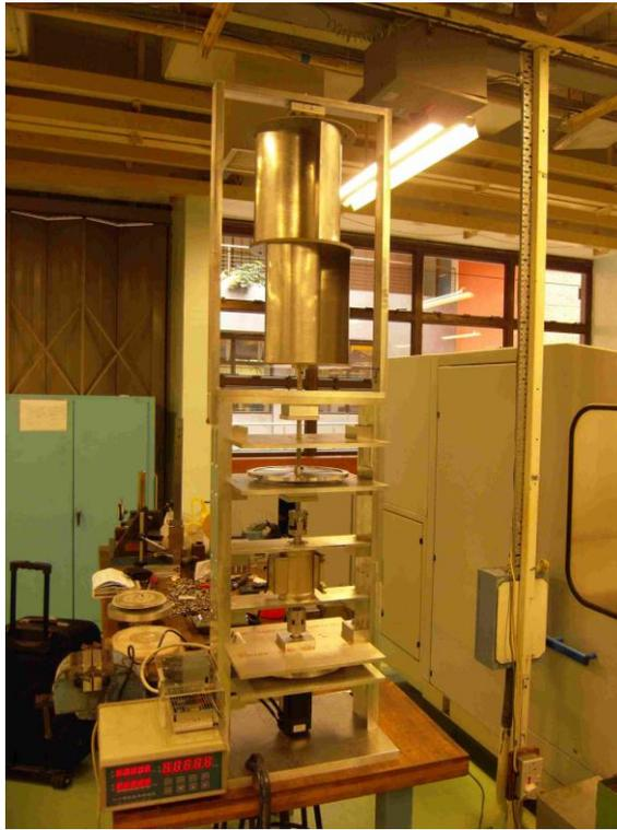
Figure 2.28 A vertical testing rig
