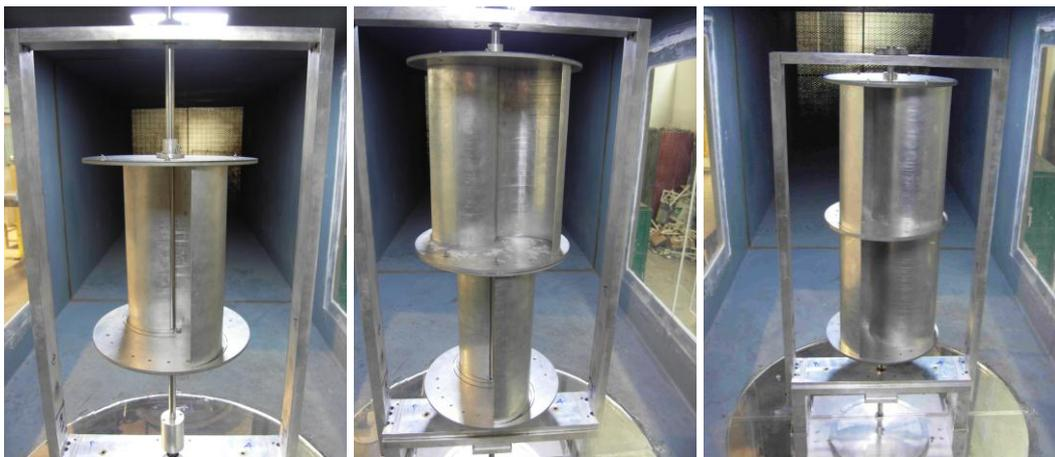
Figure 3.15 The real rotors with two and three blades
