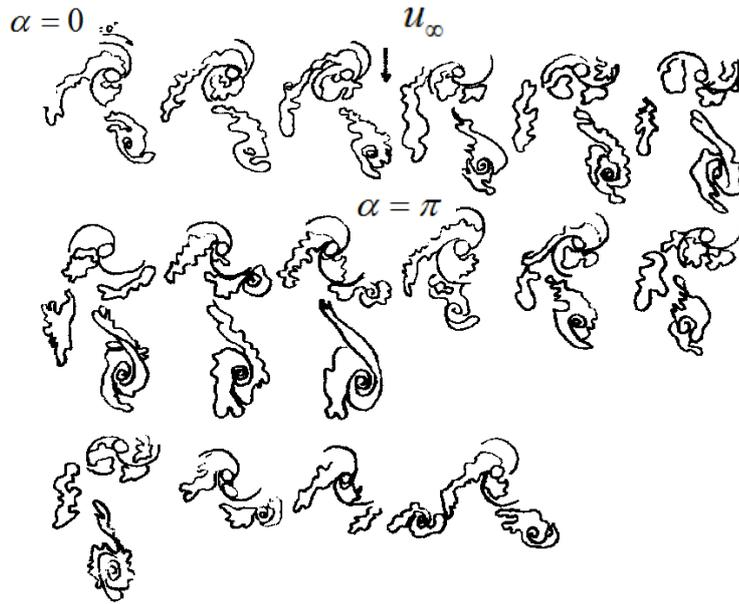
Figure 2.25 The vortices generated by the Savonius rotor (Benghrib et al, 1998)
