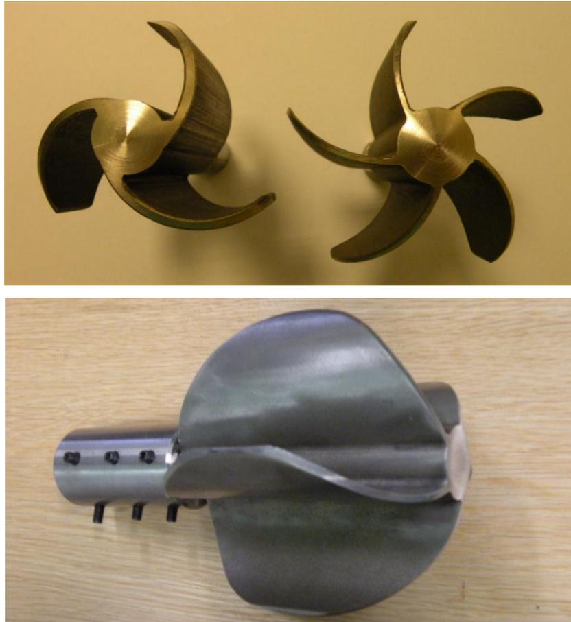
Figure 0.6 CNC turbine models (Appendix B)
