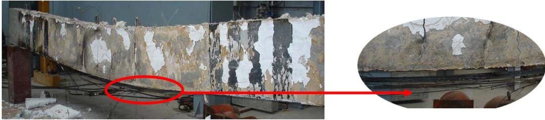
**Fig. 2.7** Appearance of CFRP sheets-strengthened RC beams after the removal of the insulation materials (Gao et al. 2010)
