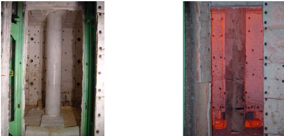
**Fig. 2.8** Insulated FRP-strengthened concrete column before and after fire testing (Bisby et al. 2005b)
