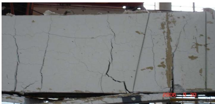
**Fig. 2.6** Cracking of calcium silicate cladding boards (Gao et al. 2010)
