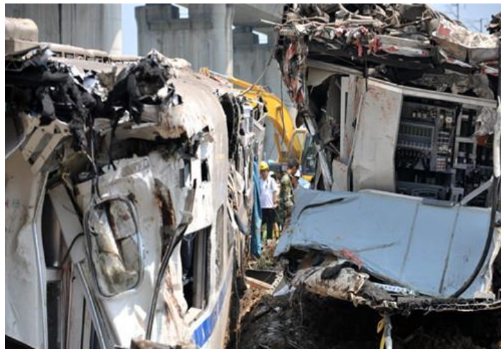
Figure 3 Bullet trains destroyed in the accident on July 23, 2011 (The accident was caused by the breakdown of the power supply system and the communication system due to the lightning strikes)
