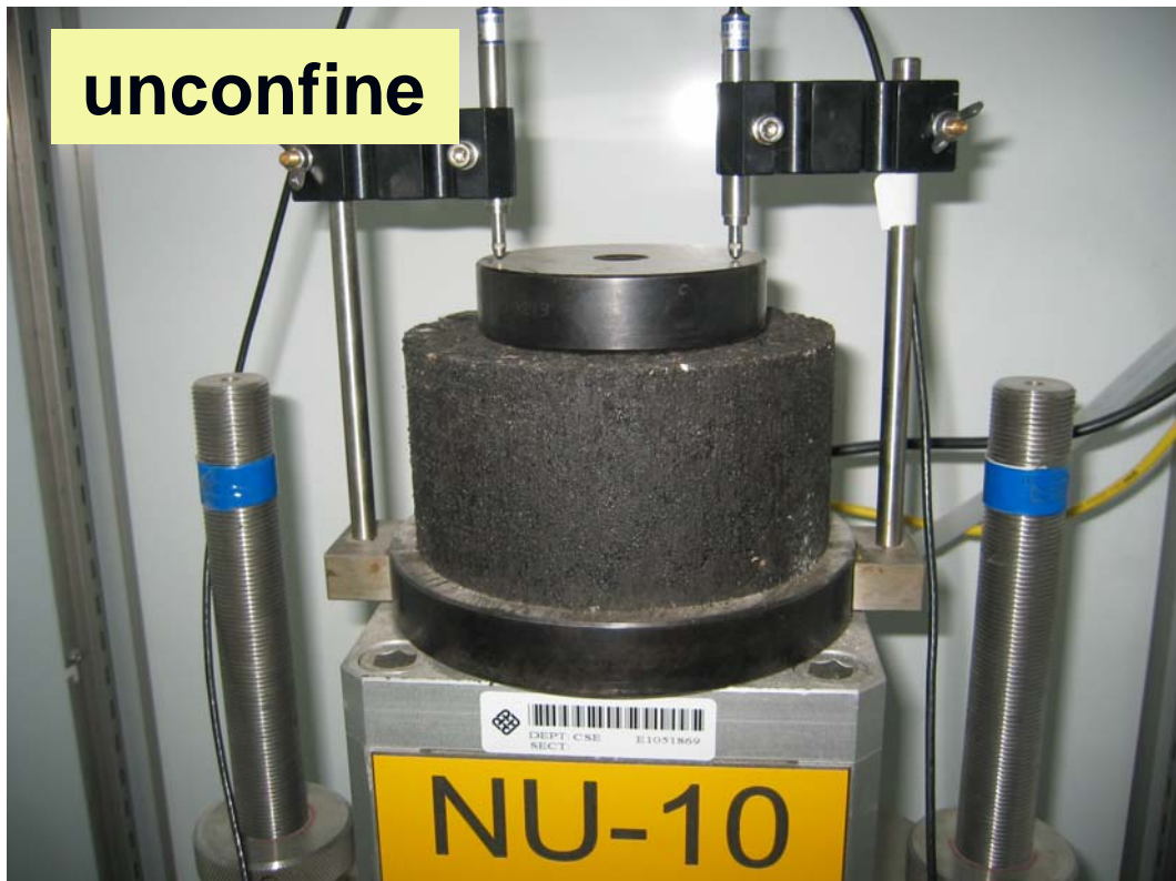
Picture 5-3 The Apparatus for Dynamic Creep Test
