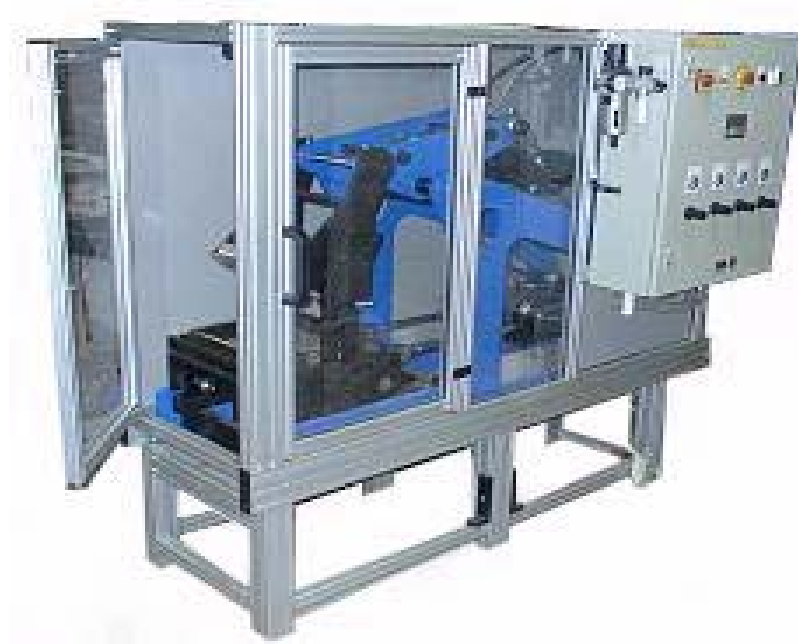
Picture 3-7 Roller Compactor
