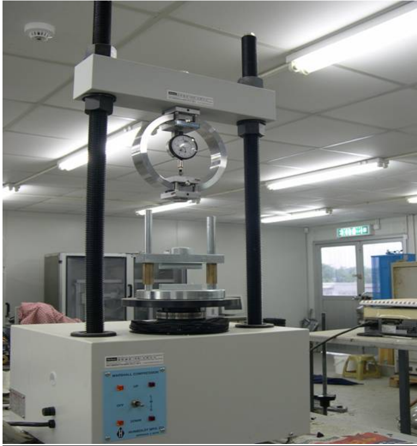
Picture 5-6 The Apparatus for ITS Test
