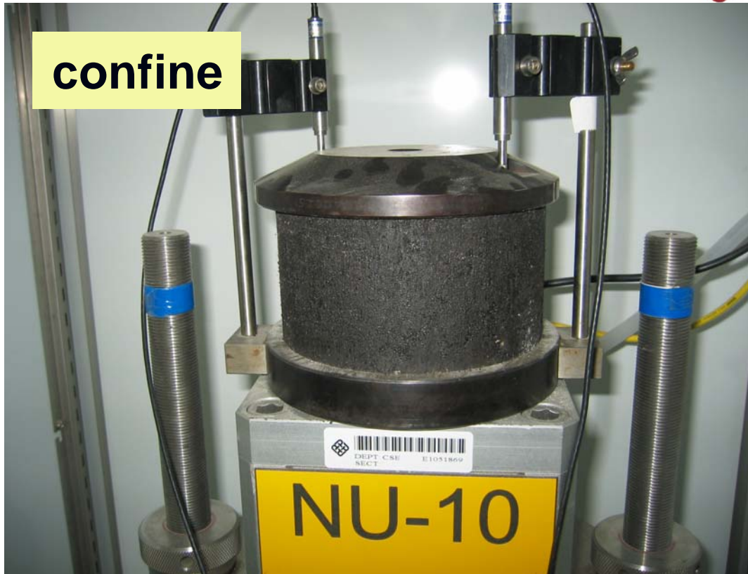
Picture 5-4 The Apparatus for Indentation Creep Test
