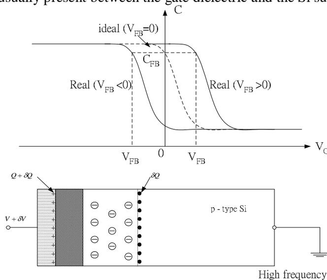
Figure 2.4.1 High frequency  $C-V$  curves and MOS block diagram.
