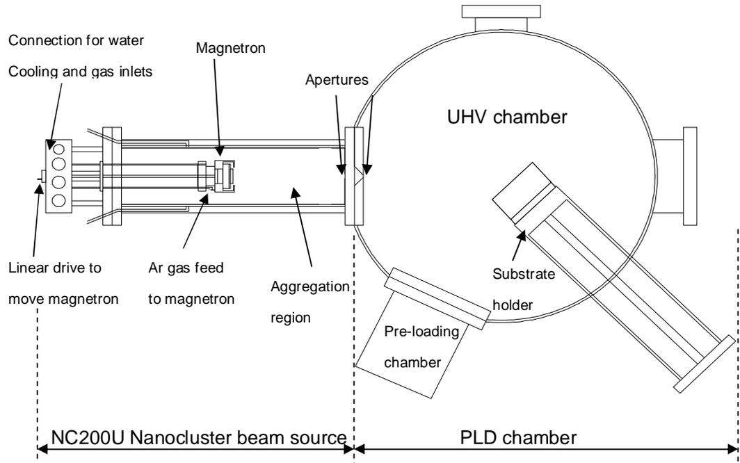
Figure 4.2.3 Schematic layout of the nanocluster beam source with laser molecular beam epitaxy vacuum chamber system.
