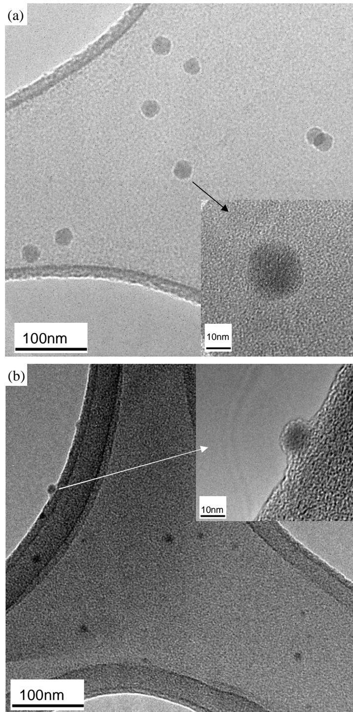
Figure 4.3.3 TEM images of low density and small mean diameter Ge nanocrystals formed by nanocluster source under the following condition: 300 °C, 30 W, 30 sccm. (a) 100 mm, and (b) 60 mm.
