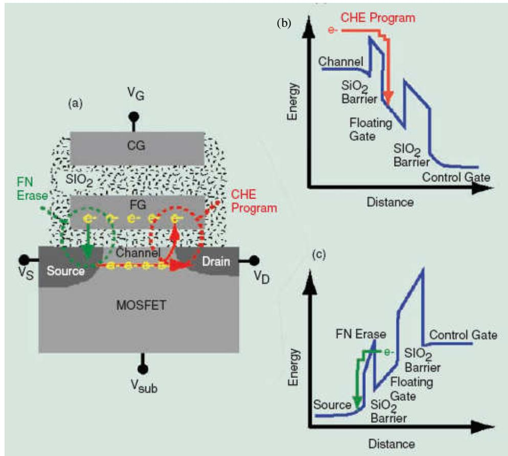
Figure 2.5.1 (a) Schematic of a basic ETOX (EPROM Tunnel Oxide) flash memory device showing the program and erase operations. (b) Electron flow during programming by CHE injection. (c) Electron flow during erasing by FN tunneling to the source. [57]
