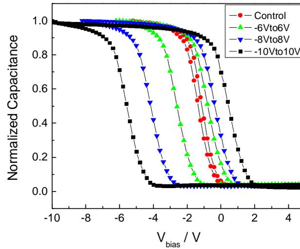
Figure 4.3.6 High frequency (1 MHz)  $C$ - $V$  measurements of the trilayer floating gate capacitors with and without Ge deposition. Large counter-clockwise hysteresis loop up to  $\Delta V_{FB} = 6.0$  V can be observed in the sample of 15-min Ge nanocluster deposition. All samples are normalized with accumulation capacitance of 0.15 nF.
