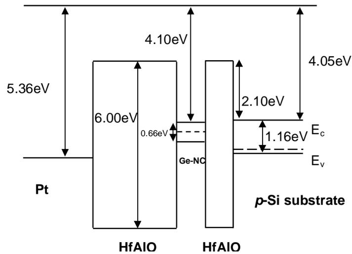
Figure 1.2.1 Energy band diagrams of the Ge nano-floating gate structure at flat-band condition [60].
