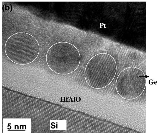
Figure 3.3.5 High-resolution TEM images of samples composed of HfAlO control gate, Ge nanocrystals, and HfAlO tunnel layer on Si substrate: (a) as-grown, and (b) annealed at 800 °C.
