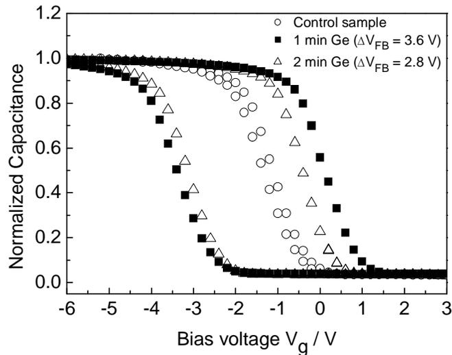
Figure 3.4.2 High frequency (1 MHz)  $C$ - $V$  measurements of the trilayer floating gate capacitors with 1 and 2 min Ge deposition time and control sample without Ge nanocrystals. All samples have been annealed at 800 °C in  $N_2$  ambient for 45 minutes. Large counter-clockwise hysteresis loop up to  $\Delta V_{FB} = 3.6$  V can be observed in the sample with Ge nanocrystals. All samples are normalized with accumulation capacitance of 0.15 nF.
