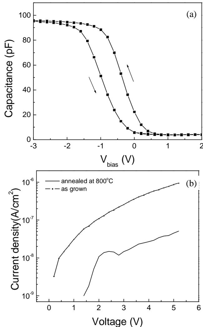
Figure 3.3.6 (a) High frequency (1MHz)  $C$ - $V$  curves, and (b)  $I$ - $V$  curves of as-grown and 800 °C annealed MOS capacitors.
