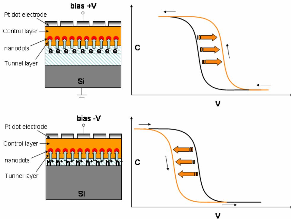
Figure 2.4.2 Diagram of a C-V curve of a nano-floating memory capacitor. Counter-clockwise loop represent an electron injection from the Si substrate.
