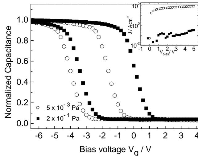
Figure 3.4.4 High frequency (1 MHz)  $C$ - $V$  characteristics of the trilayer floating gate capacitors with HfAlO growth oxygen partial pressures of  $5 \times 10^{-3}$  and 0.2 Pa. All samples have been annealed in  $N_2$  ambient for 45 min. Inset is the  $I$ - $V$  characteristic of the samples. The sample with growth oxygen partial pressures of  $5 \times 10^{-3}$  Pa shows a higher leakage current density. All samples are normalized with accumulation capacitance of 0.15 nF.
