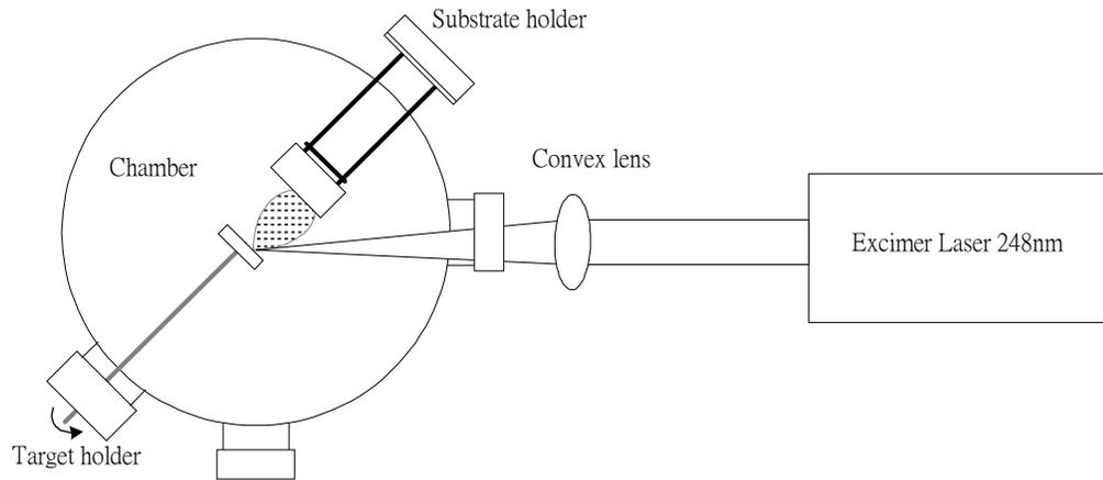
Figure 2.1.1 Schematic diagram of the PLD setup.
