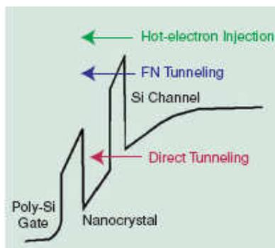
Figure 2.5.3 Energy band edge schematic illustrating direct quantum mechanical tunneling compared to other injection mechanism.[57]
