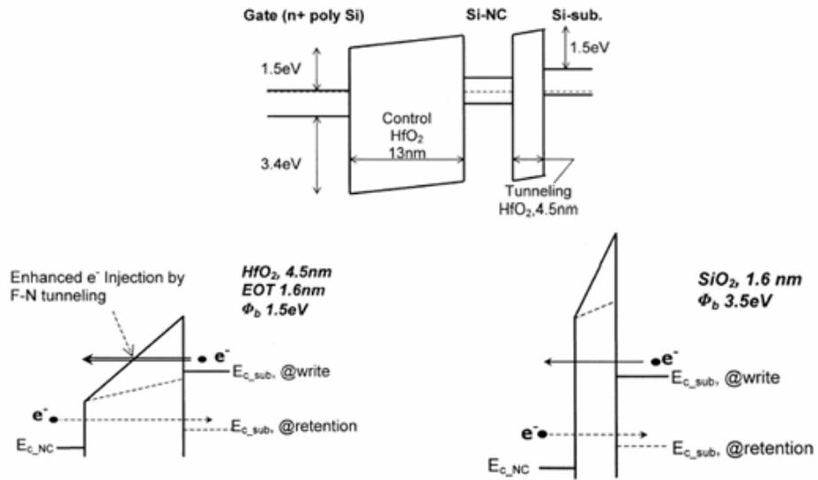
Figure 1.2.2 Energy band diagram of Si nanocrystal memory with HfO<sub>2</sub> at equilibrium, and enlarged conduction band-edge profile of Si nanocrystal/tunneling dielectric/Si substrate of (a) HfO<sub>2</sub>, (b) SiO<sub>2</sub>, at writing mode. Dashed lines in (a) and (b) indicate conduction band edge profile at data retention. [47]
