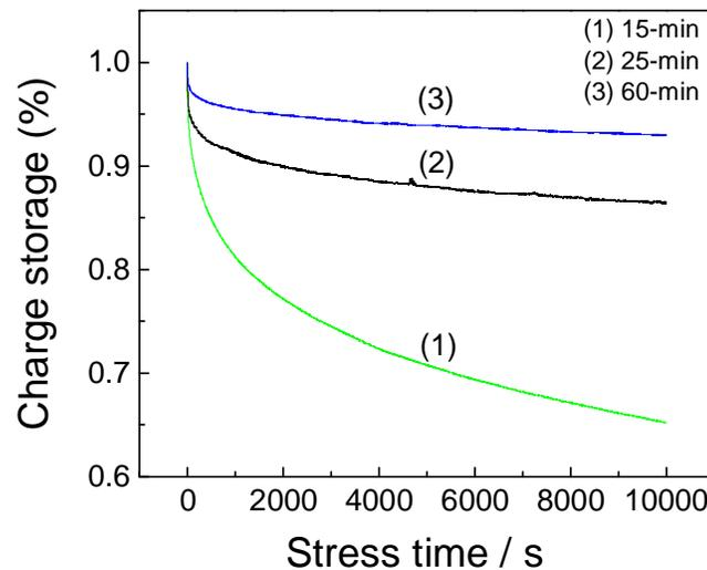
Figure 4.3.8 *C-t* characteristics of the trilayer floating gate capacitors with: (1) 15-min, (2) 25-min, and (3) 60-min Ge nanocluster deposition. The charging voltage is 10 V for 20 s and the measurement voltage is -1 V.
