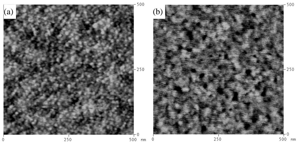
Figure 3.3.2 AFM images of Ge nanocrystals on HfAlO/Si matrix by PLD for 30 s at (a) 600 °C and (b) 700 °C.
