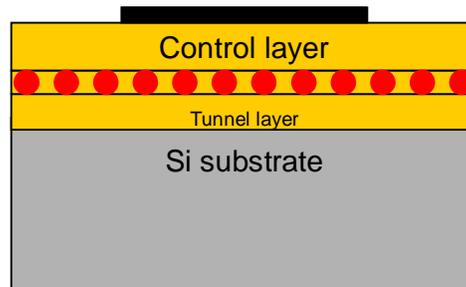
Figure 3.2.1 Schematic diagram of the trilayer nano-floating gate memory MOS capacitor.
