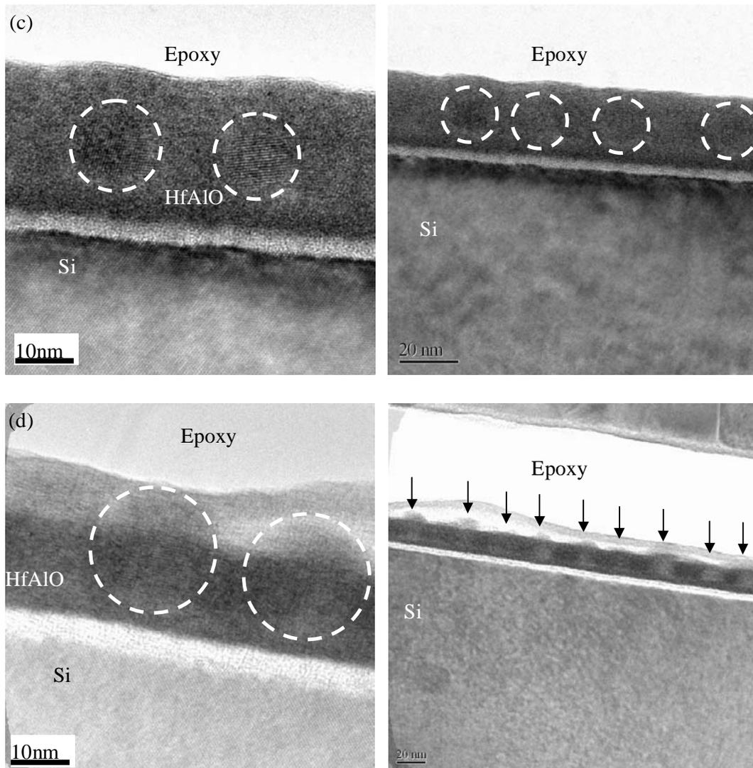
Figure 3.3.4 TEM images of the trilayer floating gate capacitors with different Ge deposition time: (a)30 s, (b)1-min, (c) 2-min , (d) 3-min. The dot-circle region and/or the arrow indicate that Ge nanocrystals are formed within the HfAlO matrix.
