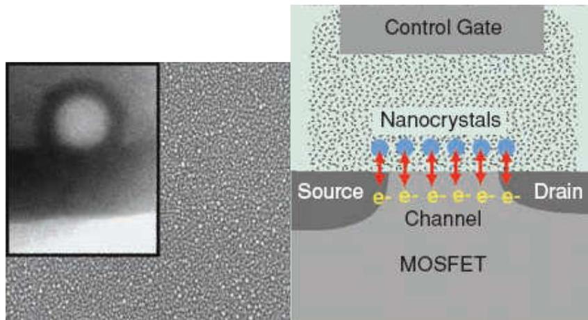
Figure 2.5.2 (a) A scanning electron micrograph of dense Si-nanocrystal coverage required for reliable flash memory operation. Inset: An energy-filtered transmission electron micrograph of a single nanocrystal, encapsulated in an oxide shell, on a tunnel barrier. (b) An illustration of a nanocrystal floating gate memory. [57]
