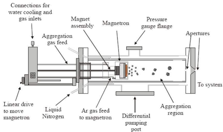
Figure 4.2.1 Schematic diagram of the nanocluster source (NC200U) system.
