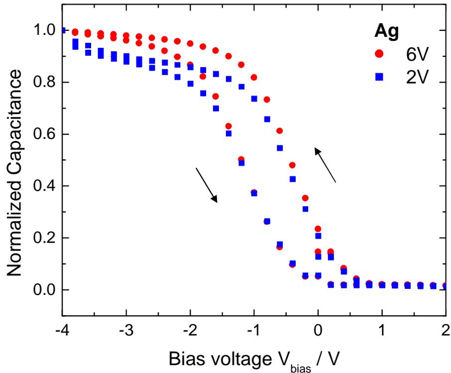
Figure 5.3.4 High frequency  $C$ - $V$  measurement with (a) +6 V forward and -4 V reverse bias voltage and (b) +2 V forward and -4 V reverse bias voltage.
