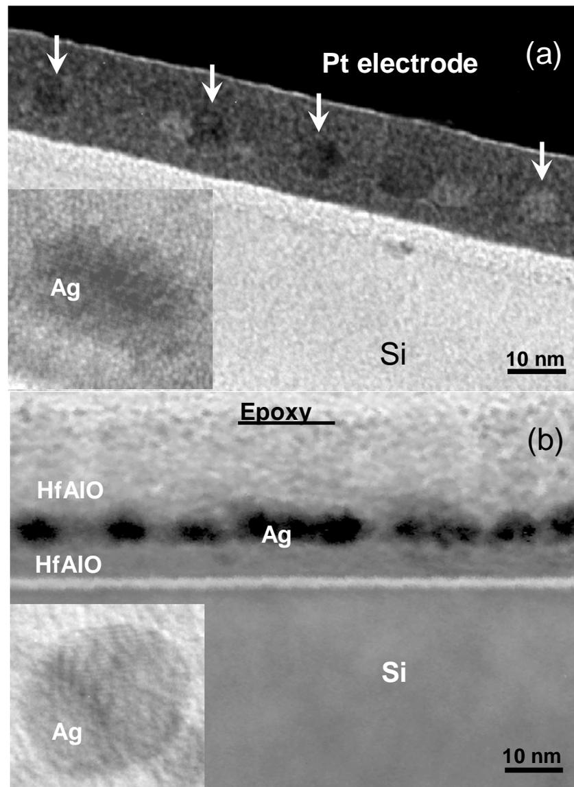
Figure 5.3.2 HRTEM images of the trilayer floating gate capacitors: (a) 2-min, and (b) 5-min Ag deposition.
