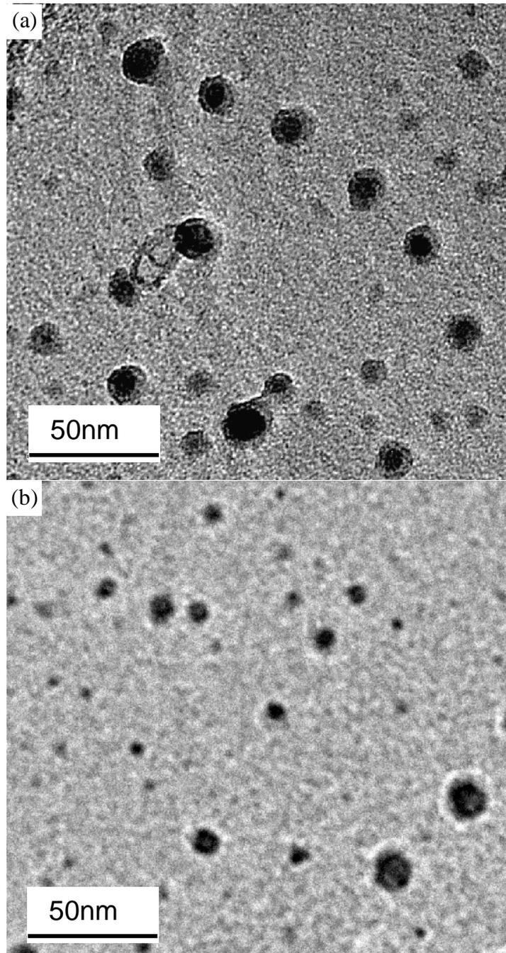
Figure 4.3.2 TEM images of Ge nanocrystals formed by nanocluster source. Both samples are grown at 600 °C with sputtering power of 40 W, and fixed magnetron-to-aperture distance of 100 mm. Only the sputtering gas flow rate is different: (a) 40 sccm and (b) 30 sccm.
