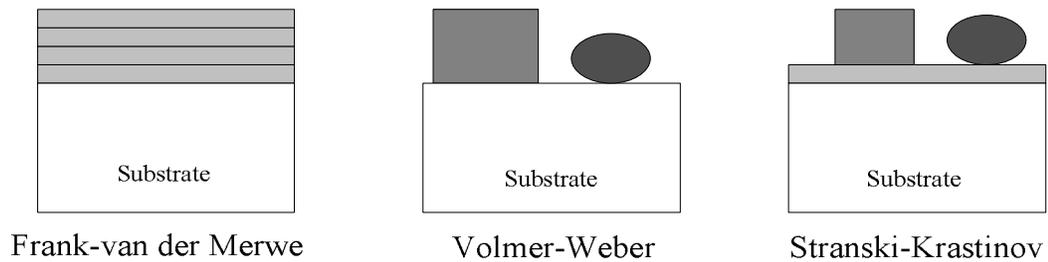
Figure 2.1.2 Three modes of film growth [6,8-9]. Layer-by-layer (Frank-Van der Merwe) growth consists of deposition of one monolayer at a time and results in a very smooth epitaxial film. Island (Volmer-Weber) growth results in the formation and growth of isolated islands. Mixed (Stranski-Krastanov) growth consists of island growth after the first monolayer forms successfully.
