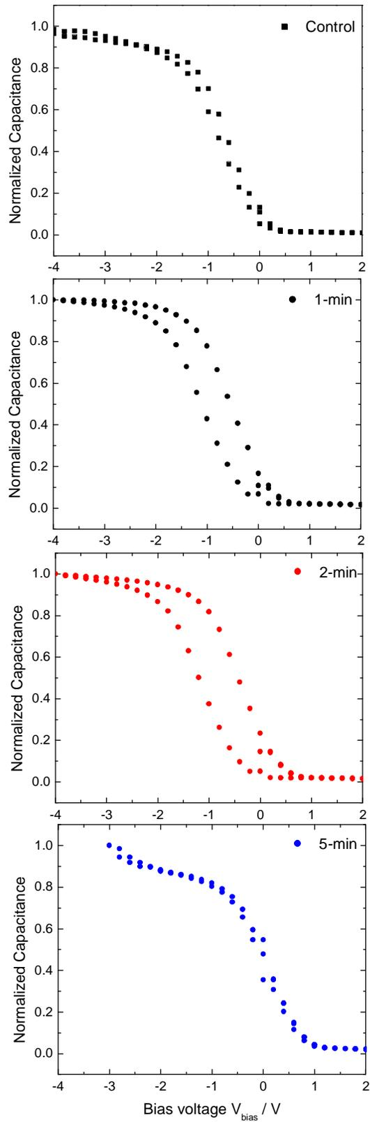
Figure 5.3.3 C-V measurement of the trilayer capacitor structure with different Ag nanocluster deposition time embedded in HfAlO matrix.
