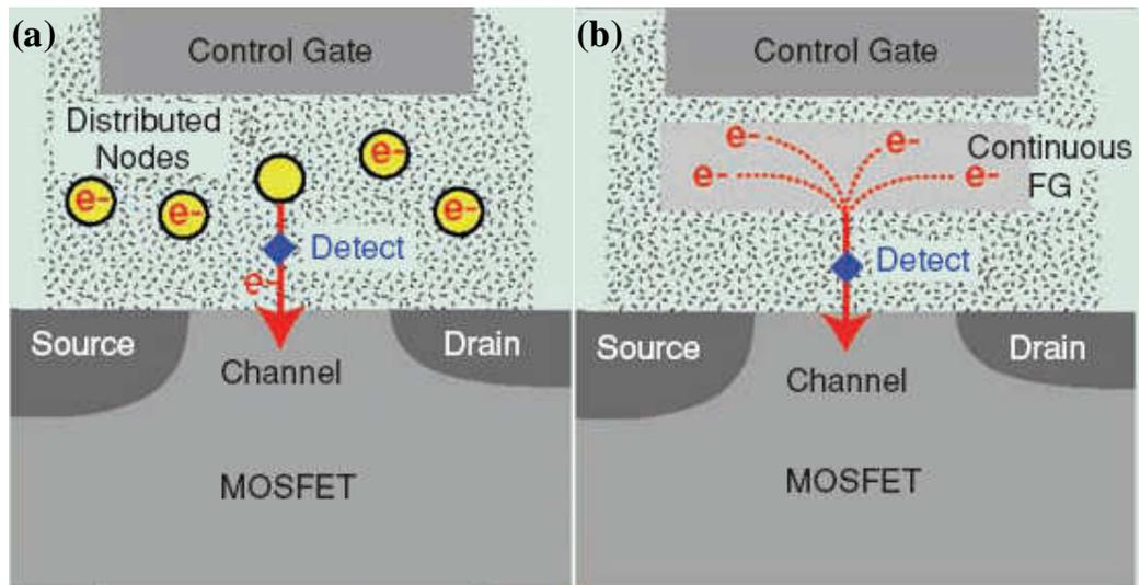
Figure 1.1.4 Charges stored in isolated storage nodes within the dielectric matrix (a), compared with a normal floating gate memory (b). [2]
