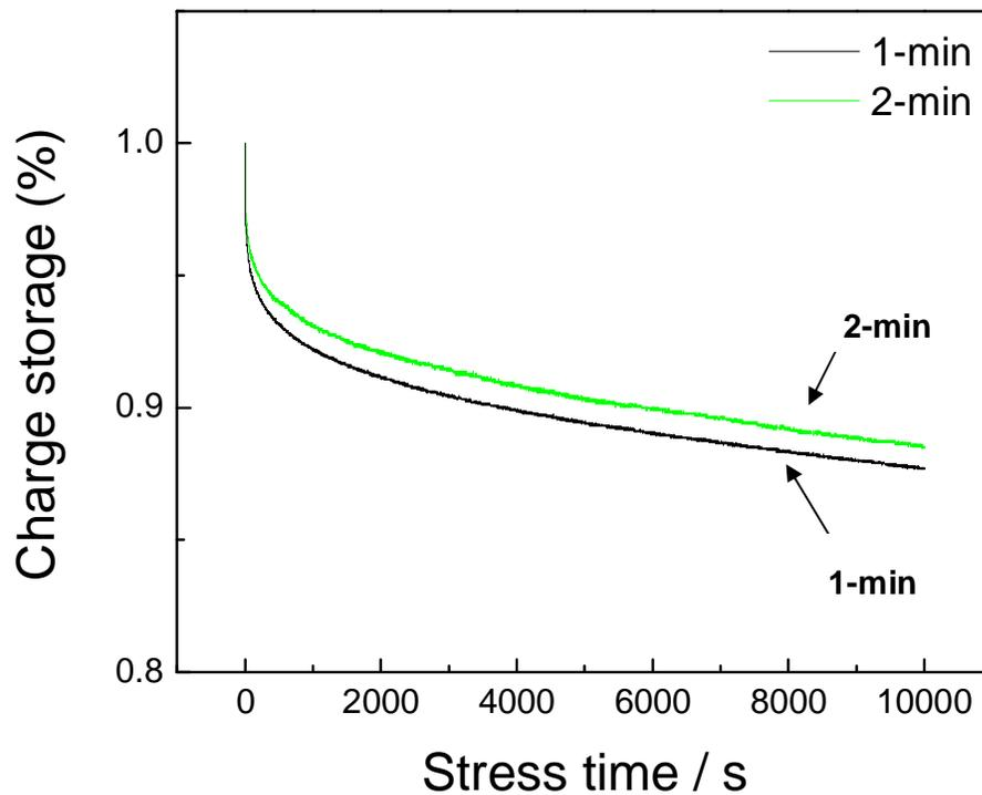
Figure 5.3.5  $C-t$  characteristics of the trilayer floating gate capacitors with 1- and 2-min Ag nanocluster deposition. The charging voltage is 10 V for 20 s and the measurement voltage is -1 V.
