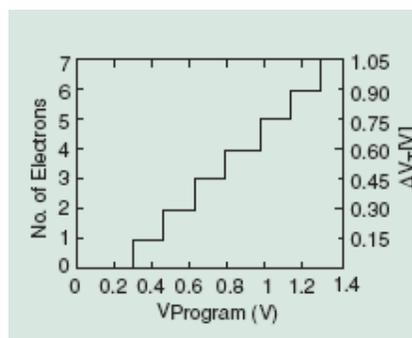
Figure 1.3.5 A simulated Coulomb staircase showing the change in the number of electrons in nanocrystals as a function of the program voltage (left axis). The corresponding threshold voltage memory shift is shown on the right axis. [2]
