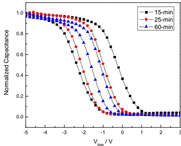
Figure 4.3.7 High frequency (1 MHz)  $C$ - $V$  characteristics of the trilayer floating gate capacitors with: (1)15-min, (2)25-min, and (3)60-min Ge nanocluster deposition. All samples are normalized with accumulation capacitance of 0.15 nF.
