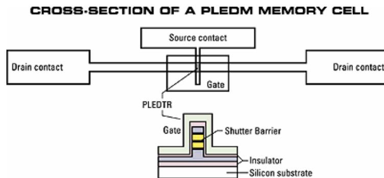
Figure 1.1.2 Cross-section of a PLEDM memory cell.[12-13]
