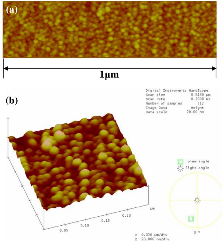
Figure 5.3.1 AFM images of the as-grown Ag nanocrystal on HfAlO; (a) surface image, and (b) 3-D view. From the AFM morphology images, the clear boundary indicates that the Ag nanocrystals are isolated from each other.
