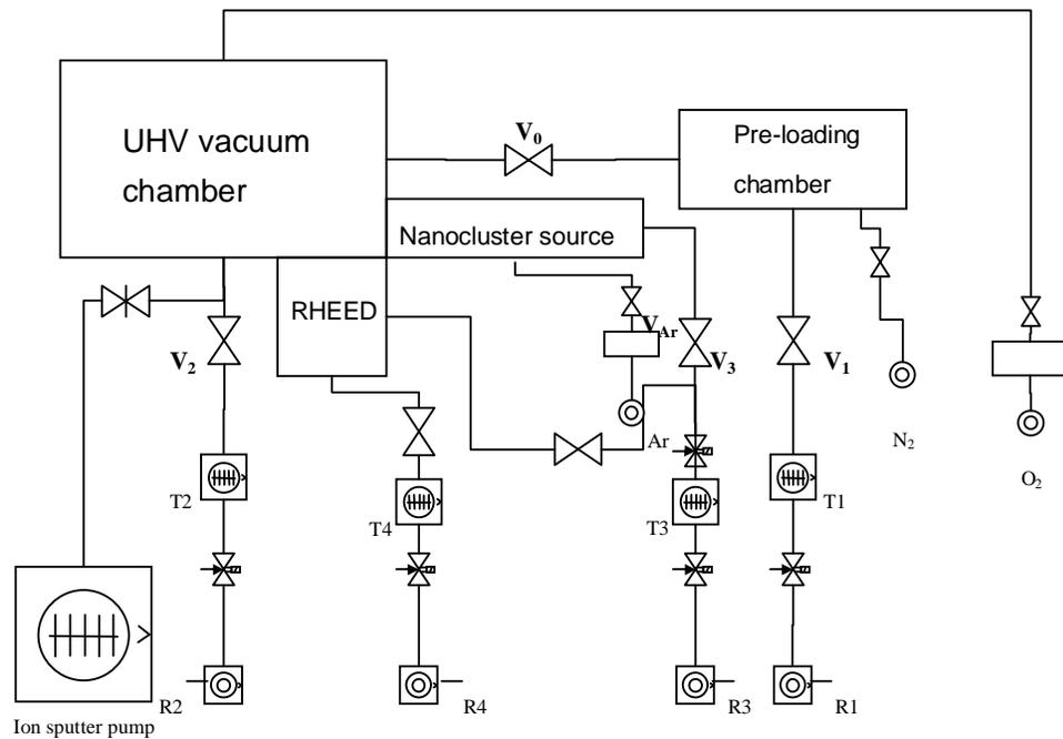
Figure 4.2.2 Vacuum system and gas circuit chart.
