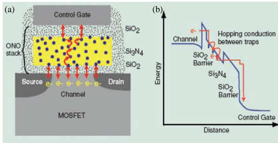
Figure 1.1.1 (a) Basic SONOS memory device structure. Arrows show paths of electron transport during memory operation. The electrons hop between trap sites (blue dots) within the Si<sub>3</sub>N<sub>4</sub> layer. Fig. 1.1.1(b) Energy diagram illustrating the physical process of a typical SONOS program operation. [2]
