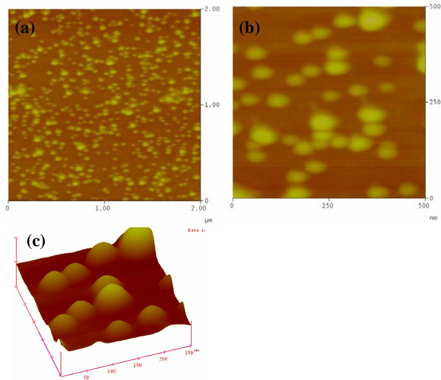
Figure 4.3.4 (a) AFM images of the Ge nanoclusters on HfAlO/Si substrate. (a) low magnification, (b) high-magnification, and (c) 3-D view.
