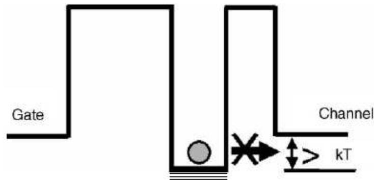
Figure 1.3.1 Energy barriers in the particular case of a metal nanocrystal with higher work function from silicon (channel area). [21]
