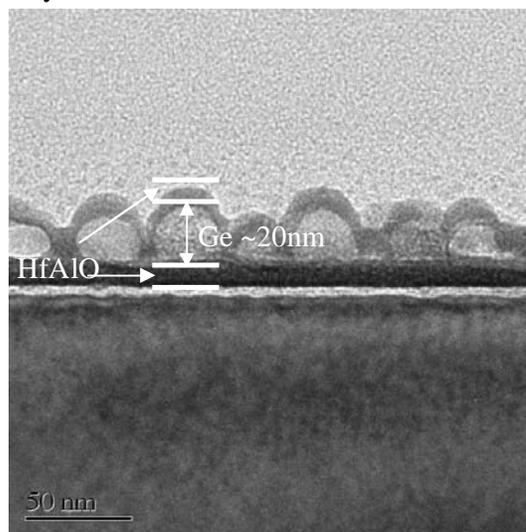
Figure 3.3.3 Cross-section TEM image of the as-grown sample.
