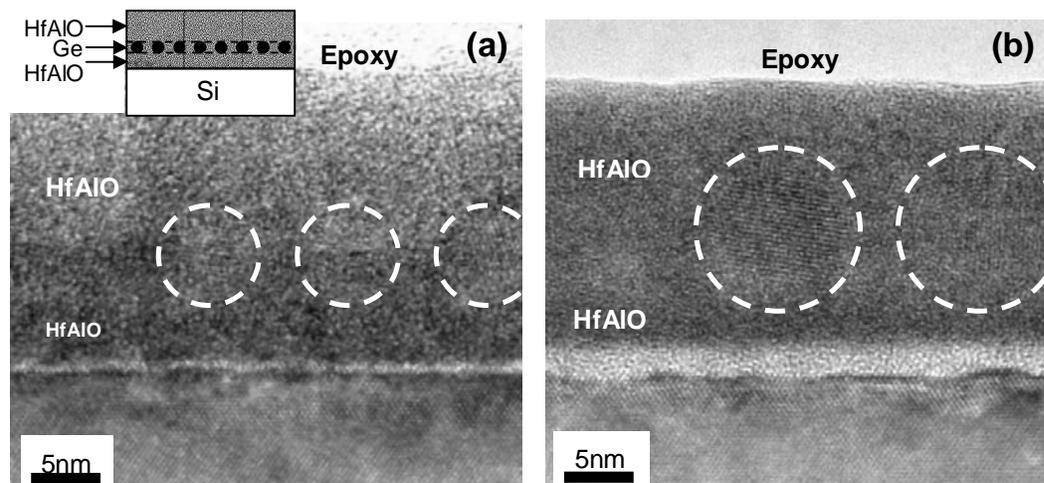
Figure 3.4.1 HRTEM images of the trilayer floating gate capacitors: (a) 1-min, and (b) 2-min Ge deposition . The region circled with dotted-line represents the Ge nanocrystals. The inset is a schematic diagram representing the trilayer structure.
