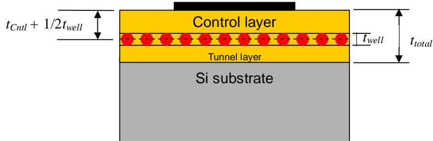
Figure 2.5.5 Schematic diagram of the trilayer nano-floating gate memory MOS capacitor.
