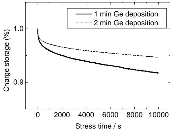
Figure 3.4.5  $C-t$  characteristics of the trilayer floating gate capacitor after 800 °C annealing in  $N_2$  ambient. The charging voltage is 10 V for 20 s and the measurement voltage of -1 V.
