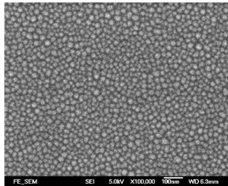
Figure 3.3.1 SEM picture of high density self-organized Ge nanocrystals deposited on HfAlO/Si substrate matrix by PLD for 1min at 600 °C.
