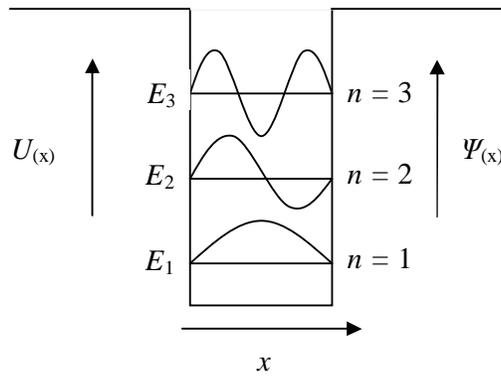
Figure 1.3.3 Potential well and wave functions of electrons confined in it.[185]
