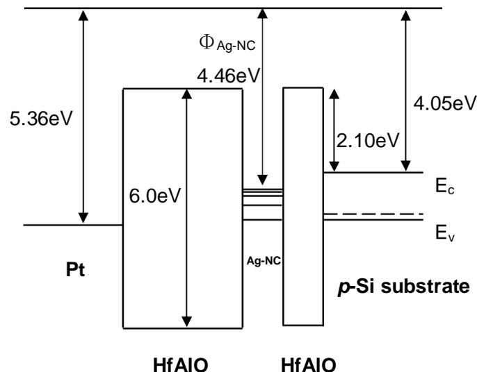
Figure 1.3.2 Energy band diagram of Ag trilayer nano-floating gate structure at flat band condition.
