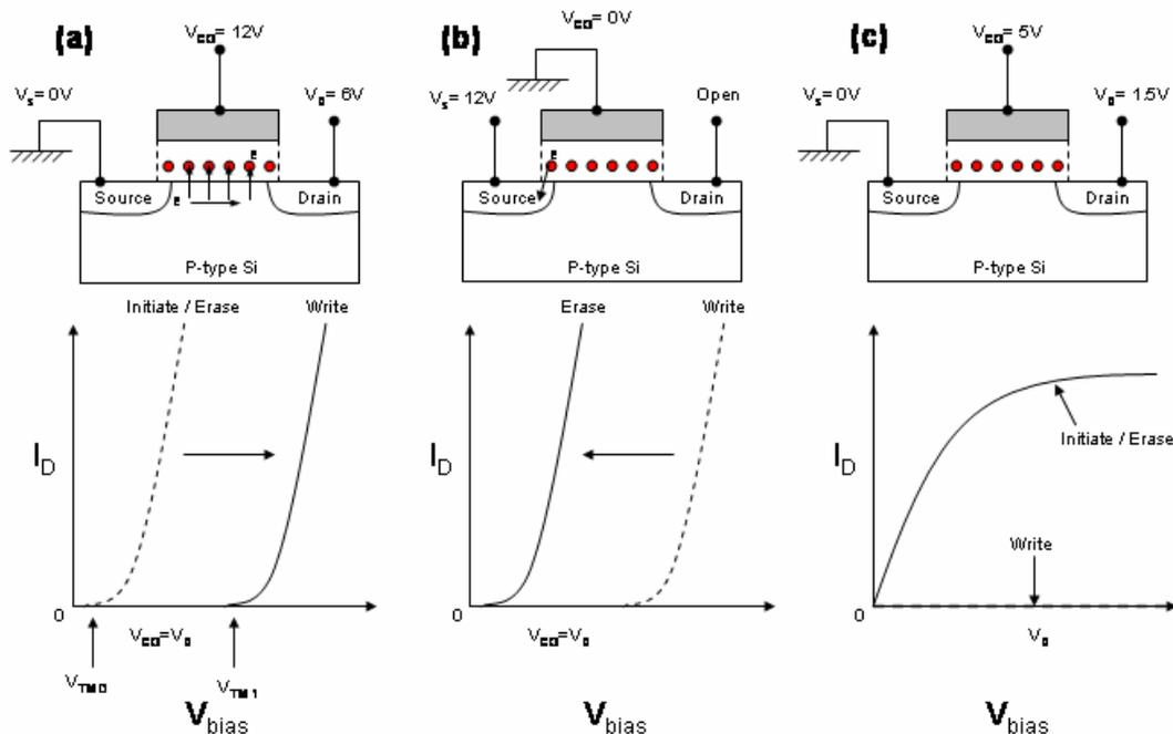
Figure 2.5.4 Schematic diagram describing the (a) write, (b) erase and (c) read processes of a nano-floating gate memory cell.
