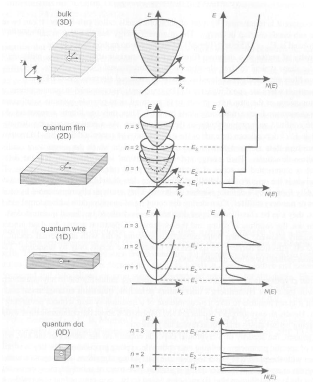
Figure 1.3.4 A schematic diagram of electron energy band structure and how the density of states changes as a function of dimensionality.[185]
