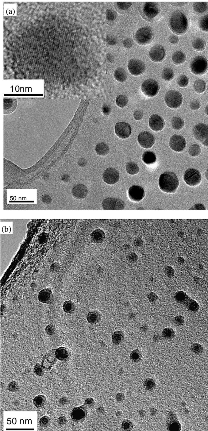
Figure 4.3.1 TEM images of Ge nanocrystals grown at 600 °C with a sputtering power of (a) 100 W and (b) 40 W. Aggregation distance is fixed at 100 mm and Ar gas flow rate at 40 sccm. Top-left inset is an image of Ge nanocrystal with a diameter of 20 nm. It shows that the as-grown Ge nanocrystals are crystalline under this condition. Bottom-left inset represents the HfAlO/Ge-NC/HfAlO/Si trilayer structure embedded with Ge-NC formed at 100 W sputtering power.
