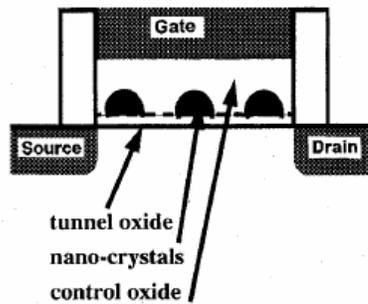
Figure 1.1.3 A schematic diagram of a nanocrystal floating gate memory cell.[14-15]
