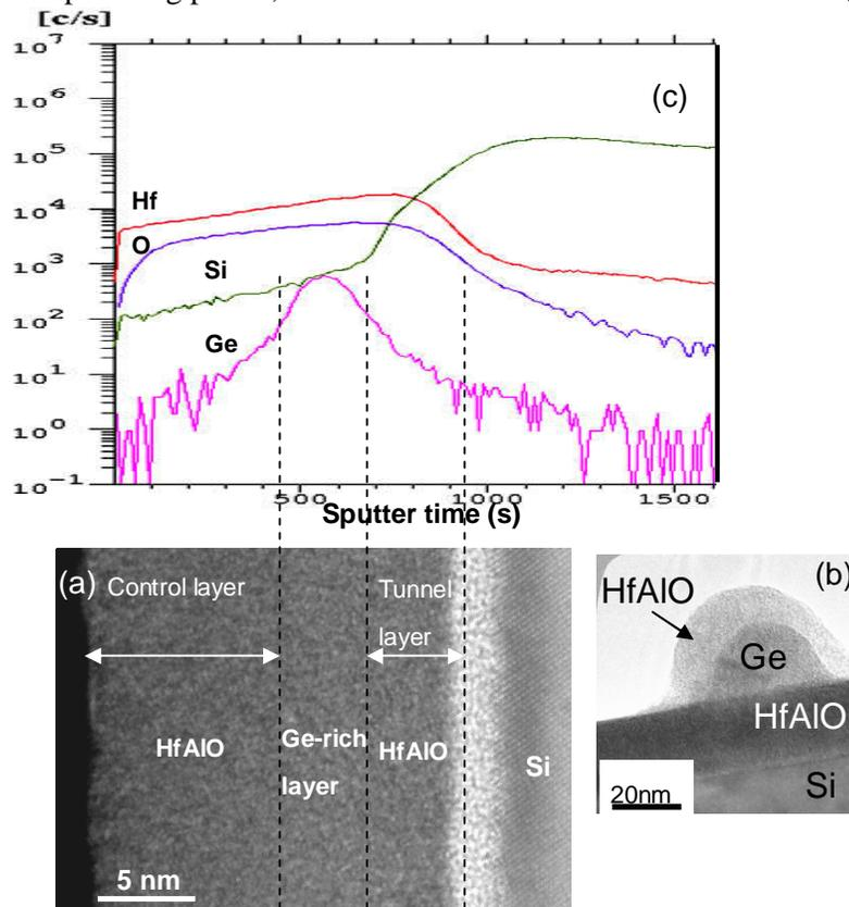
Figure 4.3.5 (a) A cross-sectional HRTEM image of the memory capacitor structure from the 15-min Ge nanocluster deposition sample, and (b) 30-min at 120W. (c) The depth profile SIMS result of the same sample in (a) showing content of Ge-rich layer inside the HfAlO oxide layer.
