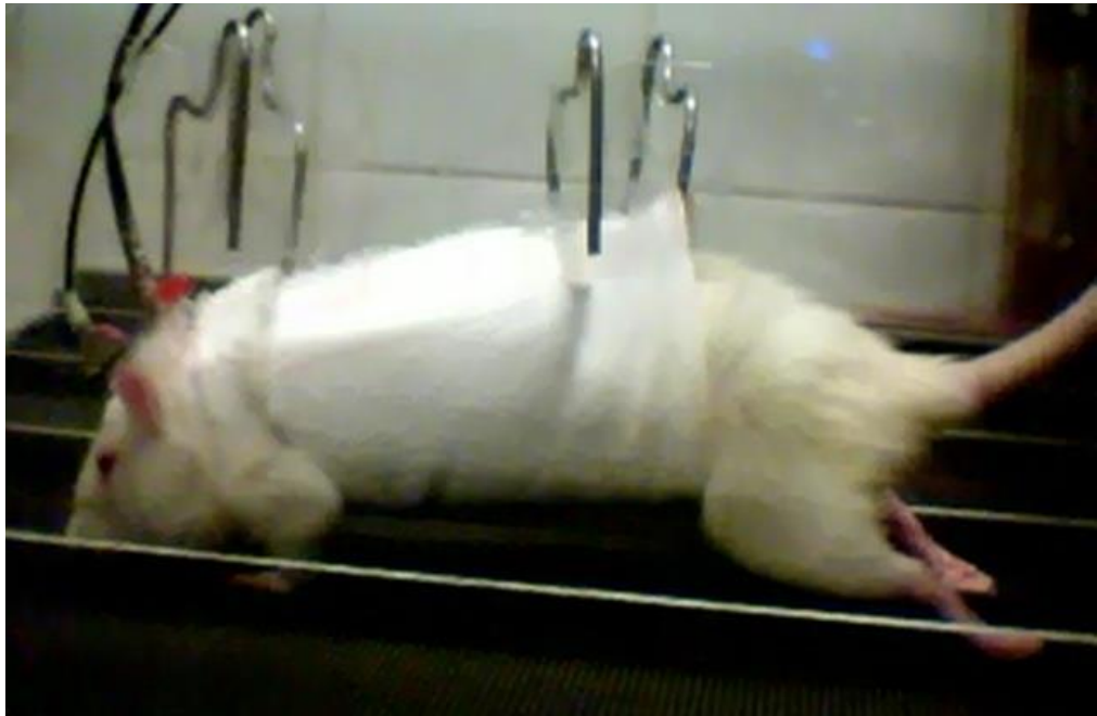
Figure 3.1 A spinal rat on a treadmill with custom body-weight support system.
