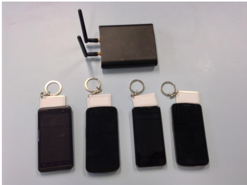
Fig. 26 RFID reader, RFID tags and Android phones used in the prototype
