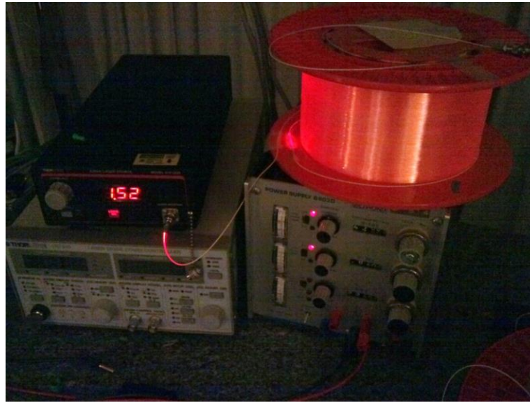
Figure 2-3 Rayleigh scattering in optical fiber (The picture is taken in our lab)
