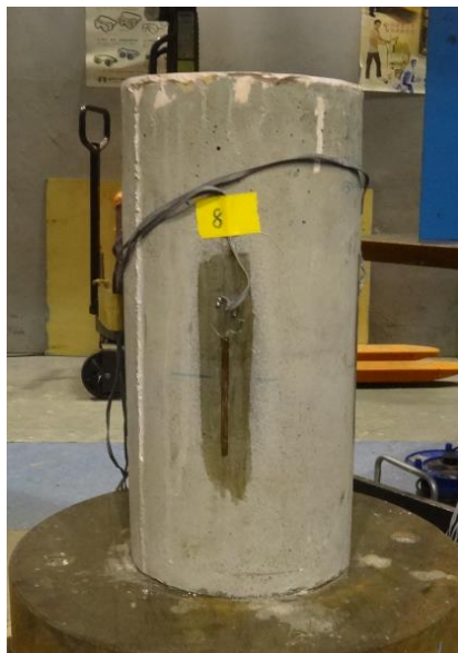
(a) Circular unconfined specimen
