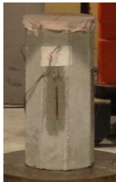
(b) Octagonal unconfined specimen
