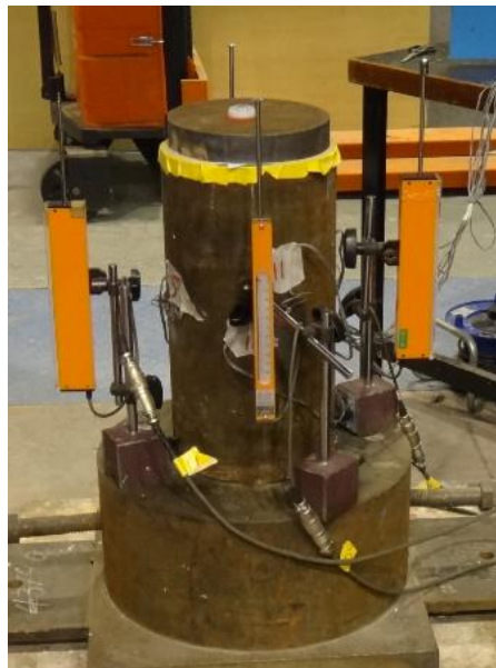
(a) Circular confined specimen
