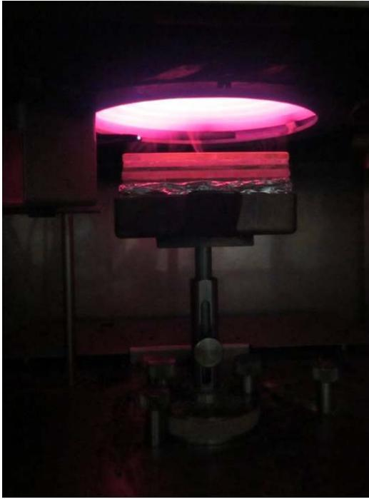
(a) Sample 5 under  $50 \text{ kW}\cdot\text{m}^{-2}$  heat flux
