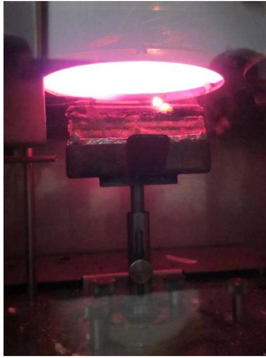
(b) Sample 5 under  $70 \text{ kW}\cdot\text{m}^{-2}$  heat flux
