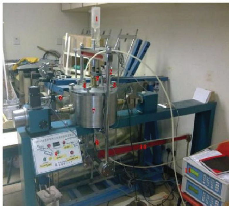
Figure 3.2 A photograph of the modified direct shear apparatus used in the present study
