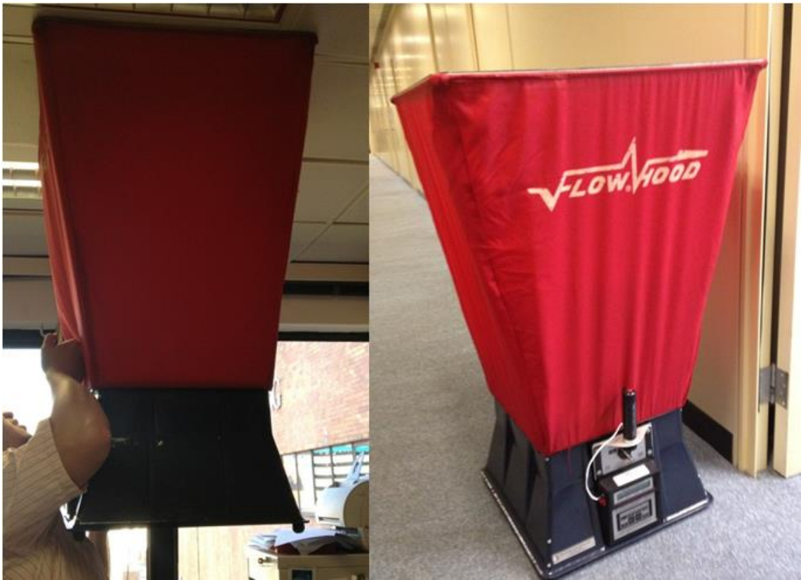
Figure 3. 3 Measurement of air flow rate
