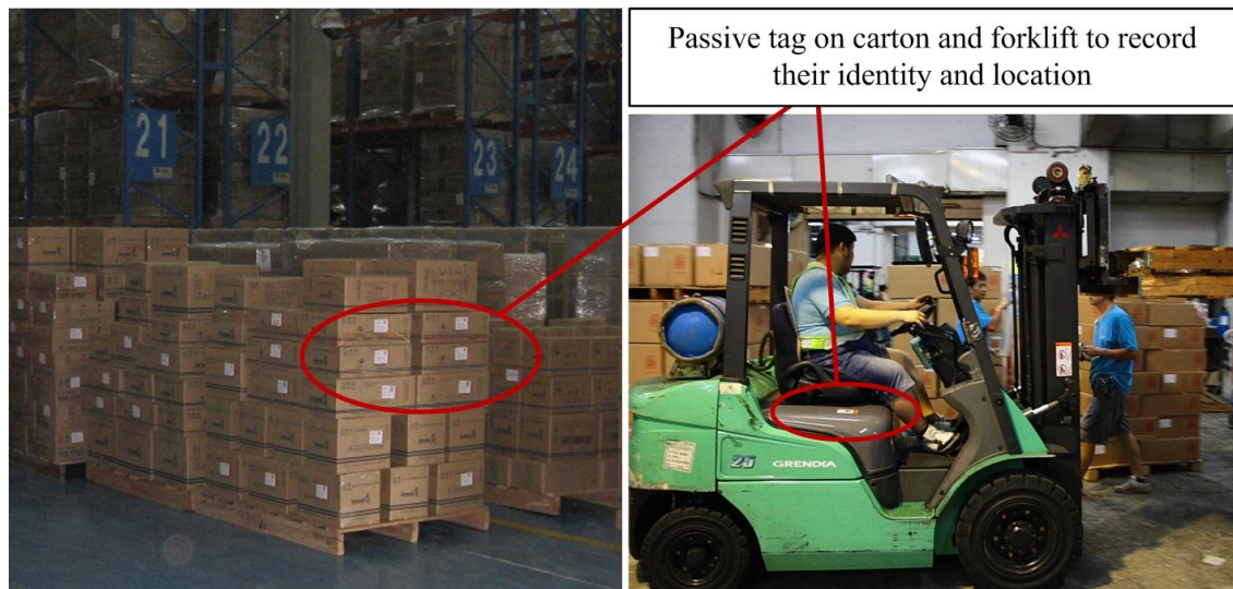
Figure 5.5 Passive RFID tag on carton and forklift
