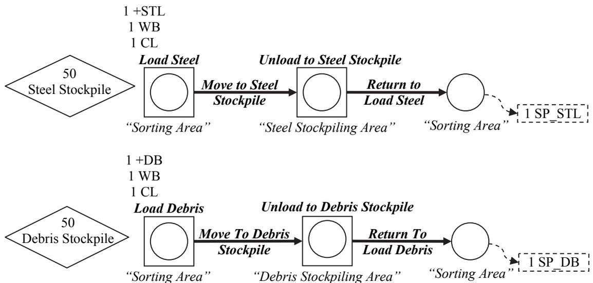
Figure 3.21. Process Mapping Model – Transportation of Steel and Debris Work Flow
