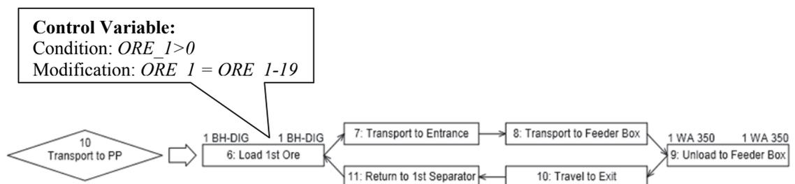
Figure 3.42. *SDESA* Model – Transport to Processing Plant Work Flow
