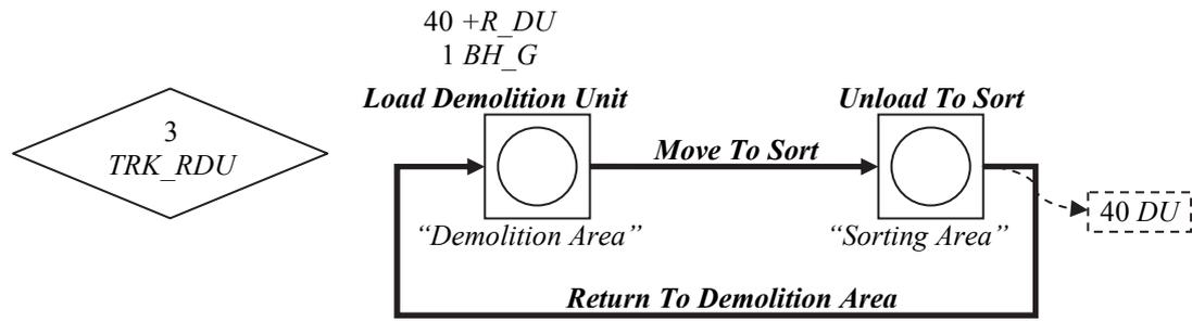
Figure 3.26. Process Mapping Model – Collection of *Raw Demolition Unit*
