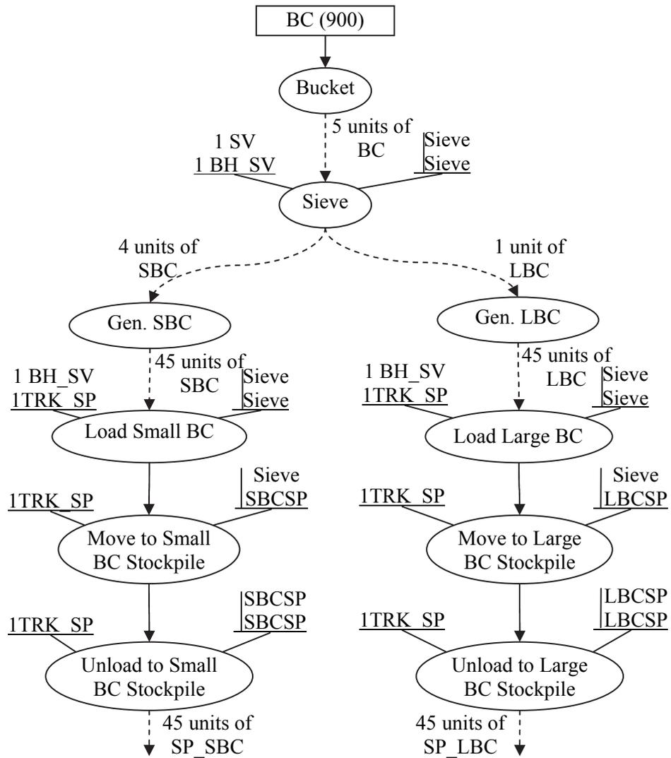
Figure 4.4. Waste-handling Process Flowchart for Sieving and Stockpiling Work Flow
