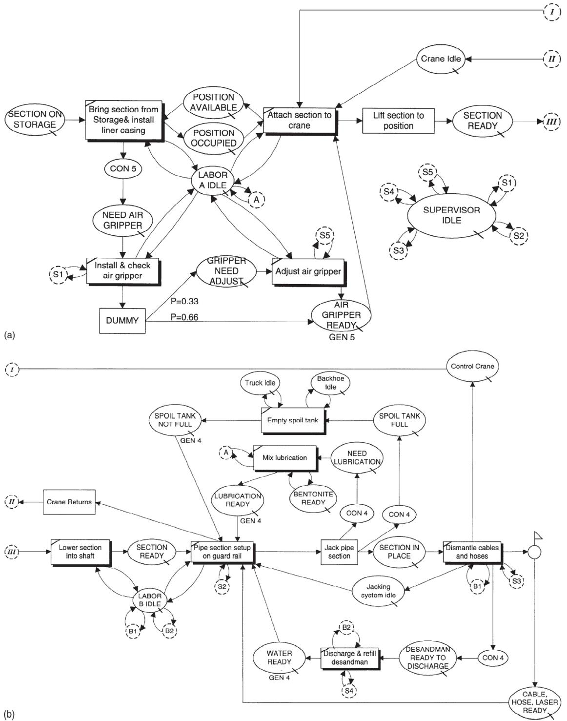
Figure 5.2. Prototype *CYCLONE* Model for the Observed Microtunneling Operation (Luo and Najafi 2007)
