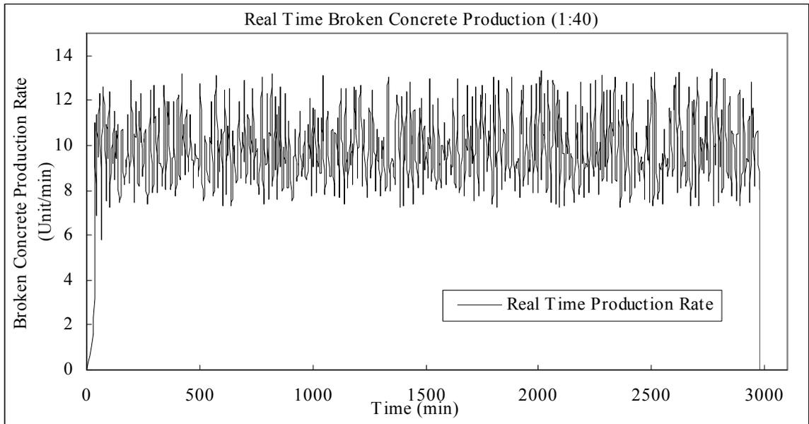
Figure 4.44. Real Time *BC* Production Rate against Time for Scale  $\frac{1}{40}$  x Model
