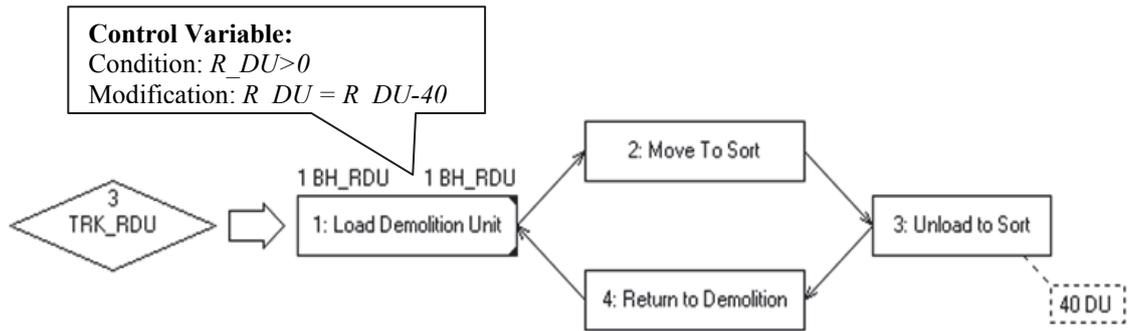
Figure 3.28. SDESA Model – Collection of Raw Demolition Unit Work Flow
