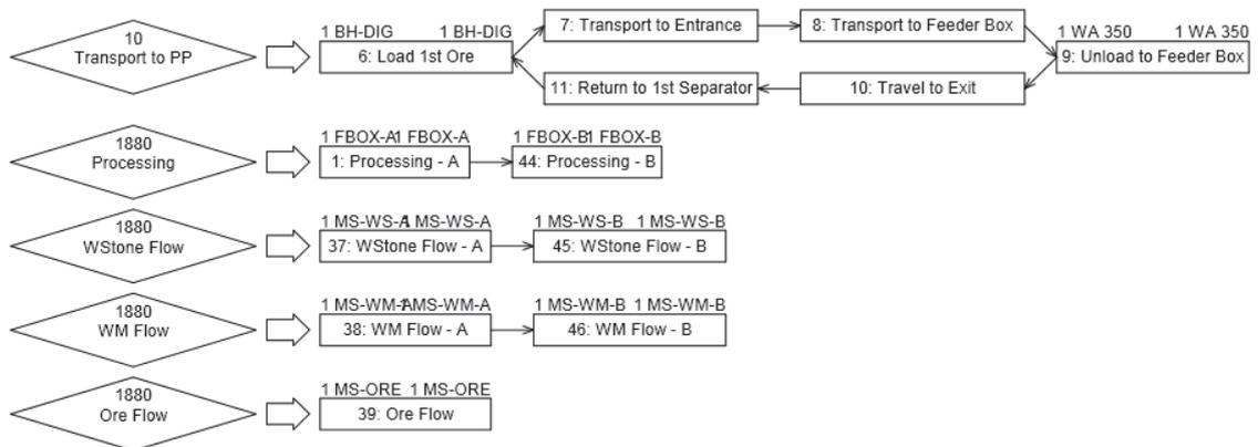
Figure 7.4. *SDESA* Model of Mining Process from Digging Area to Processing Plant
