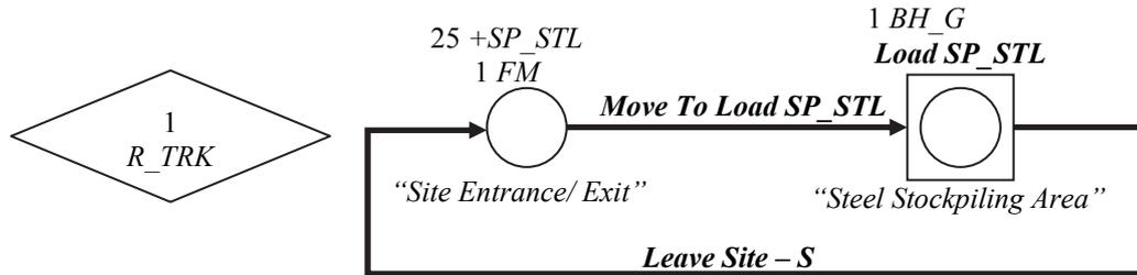
Figure 3.25. Process Mapping Model – Steel Recycling Work Flow
