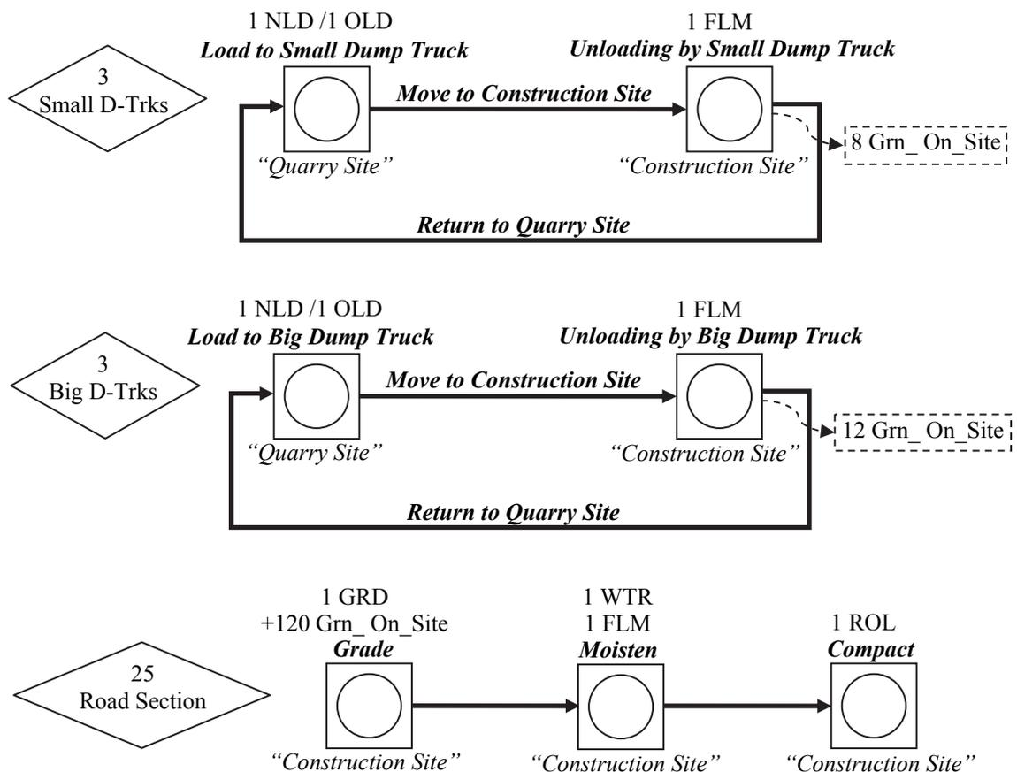
Figure 3.12. Process Mapping Model of a Road Base Construction Site
