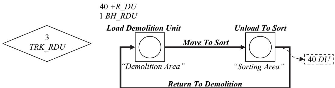
Figure 4.15. Process Mapping Model of Collection of Raw Demolition Unit Work Flow
