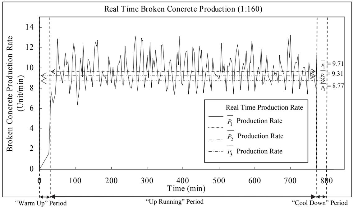
Figure 4.42. Real Time BC Production Rate against Time for Scale  $\frac{1}{160}$  x Model
