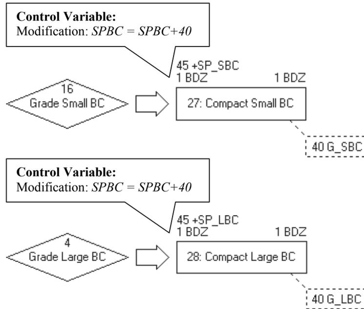
Figure 4.32. SDESA Model of Compaction Work Flow
