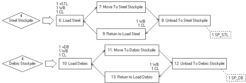
Figure 3.31. *SDESA* Model – *Transportation of Steel and Debris* Work Flow
