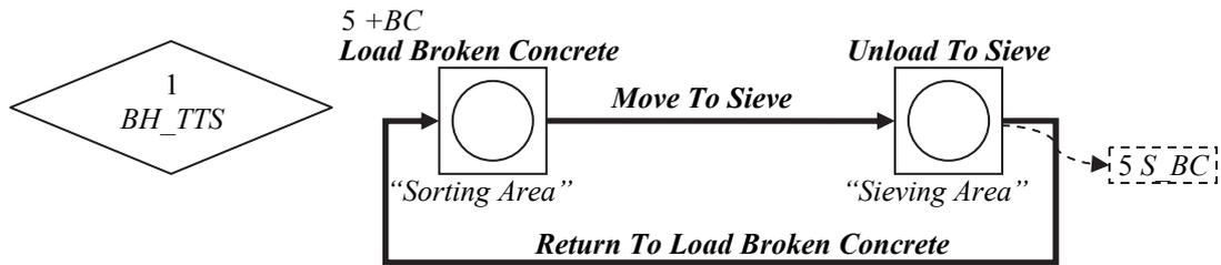
Figure 4.25. Mapping Model of Transportation of Broken Concrete Work Flow
