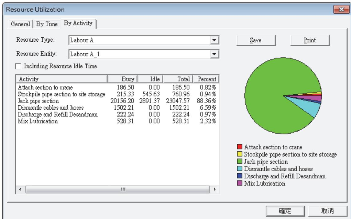
Figure 3.40. Statistical Output on Resource Utilization
