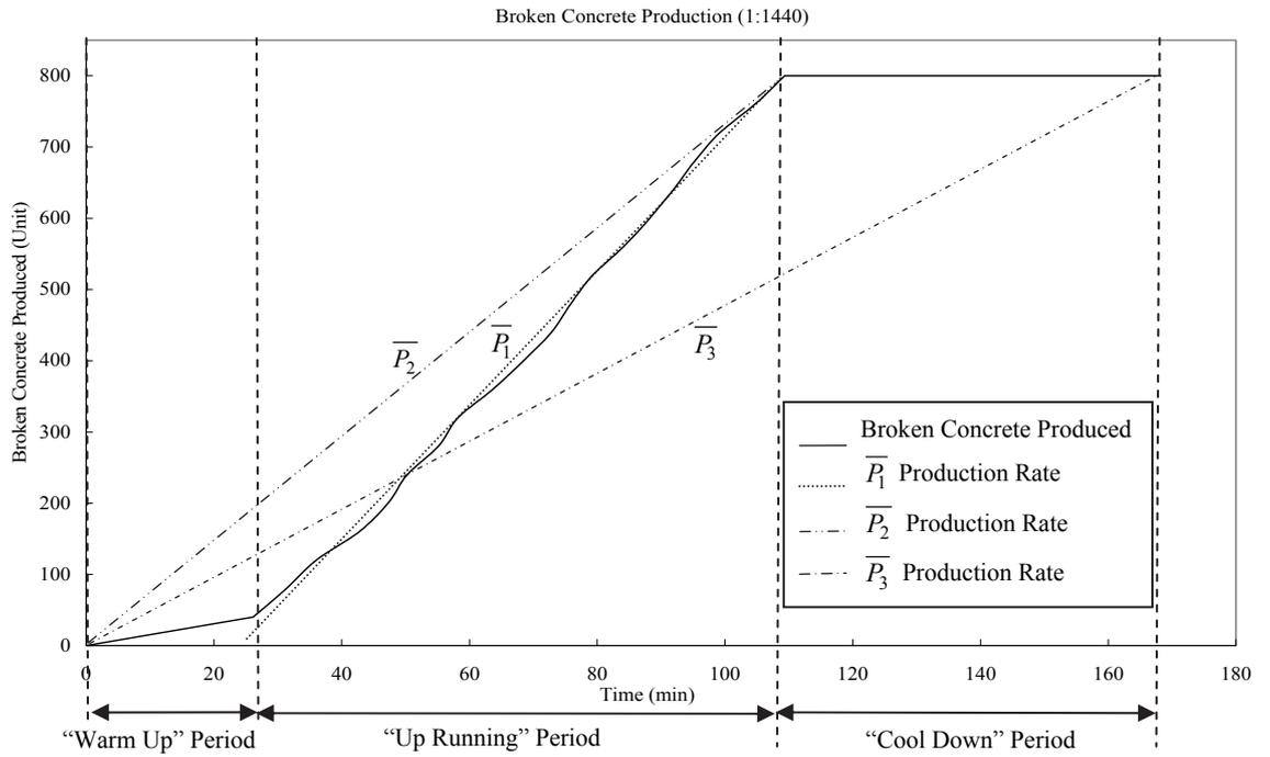
Figure 4.39. Broken Concrete Production against Time for Scale  $\frac{1}{1440}$  x Model
