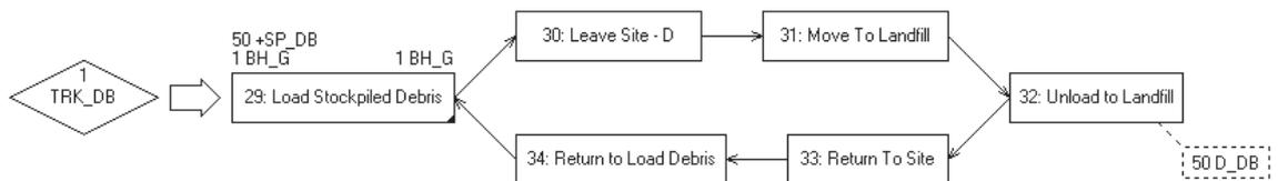
Figure 4.24. SDESA Model of Debris Disposal Work Flow
