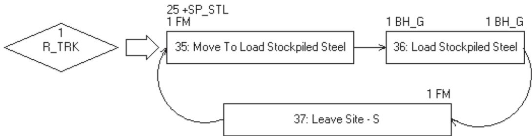
Figure 4.22. *SDESA* Model of Steel Recycling Work Flow
