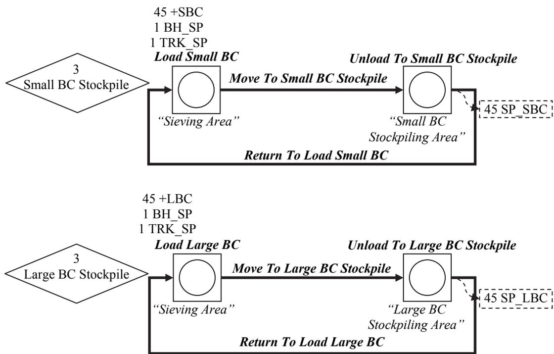
Figure 4.29. Mapping Model of Broken Concrete Stockpiling Work Flow
