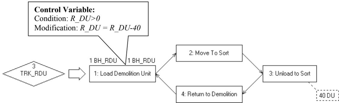
Figure 4.16. *SDESA* Model of Collection of Raw Demolition Unit Work Flow
