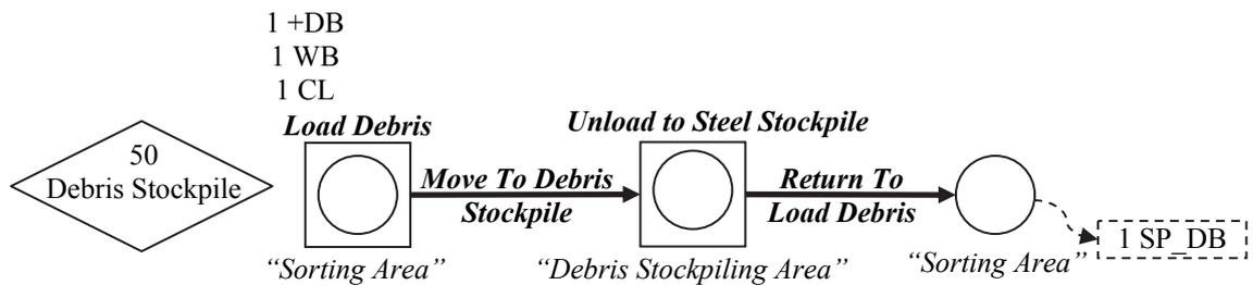
Figure 4.20. Process Mapping Model of *Debris Stockpile* Work Flow
