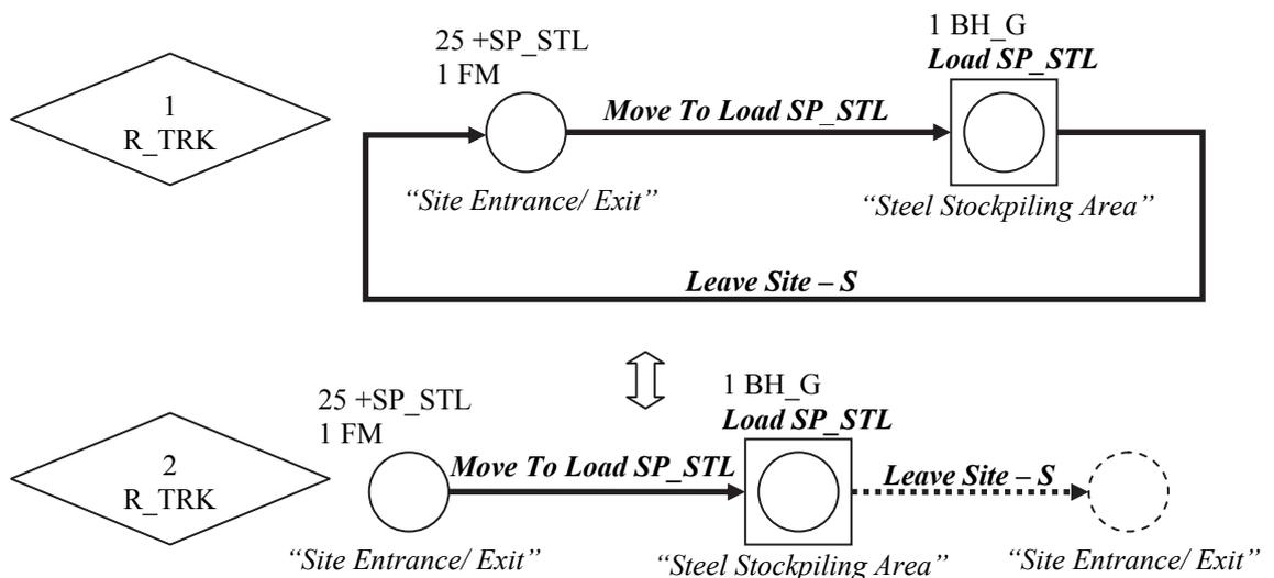
Figure 3.8. Conversion of a *VL* Type Work Flow into a *PL* Type Work Flow
