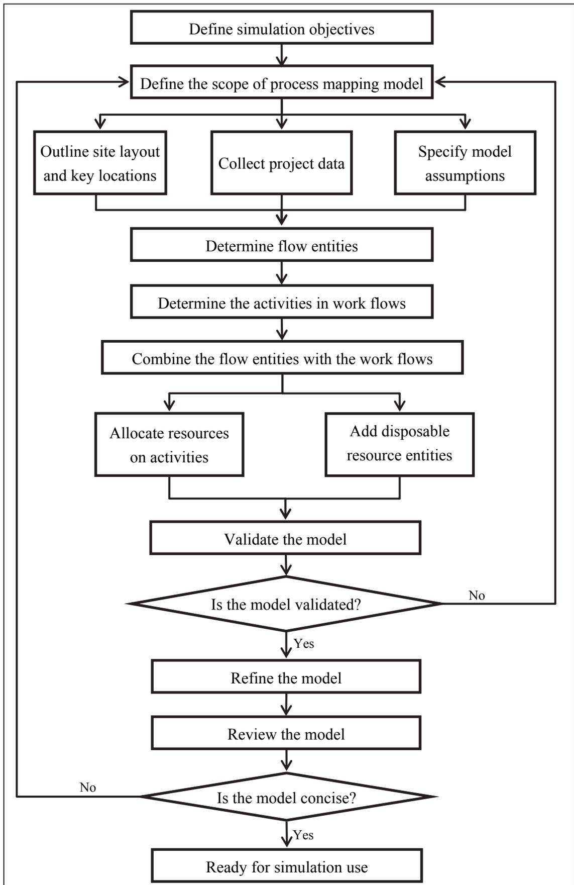
Figure 3.2. Formal Framework of the Construction Simulation Modeling Method
