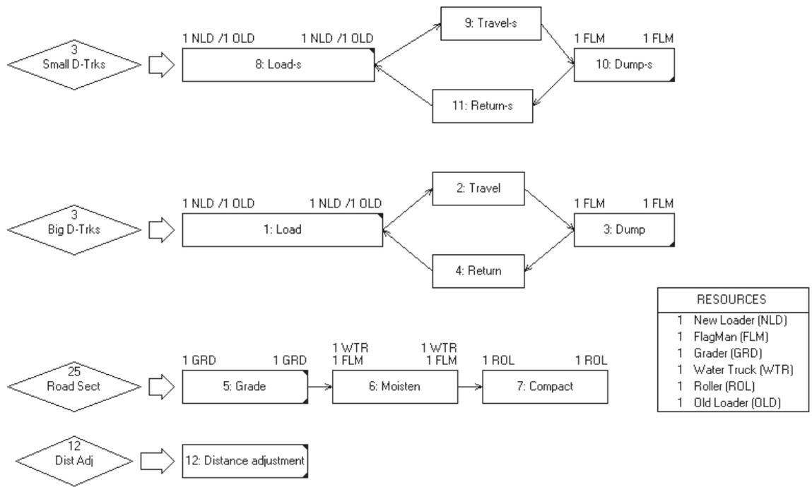
Figure 3.13. Refined Model of a Road Base Construction Site
