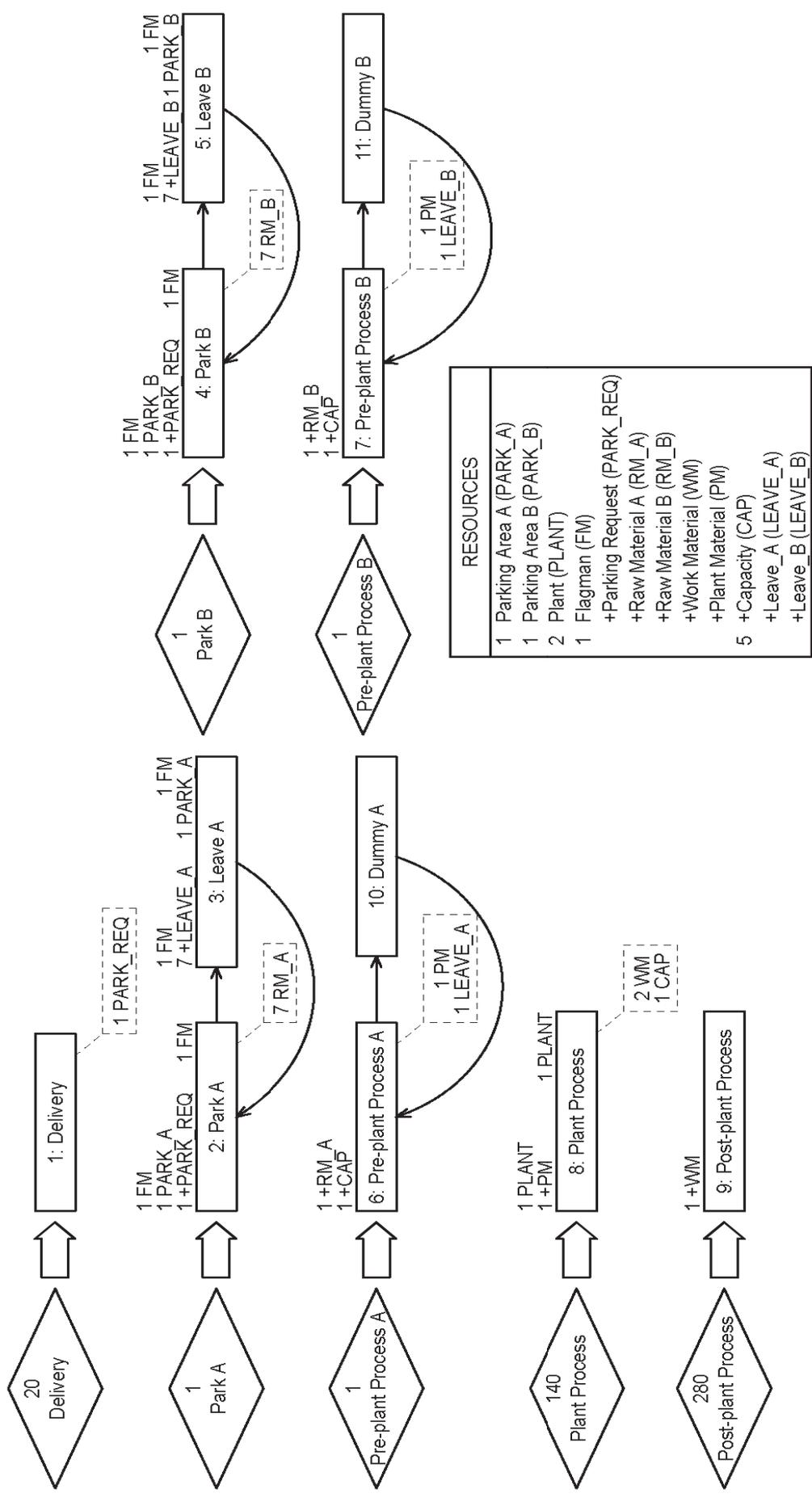
Figure 6.5. Total SDES4 Model of a Concreting Site
