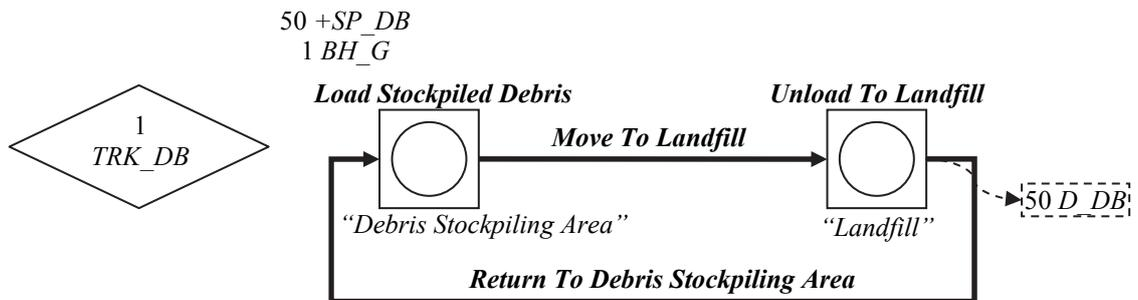
Figure 4.23. Process Mapping Model of Debris Disposal Work Flow
