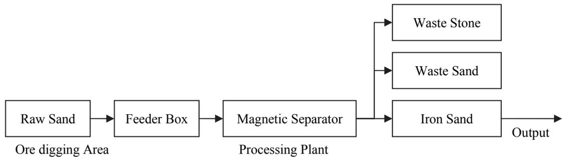
Figure 7.2. Schematic Flow of Iron Sand Processing
