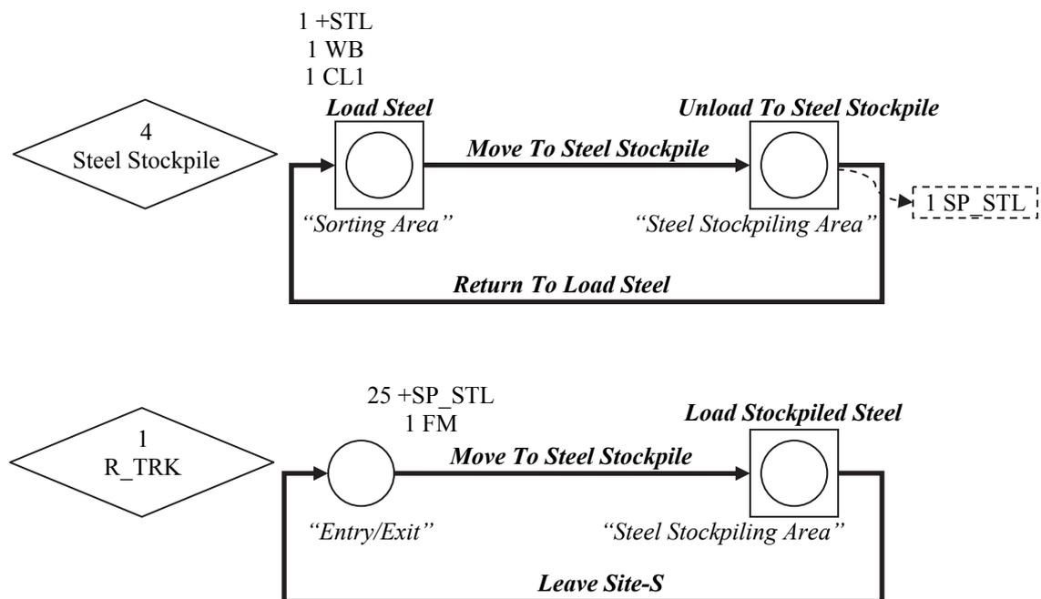
Figure 3.10. Process Mapping Model –Transportation of Steel and Steel Recycling Work Flow
