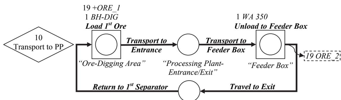
Figure 3.41. Process Mapping Model – *Transport to Processing Plant* Work Flow
