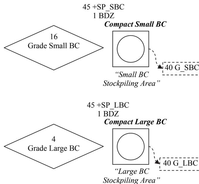
Figure 4.31. Mapping Model of Compaction Work Flow
