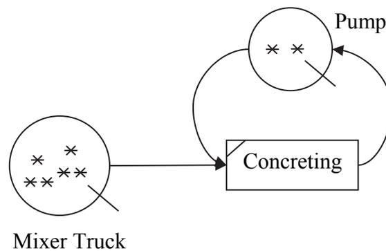
Figure 6.4. Updated *CYCLONE* Model with Two Resource Entities Being Placed Initially at the Queue Node Associated with the Stationary Pump
