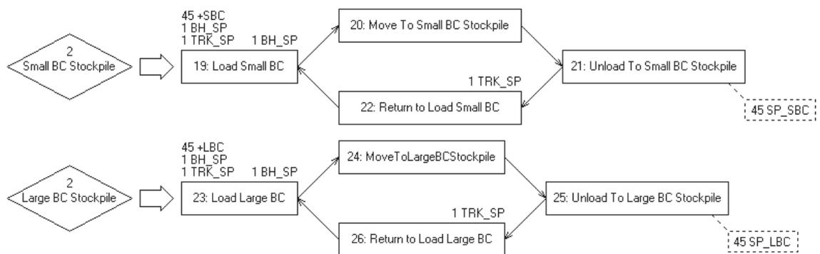
Figure 4.30. *SDESA* Model of Broken Concrete Stockpiling Work Flow
