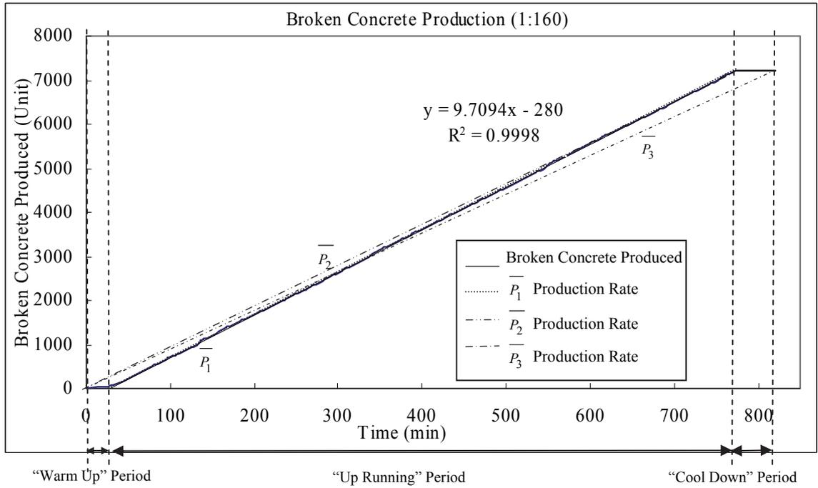
Figure 4.41. Broken Concrete Production against Time for Scale  $\frac{1}{160}$  x Model
