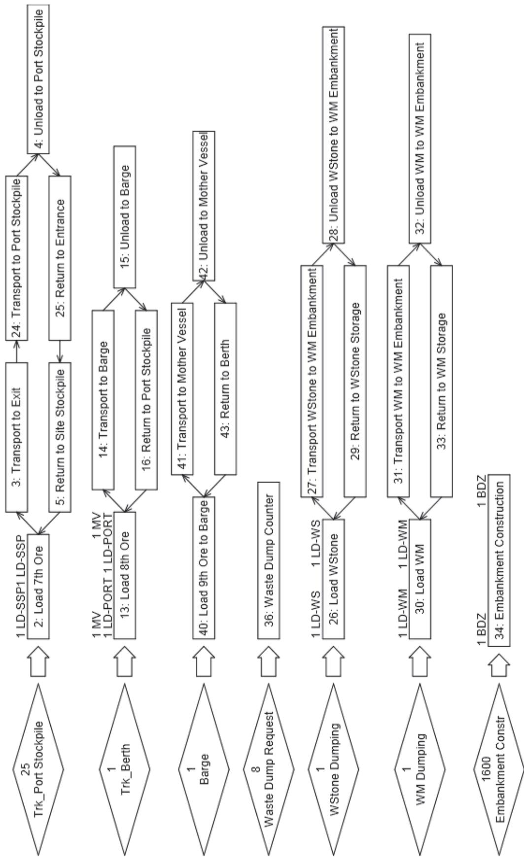
Figure 7.5. Total Model of Mining Project in Indonesia in SDESA (con't)
