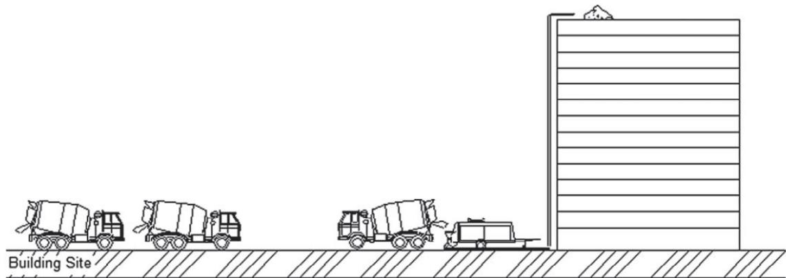
Figure 6.3. Illustration for Continuous Concrete Pumping Process
