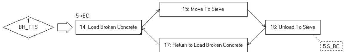
Figure 4.26. SDESA Model of Transportation of Broken Concrete Work Flow
