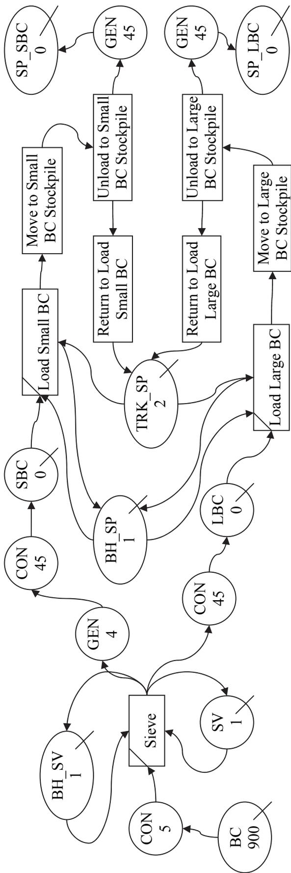
Figure 4.3. CYCLONE Model for Sieving and Stockpiling Work Flow
