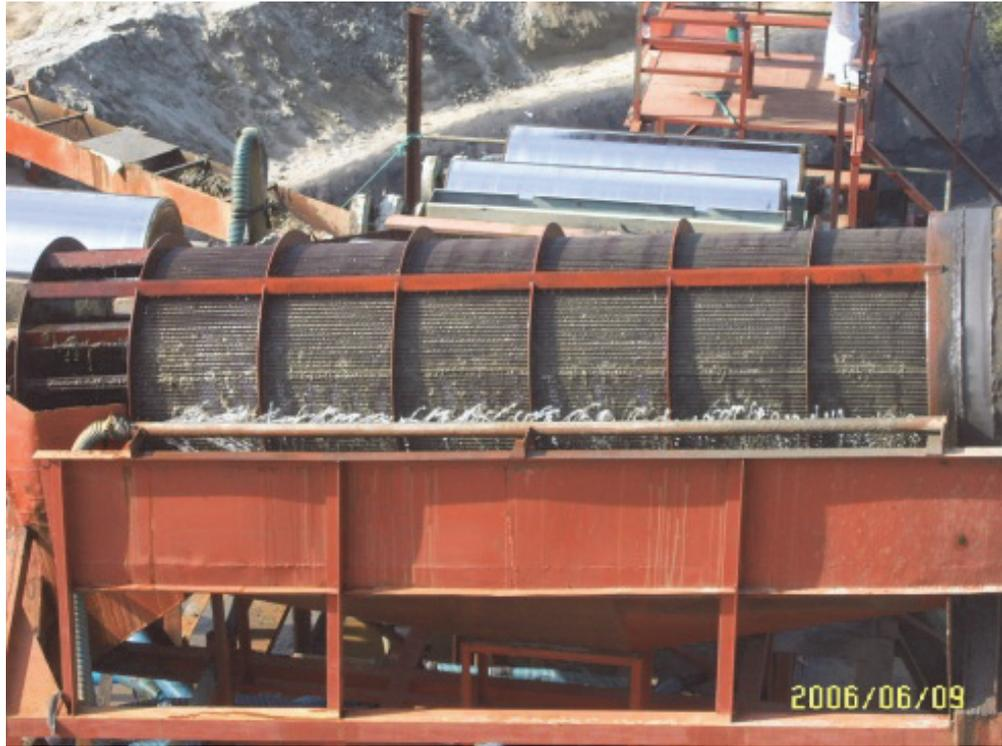
Figure 6.6. Raw Material Slurry Undergoing Magnetic Separation
