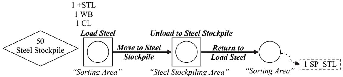
Figure 4.19. Process Mapping Model of *Steel Stockpile* Work Flow
