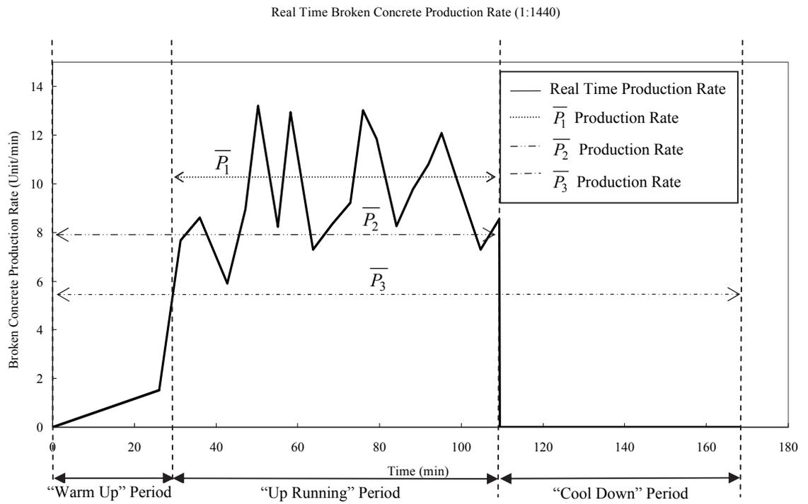
Figure 4.40. Real Time BC Production Rate against Time for Scale  $\frac{1}{1440}$  x Model
