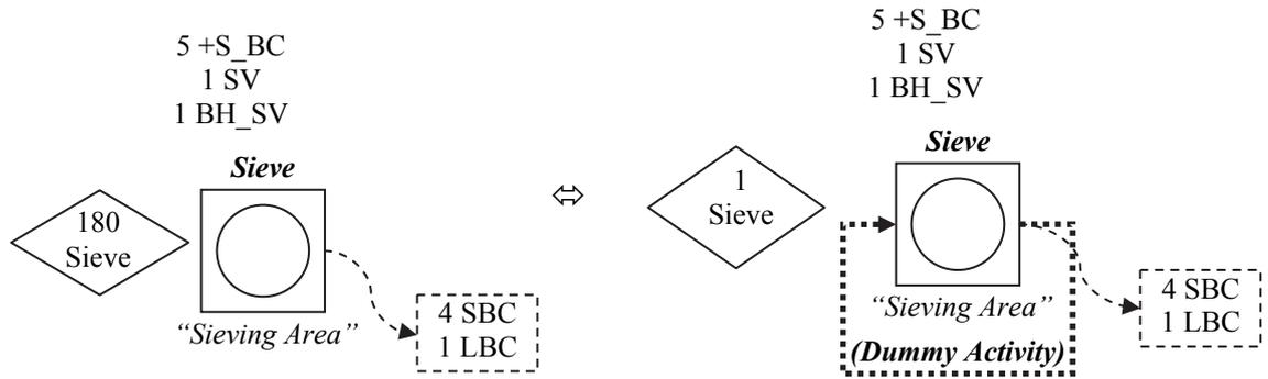
Figure 3.7. Conversion of a *PL* Type Work Flow into a *VL* Type Work Flow
