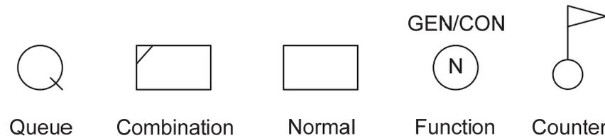
Figure 2.1. Basic Modeling Elements of *CYCLONE*
