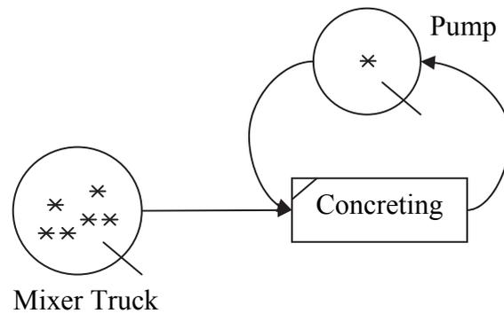
Figure 6.2. Simple *CYCLONE* Model for Concrete Pumping Process
