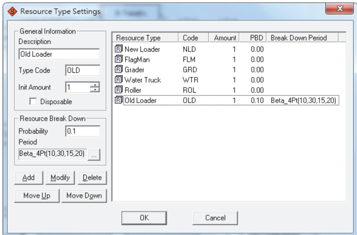
Figure 3.15. Resource Type Setting for “Old Loader” in a Road Base Construction Site
