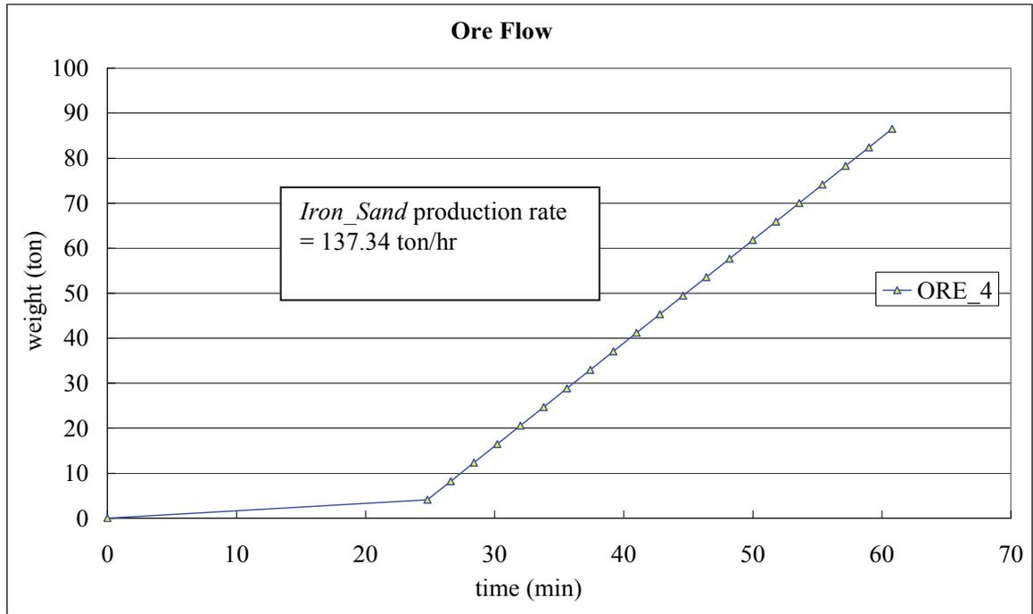
Figure 7.7. Iron Sand Production over Time Resulting from *SDESA* Simulation
