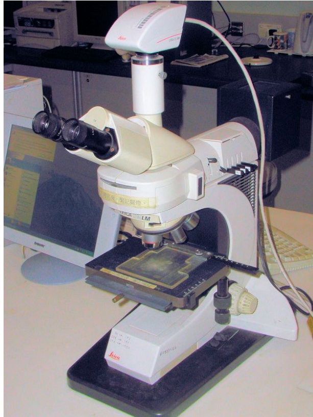
Fig 6.8 Microscope used in the FLDs test
