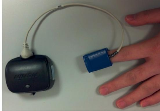
Fig. 5.3: Nonin Model 4100 Bluetooth pulse oximeter
