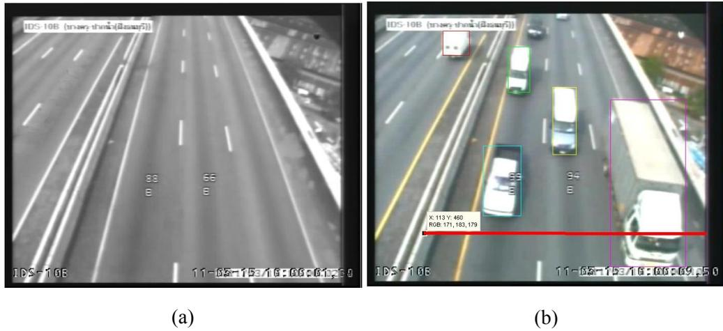
**Figure 3.1:** (a) Background estimation; (b) Effect of object detection
