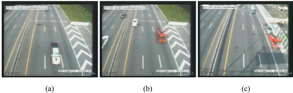
**Figure 5.7:** Real-world case study #1: (a) Incident vehicle passes the upstream detector; (b) Tow truck passes the upstream detector; (c) Incident vehicle and truck passes through the downstream detector
