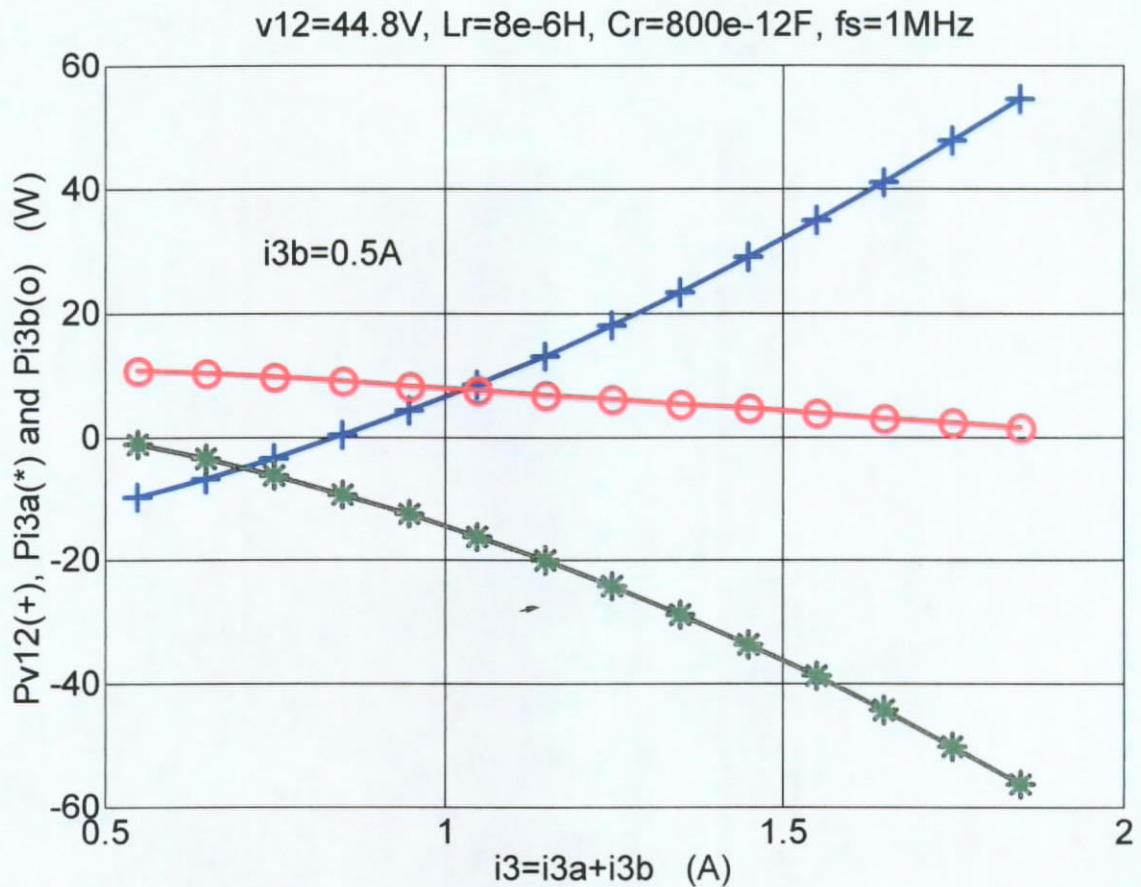
Fig. 3.4. Power Distribution of Half-wave Type of FM ZVS QR Cuk Converters.
