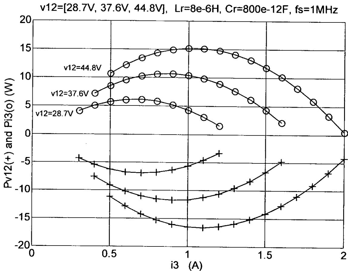
Fig. 7.1. Power Distribution of Half-wave Type of FM ZVS QR Buck Converter.
