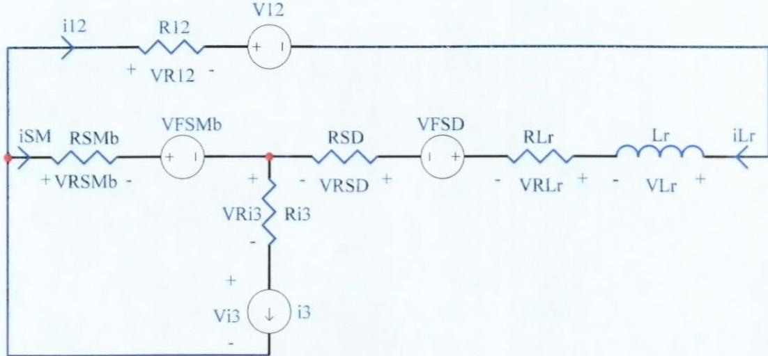
Fig. 5.4. Inductor Discharging Stage [ $T_a, T_3$ ] of FM ZVS QR Boost Converter.
