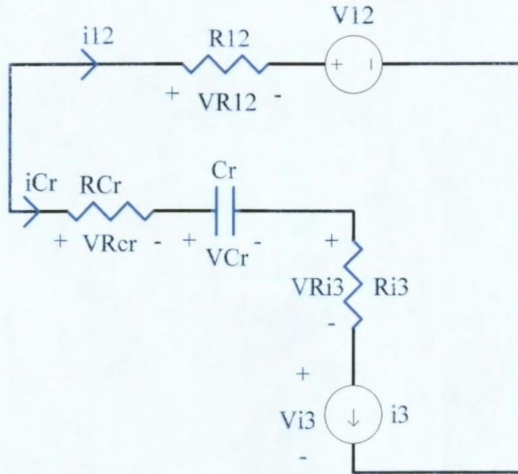
Fig. 4.2. Capacitor Charging Stage  $[T_0, T_1]$  of FM ZVS QR Buck Converter.
