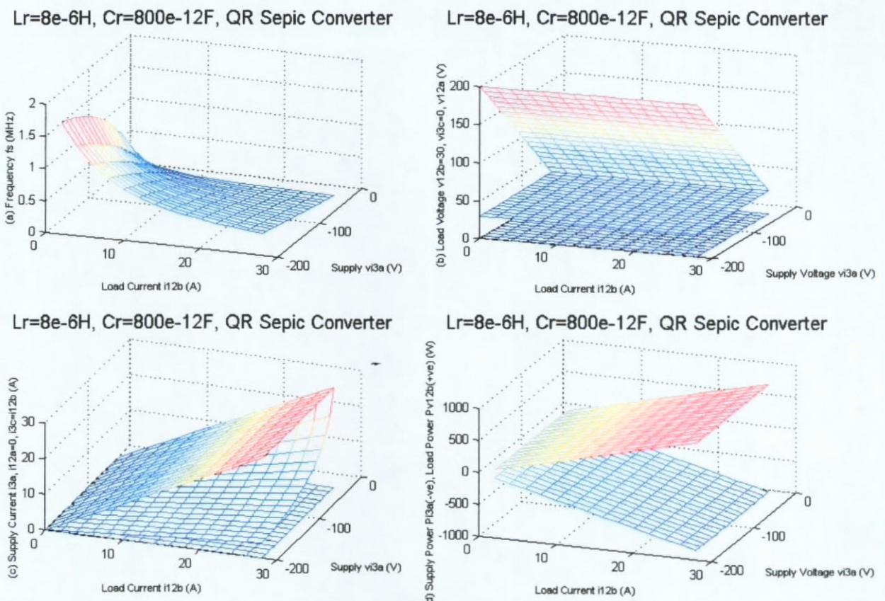
Fig. 7.11. QR Regulated Sepic Converter (a) Switching Frequency  $f_s$ , (b) Regulated Load Voltage  $V_{12b}$  & Intermediate Voltage Branch  $V_{12a}$ ,  $V_{i3c}$  (c) Supply Current  $I_{3a}$  & Intermediate Current Branch  $I_{12a}$ ,  $I_{3c}$  (d) Supply Power  $P_{i3a}$  and Load Power  $P_{v12b}$ .
