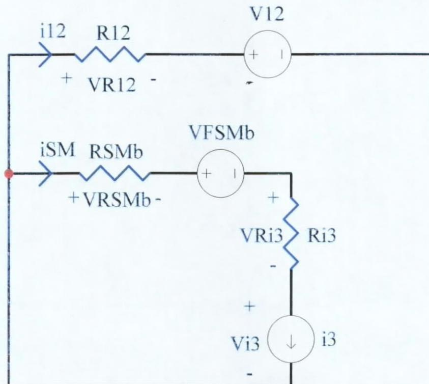
Fig. 5.5. Free-Wheeling Stage  $[T_3, T_s]$  of FM ZVS QR Boost Converter.
