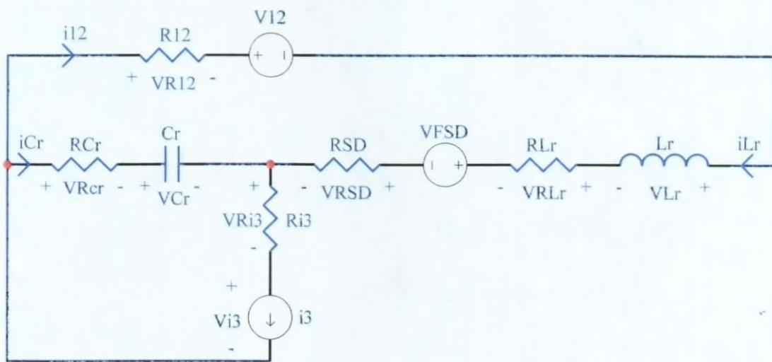
Fig. 5.2. Resonant Stage  $[T_1, T_2]$  of FM ZVS QR Boost Converter.
