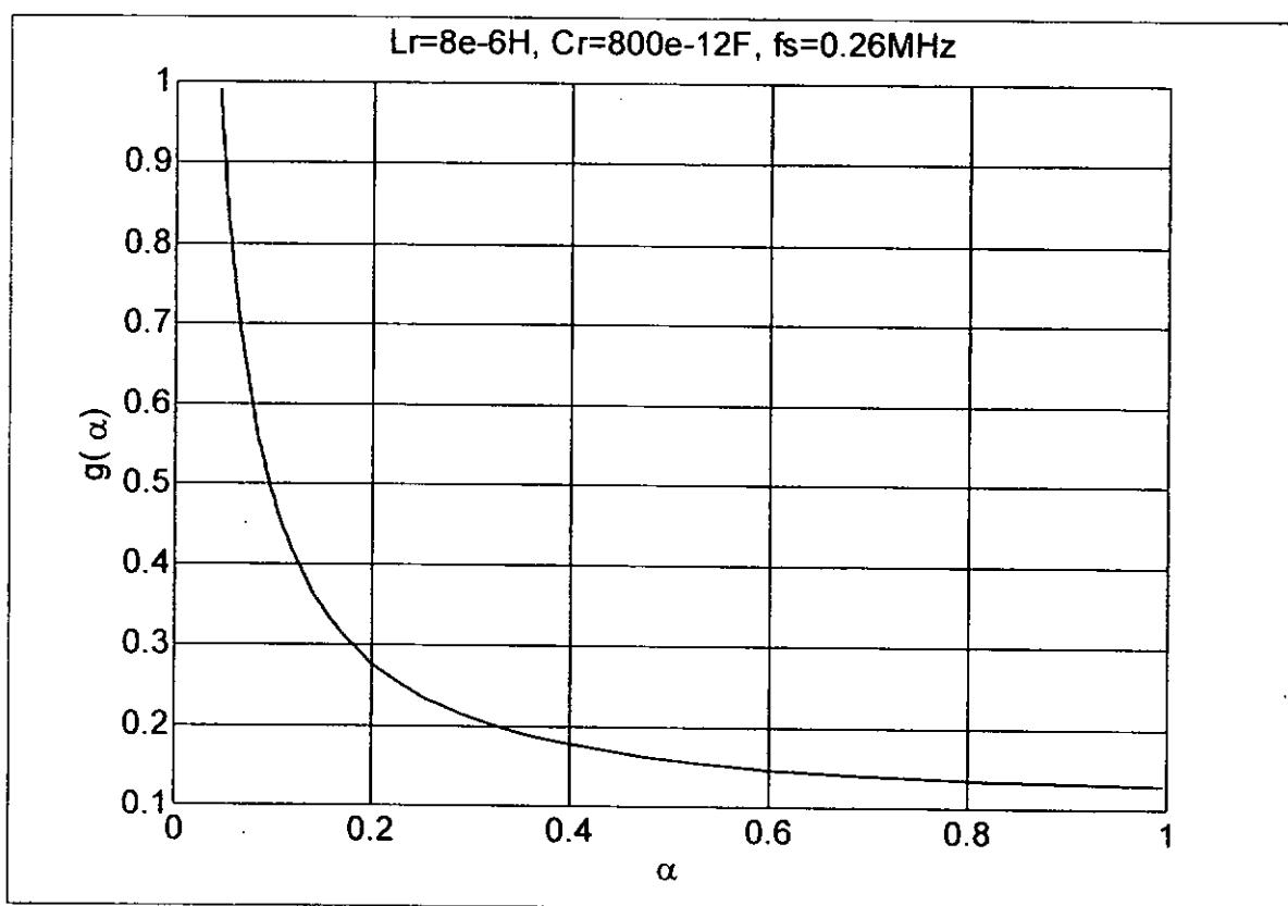
Fig. 2.7 Transfer Function  $g(\alpha)$  at a fixed switching frequency  $f_s = 260 \text{ kHz}$ .
