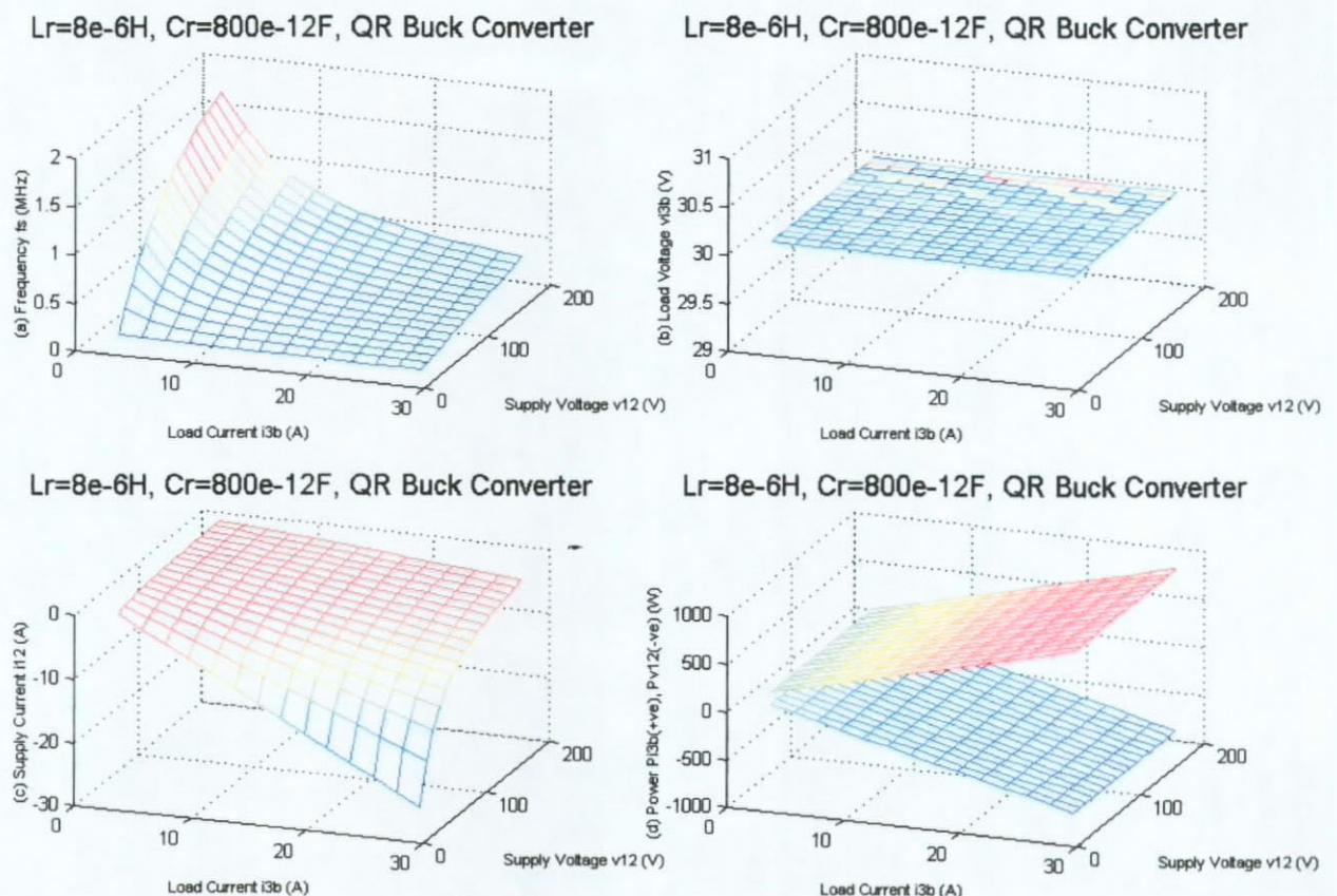
Fig. 7.7. QR Regulated Buck Converter (a) Switching Frequency  $f_s$ , (b) Regulated Load Voltage  $V_{i3}$ , (c) Supply Current  $I_{12}$ , (d) Supply Power  $P_{v12}$  and Load Power  $P_{i3}$ .
