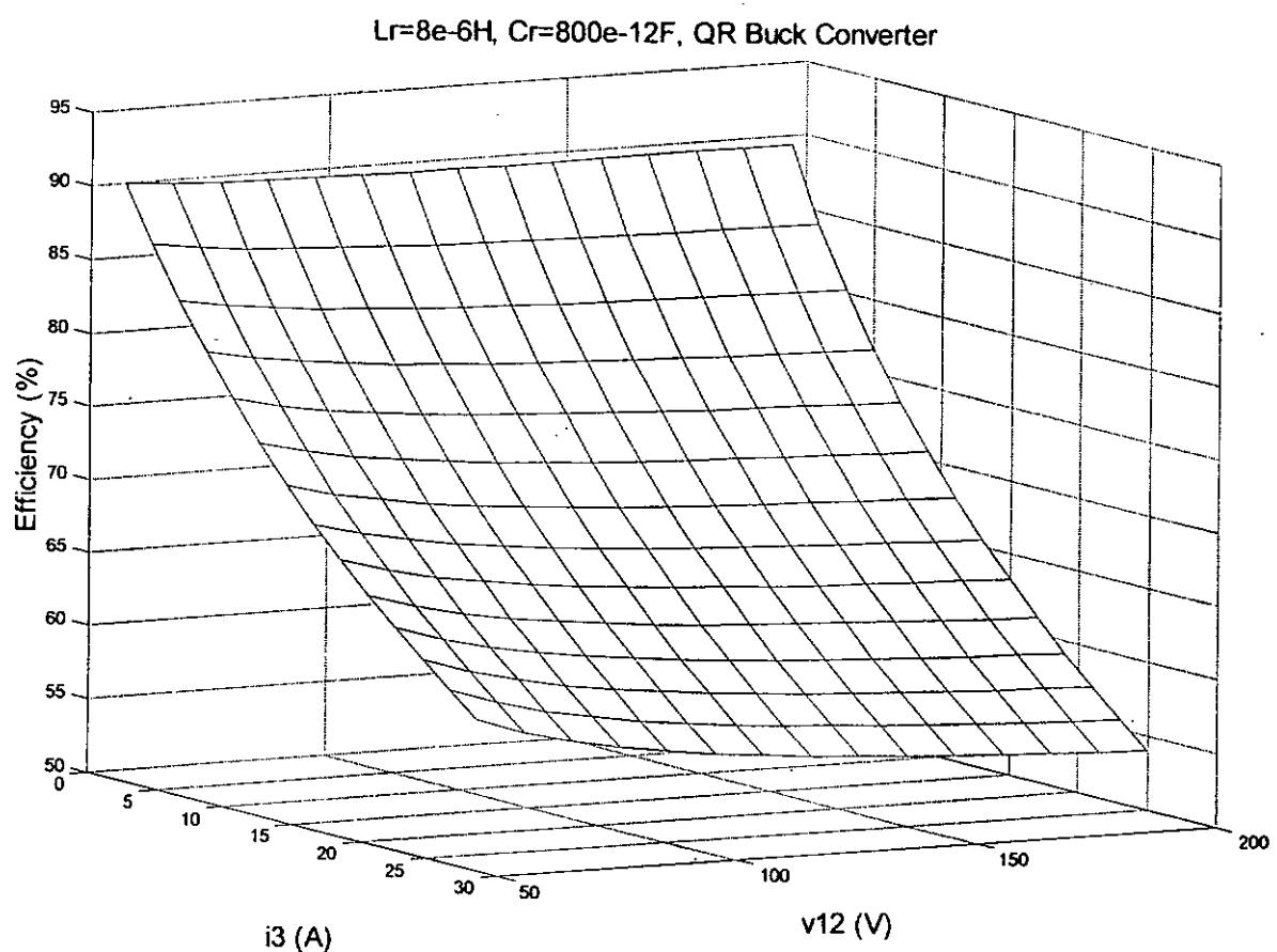
Fig. 7.14. Efficiency of Half-wave Type FM ZVS QR Buck Converter.
