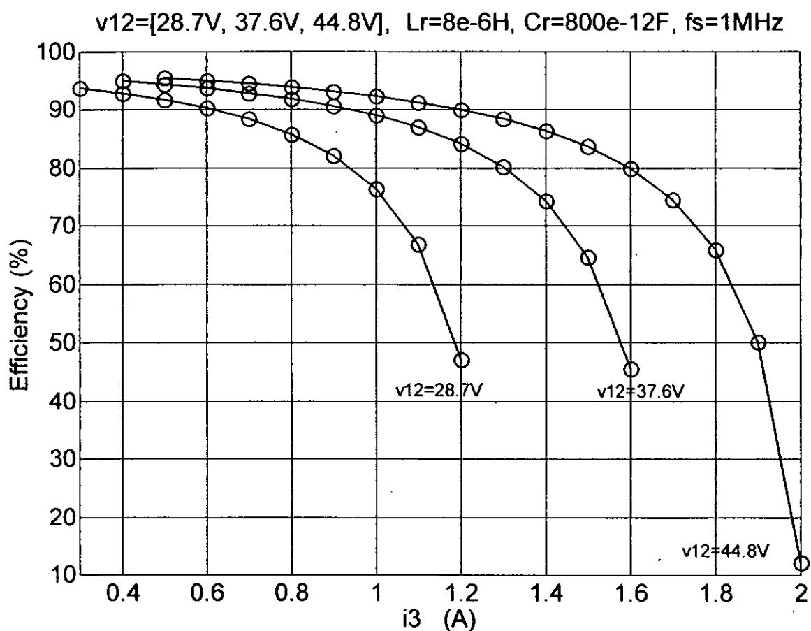
Fig. 7.5. Efficiency of Half-wave Type of FM ZVS QR Buck Converter.
