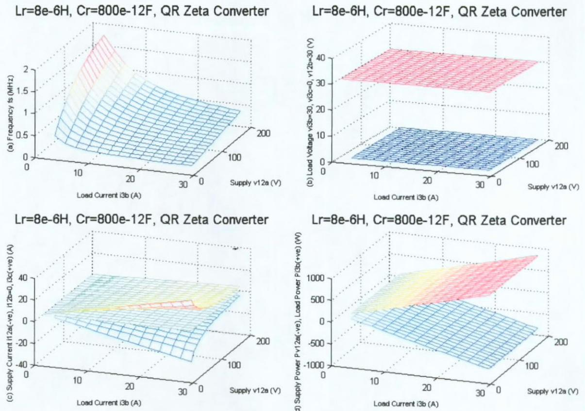
Fig. 7.12. QR Regulated Zeta Converter (a) Switching Frequency  $f_s$ , (b) Regulated Load Voltage  $V_{i3b}$  & Intermediate Voltage Branch  $V_{12b}$ ,  $V_{i3c}$  (c) Supply Current  $Iv_{12a}$  & Intermediate Current Branch  $Iv_{12b}$ ,  $I_{3c}$  (d) Supply Power  $Pv_{12a}$  and Load Power  $P_{i3b}$ .
