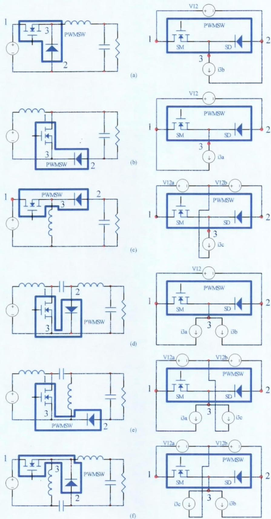
Fig. 2.2. Conventional PWM Converters. Left: Basic Circuits. Right: Operation Models. (a) Buck, (b) Boost, (c) Buck-Boost, (d) Cuk, (e) Sepic and (f) Zeta.
