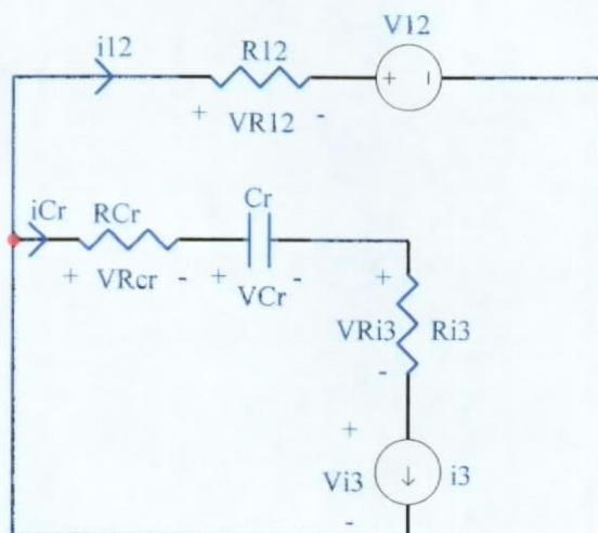
Fig. 5.1. Capacitor Charging Stage  $[T_0, T_1]$  of FM ZVS QR Boost Converter.
