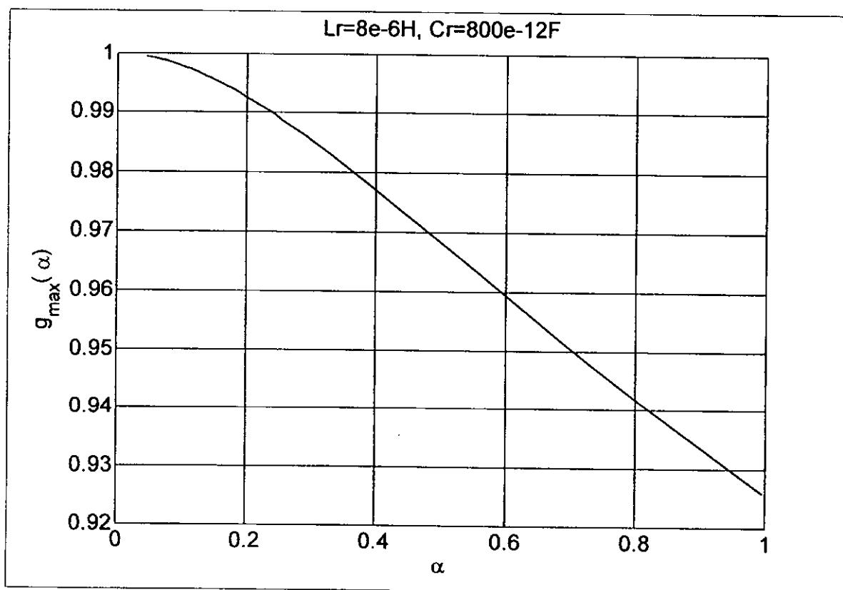
Fig. 2.6. Maximum Transfer Function  $g_{\max}(\alpha)$  at  $f_{\max}(\alpha)$ .
