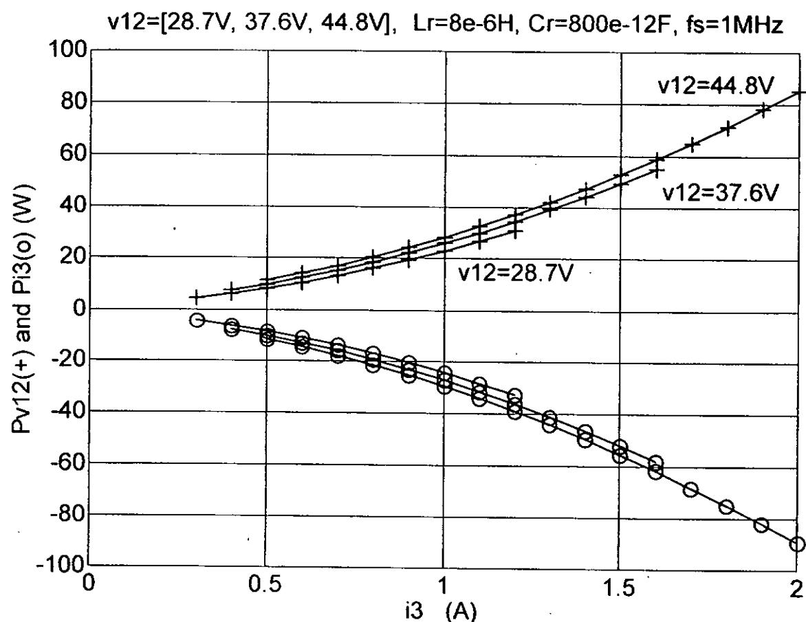
Fig. 7.2. Power Distribution of Half-wave Type of FM ZVS QR Boost Converter.
