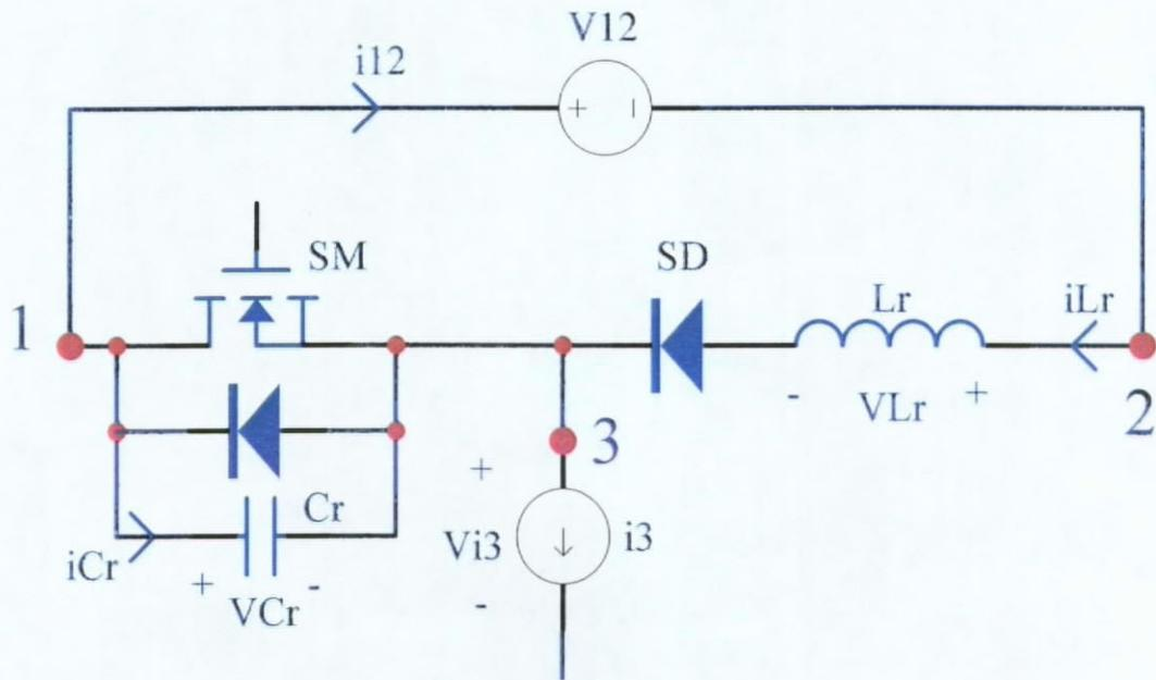
Fig. 2.4. Operational Ideal Model of FM ZVS QR Switch.
