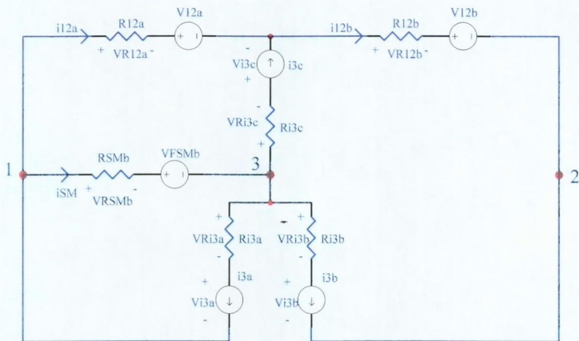
Fig. 6.6. Free-Wheeling Stage [T<sub>3</sub>, T<sub>s</sub>] of FM ZVS QR Unified Model.
