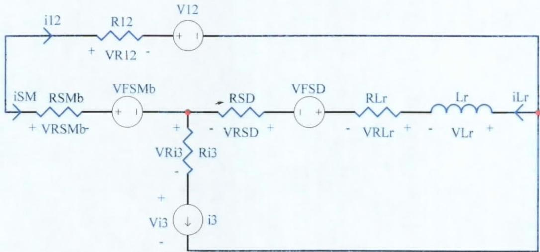
Fig. 4.5. Inductor Discharging Stage [ $T_a, T_3$ ] of FM ZVS QR Buck Converter.
