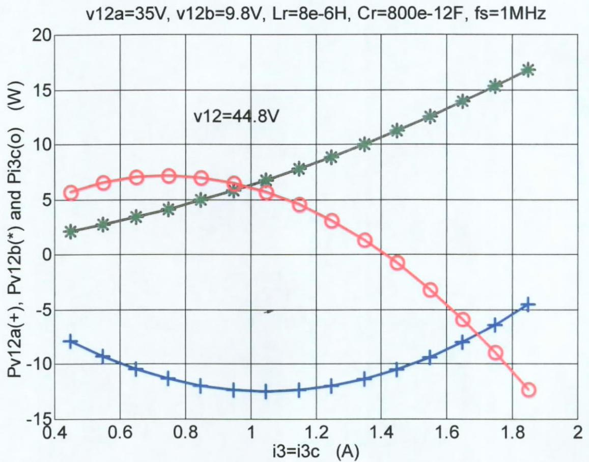
Fig. 3.3. Power Distribution of Half-wave Type of FM ZVS QR Buck-Boost Converters.
