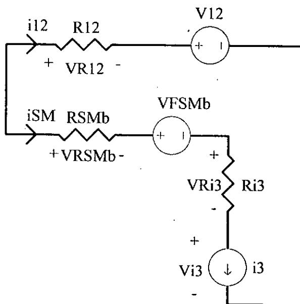
Fig. 4.6. Free-Wheeling Stage  $[T_3, T_s]$  of FM ZVS QR Buck Converter.
