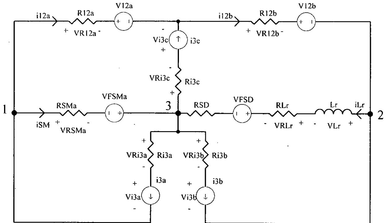
Fig. 6.4. First Inductor Discharging Stage [T<sub>2</sub>, T<sub>a</sub>] of FM ZVS QR Unified Model.
