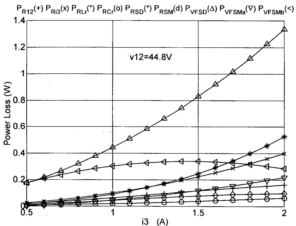
Fig. 7.3. Power Loss of Each Component in FM ZVS QR Buck Converter.
