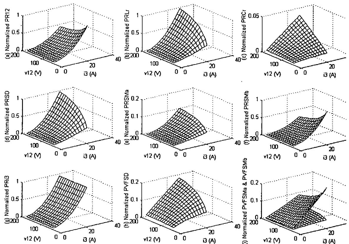
Fig. 7.13. Power Loss of Each Component in FM ZVS QR Buck Converter.
