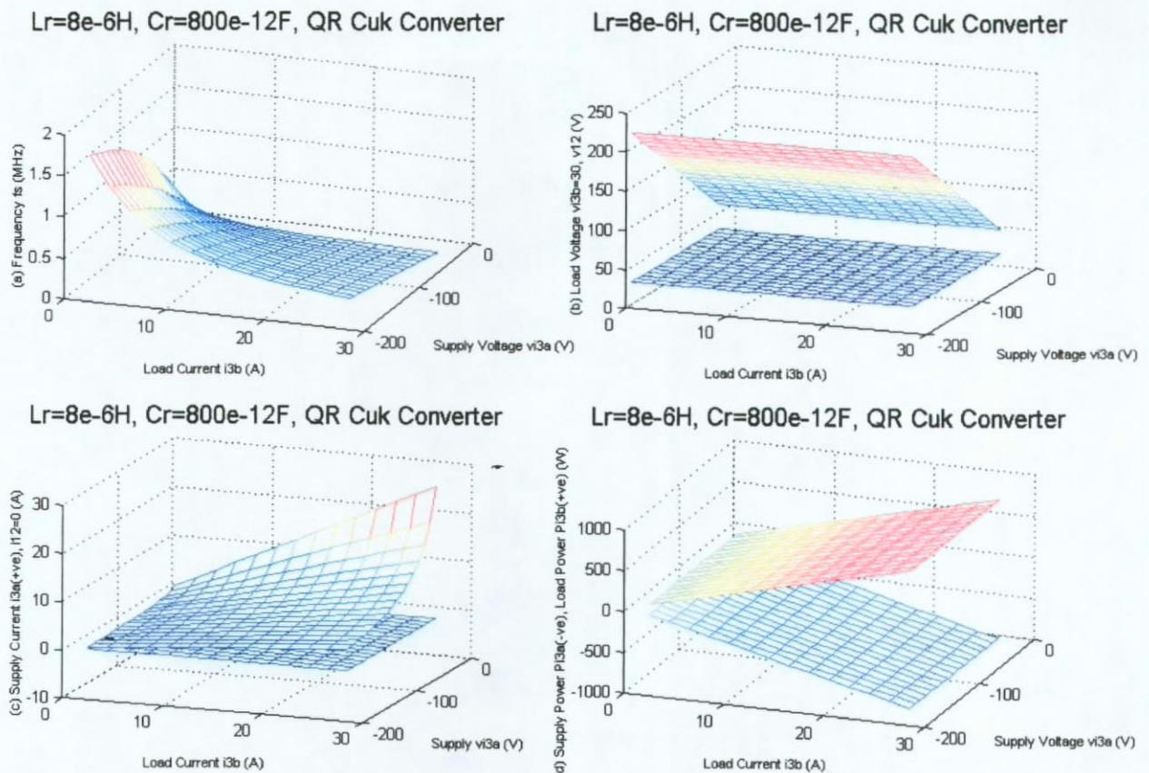
Fig. 7.10. QR Regulated Cuk Converter (a) Switching Frequency  $f_s$ , (b) Regulated Load Voltage  $V_{i3b}$  & Intermediate Voltage Branch  $V_{12}$ , (c) Supply Current  $I_{3a}$  & Intermediate Current Branch  $Iv_{12}$ , (d) Supply Power  $P_{i3a}$  and Load Power  $P_{i3b}$ .
