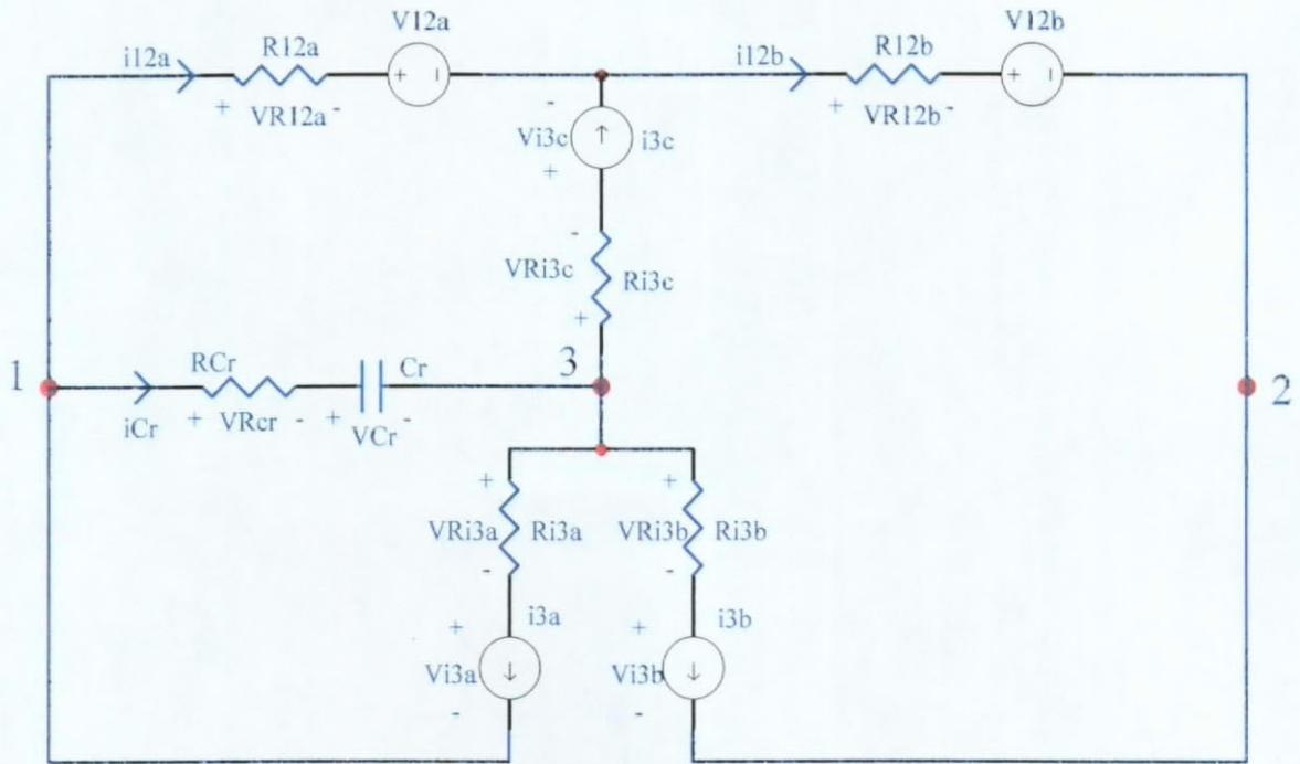
Fig. 6.2. Capacitor Charging Stage  $[T_0, T_1]$  of FM ZVS QR Unified Model.
