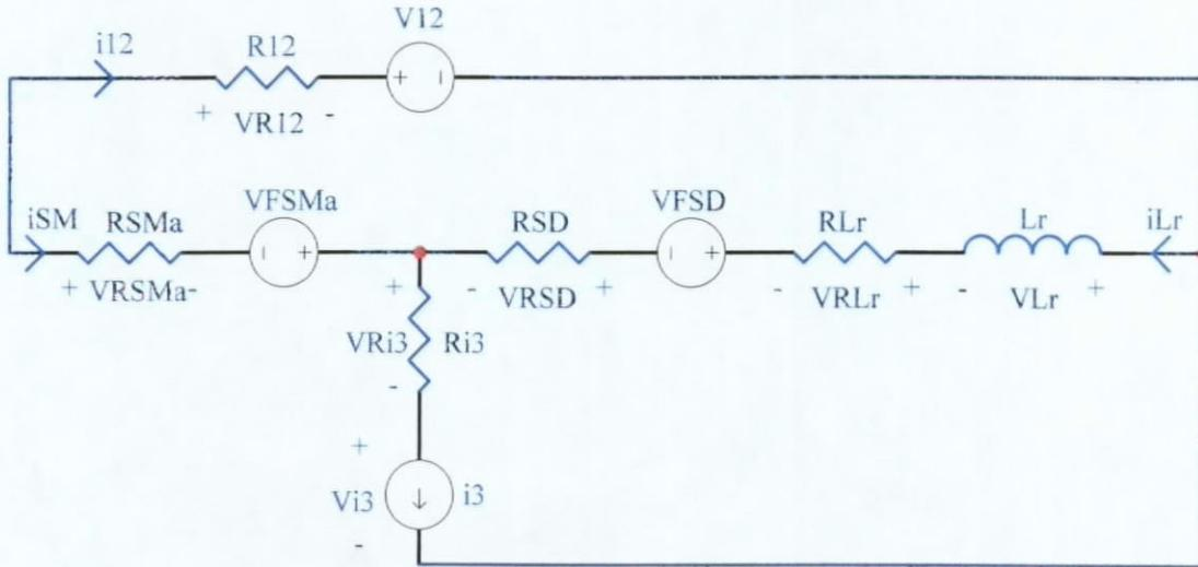
Fig. 4.4. Inductor Discharging Stage  $[T_2, T_a]$  of FM ZVS QR Buck Converter.
