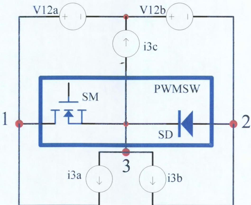
Fig. 2.3. General Operation Model of Conventional PWM Converters.
