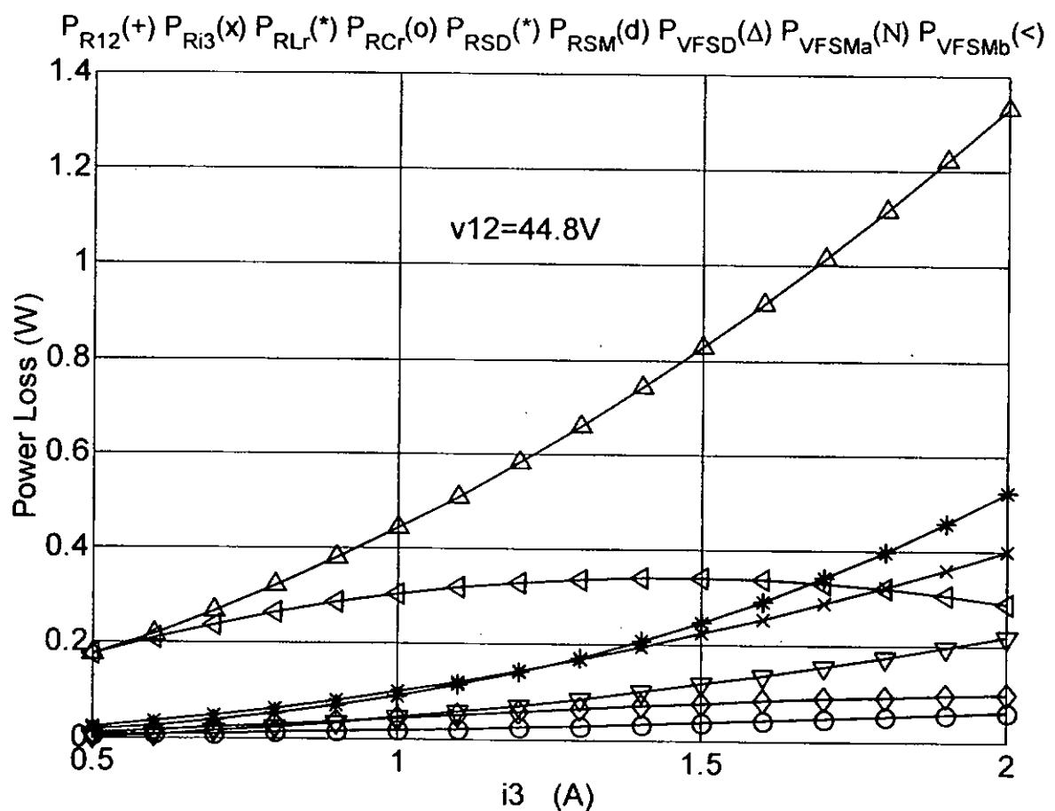
Fig. 7.4. Power Loss of Each Component in FM ZVS QR Boost Converter.
