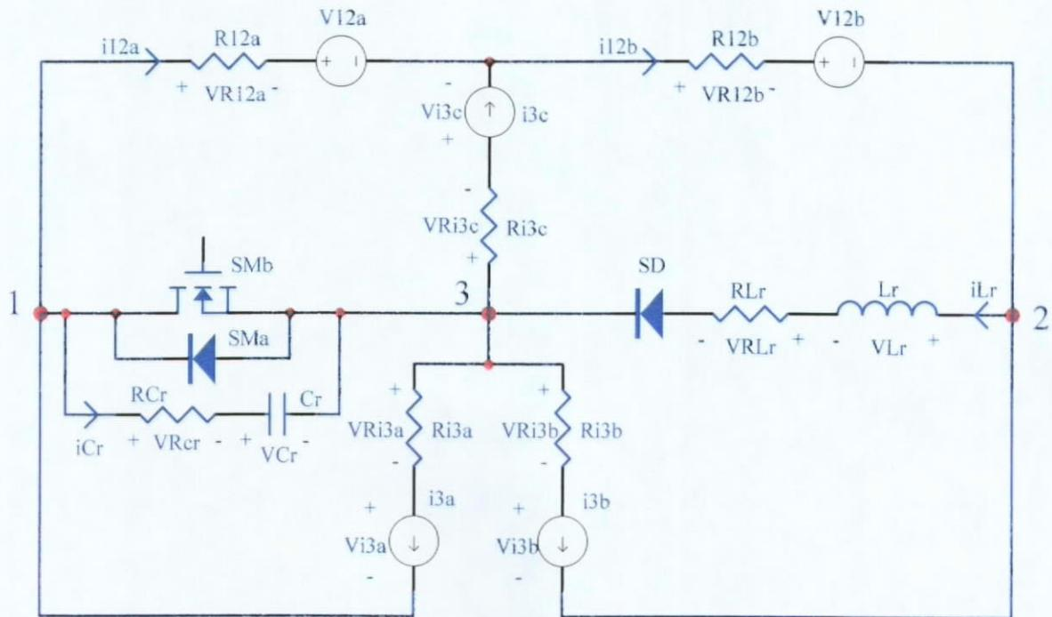
Fig. 6.1. Unified Practical Model of FM ZVS QR Converter.
