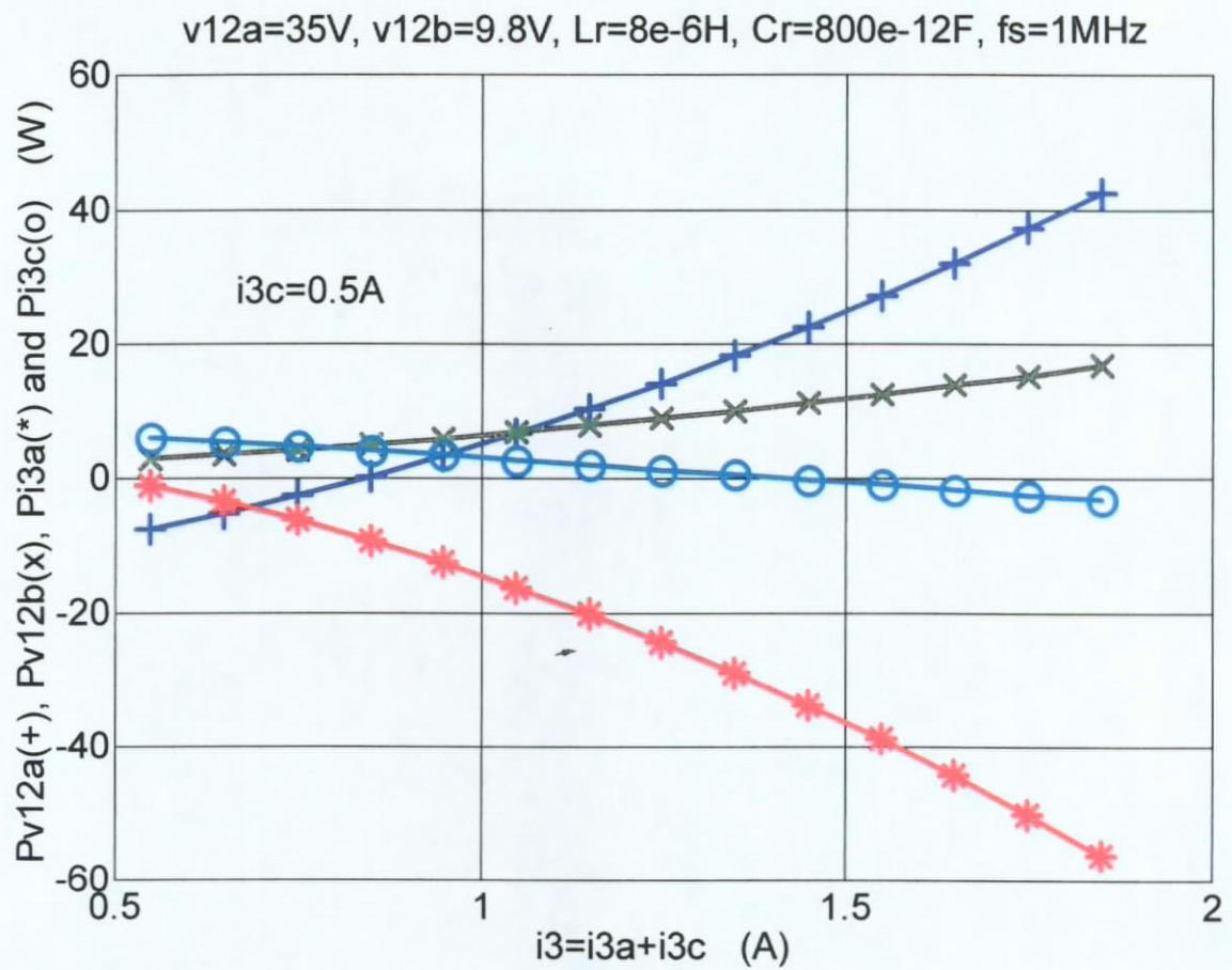
Fig. 3.5. Power Distribution of Half-wave Type of FM ZVS QR Sepic Converters.
