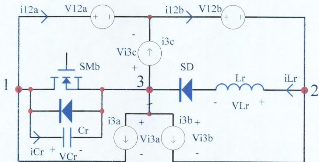
Fig. 2.9. General Operation Model of Half-wave Type of FM ZVS QR Converters.
