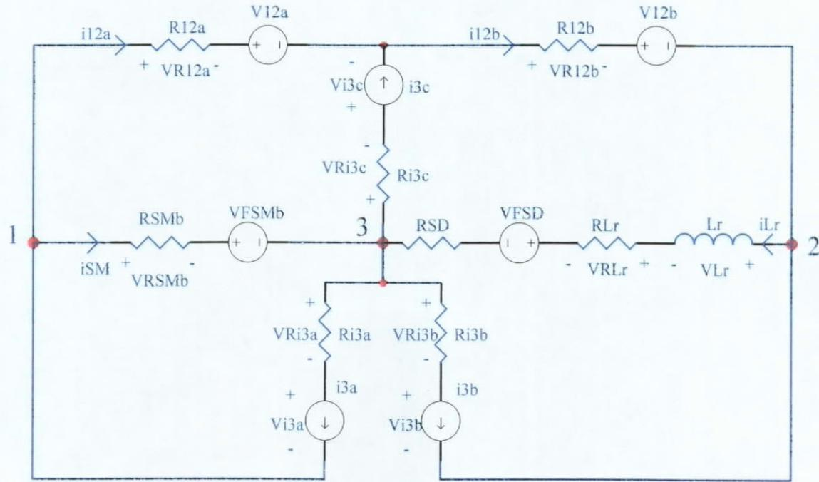
Fig. 6.5. Second Inductor Discharging Stage  $[T_a, T_3]$  of FM ZVS QR Unified Model.
