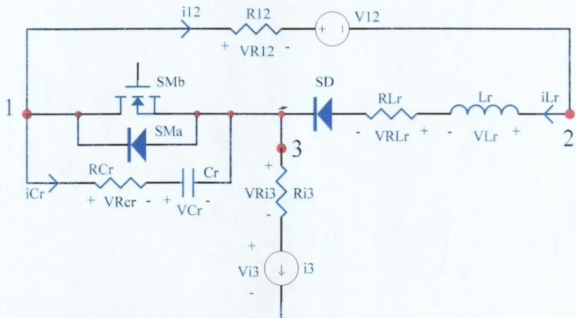
Fig. 4.1. Practical Model of FM ZVS QR Switch.
