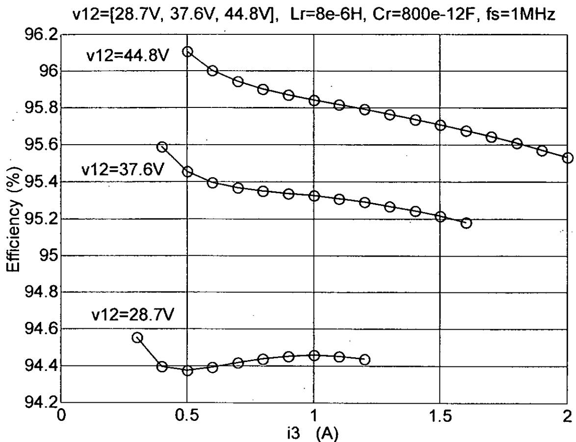
Fig. 7.6. Efficiency of Half-wave Type of FM ZVS QR Boost Converter.
