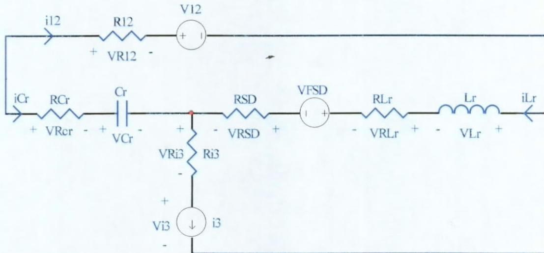
Fig. 4.3. Resonant Stage  $[T_1, T_2]$  of FM ZVS QR Buck Converter.
