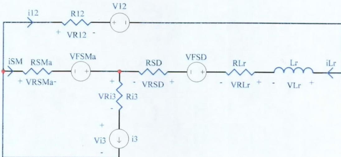
Fig. 5.3. Inductor Discharging Stage  $[T_2, T_a]$  of FM ZVS QR Boost Converter.
