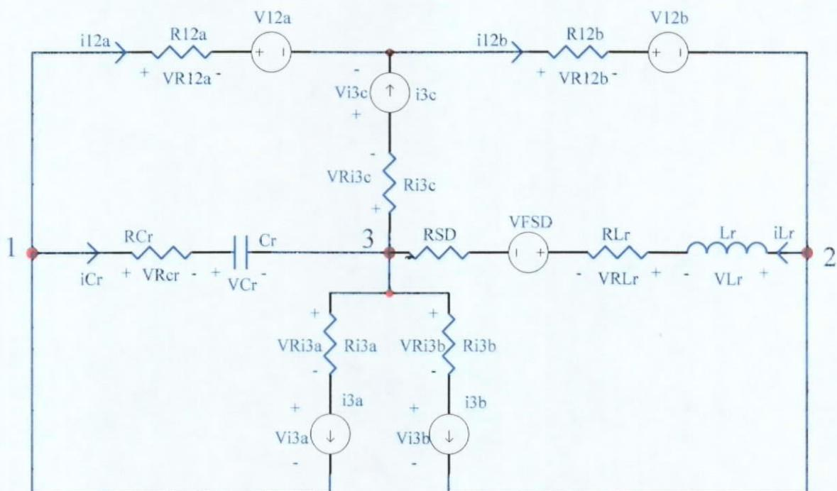
Fig. 6.3. Resonant Stage [ $T_1, T_2$ ] of FM ZVS QR Unified Model.
