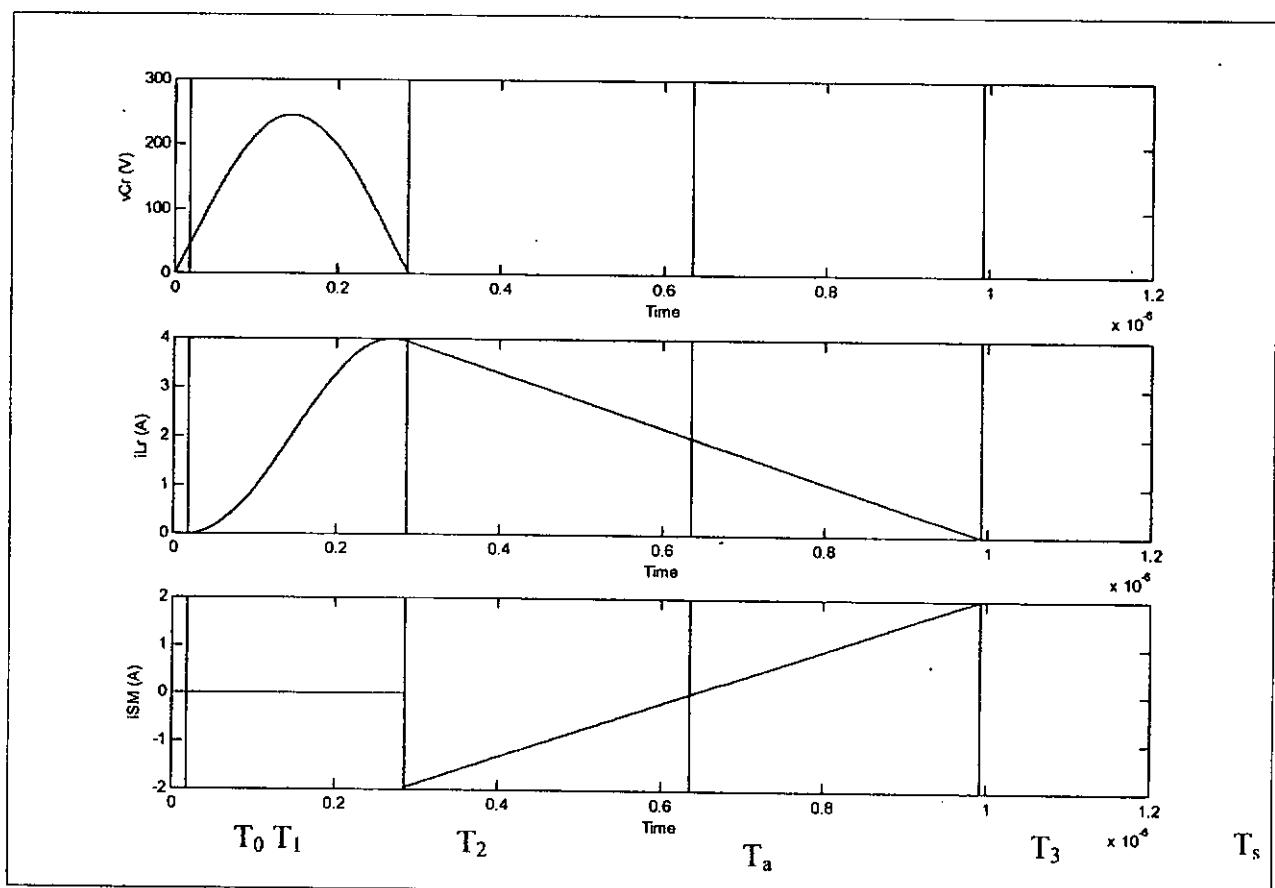
Fig. 2.5. Switching waveforms of FM ZVS QRSW.
