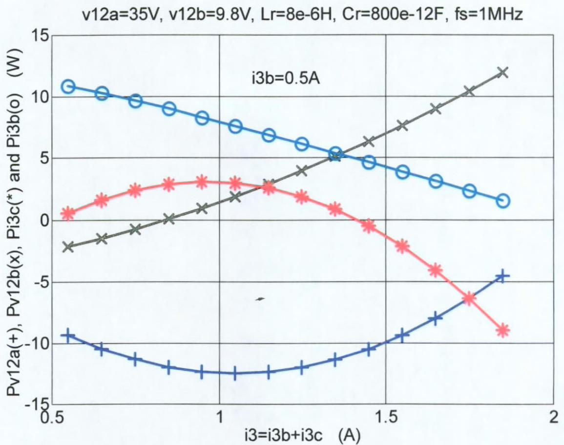
Fig. 3.6. Power Distribution of Half-wave Type of FM ZVS QR Zeta Converters.
