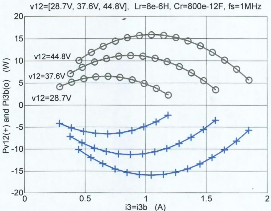
Fig. 3.1. Power Distribution of Half-wave Type of FM ZVS QR Buck Converters.
