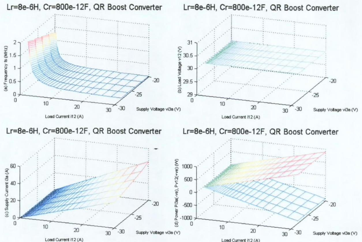
Fig. 7.8. QR Regulated Boost Converter (a) Switching Frequency  $f_s$ , (b) Regulated Load Voltage  $V_{12}$ , (c) Supply Current  $I_{3a}$ , (d) Supply Power  $P_{i3a}$  and Load Power  $P_{V12}$ .
