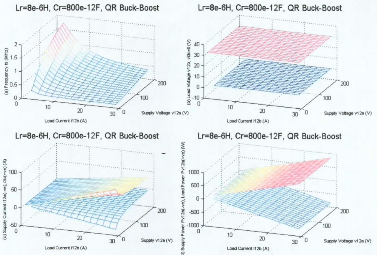
Fig. 7.9. QR Regulated Buck-Boost Converter (a) Switching Frequency  $f_s$ , (b) Regulated Load Voltage  $V_{12b}$  & Intermediate Voltage Branch  $V_{i3c}$ , (c) Supply Current  $I_{12a}$  & Intermediate Current Branch  $I_{3c}$ , (d) Supply Power  $P_{v12a}$  and Load Power  $P_{v12}$ .
