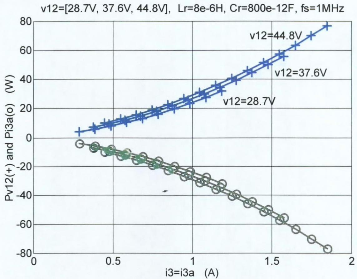
Fig. 3.2. Power Distribution of Half-wave Type of FM ZVS QR Boost Converters.
