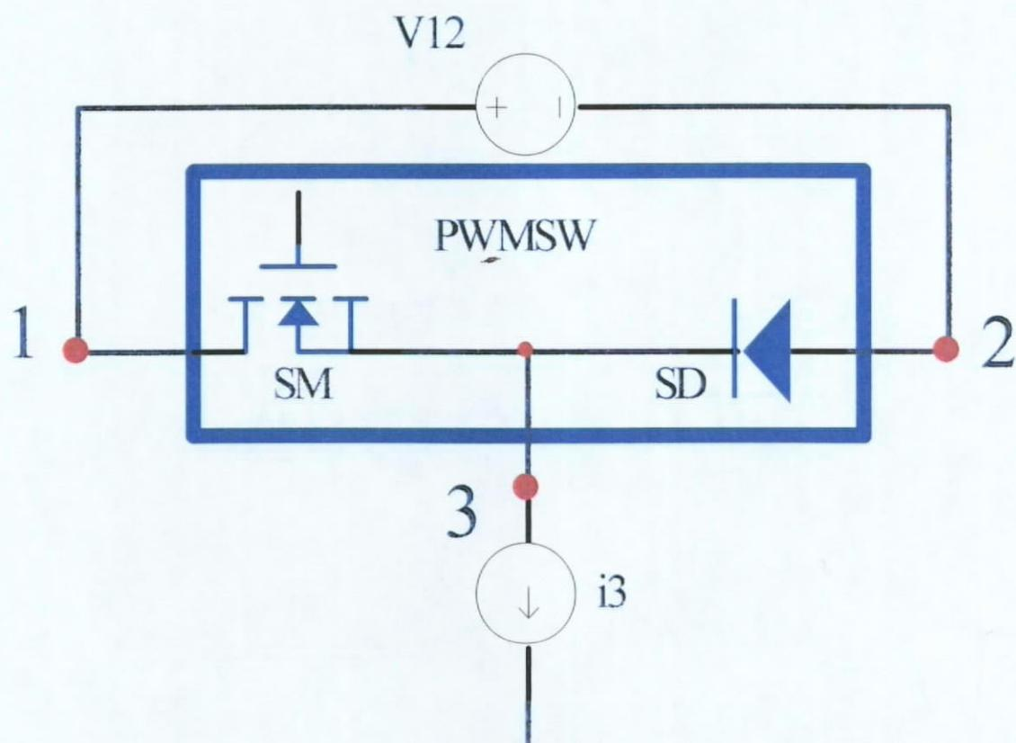
Fig. 2.1. Unified Model of PWM Converters.
