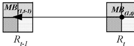
Figure 2.4. Optimal motion vector after video downscaling.
