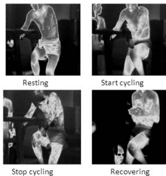
Fig. 5.5 IR photos of the front body during the cycling experiment
