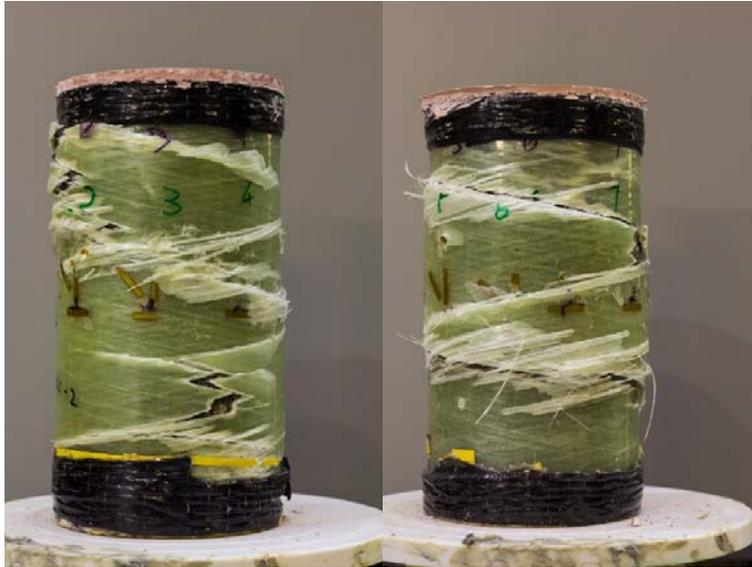
Figure 4.13 Failure mode of specimens 84-0-I & 84-0-II
