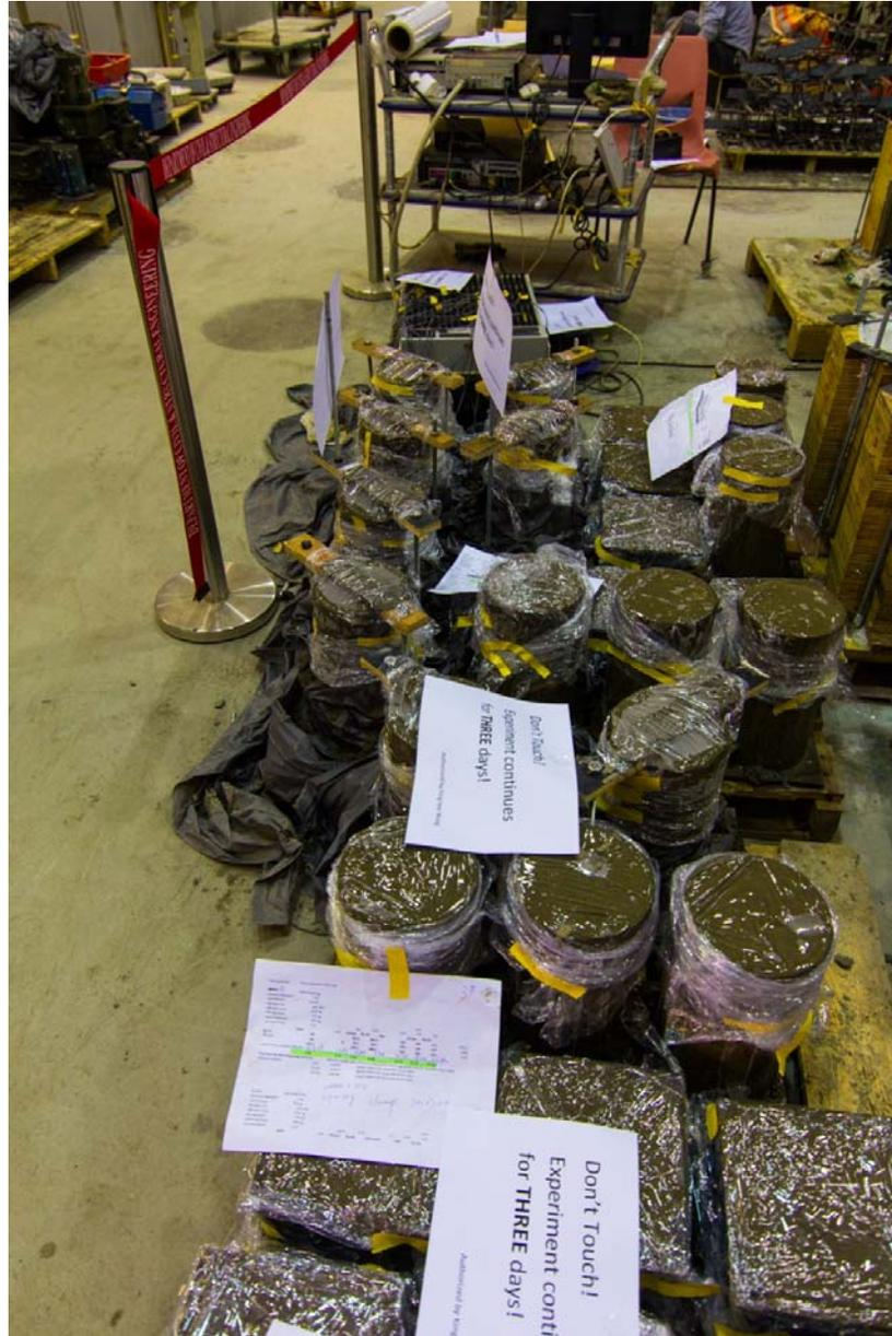
Figure 4.12 Pre-test monitoring and concrete curing
