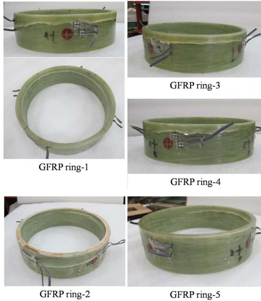
Figure 4.7 Failure mode of ring specimens under axial compression
