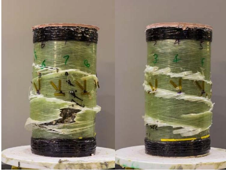
Figure 4.15 Failure mode of specimens 84-12-I & 84-12-II
