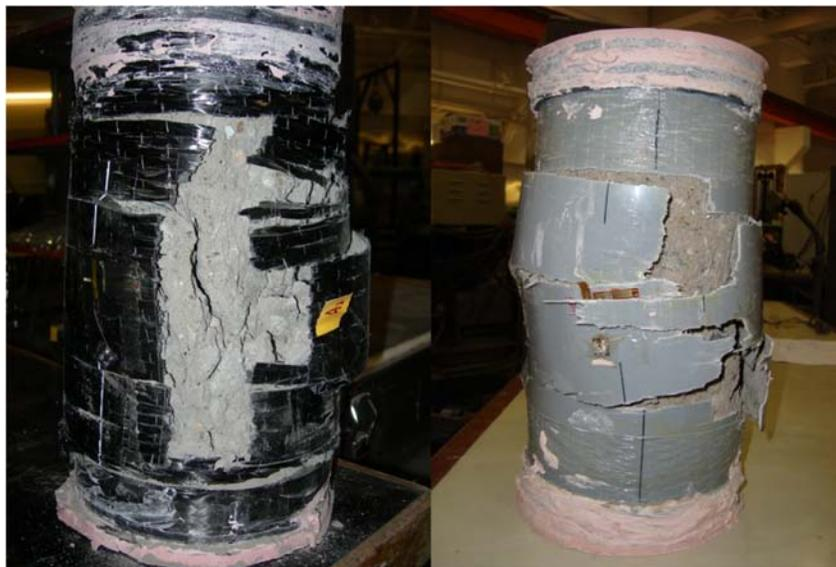
Figure 3.3 Typical failure mode of CFRP and GFRP jacket
