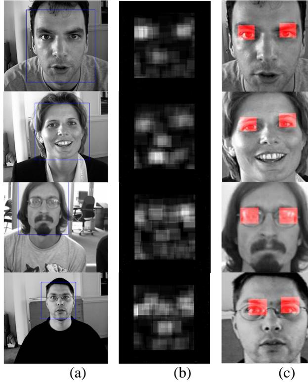
Fig. 2.8. Examples of coarse eye-region detection results using the improved saliency-detection method with the Db4 wavelet and verification based on PCA: (a) face detection results, (b) the saliency maps, and (c) the detected coarse eye regions using the proposed approach.
