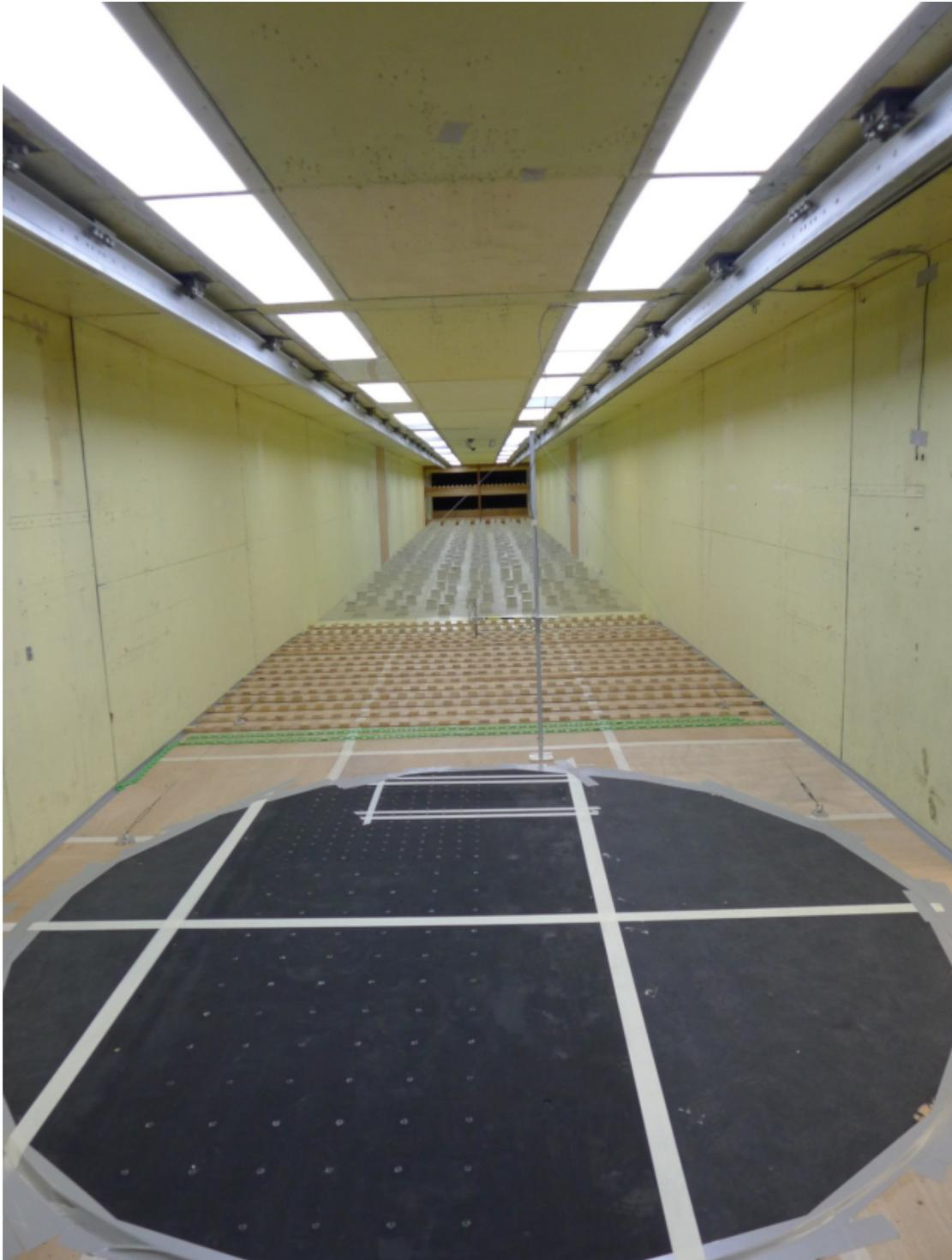
Figure 3-2. Wind tunnel setup for wind profile
