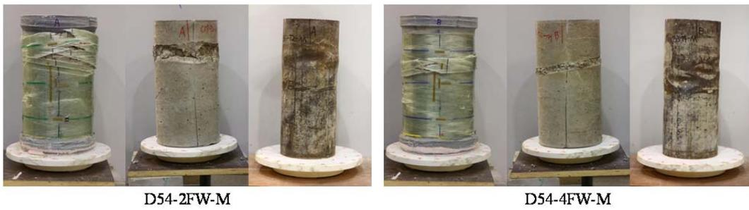
(a) Failed specimens of batch 1
