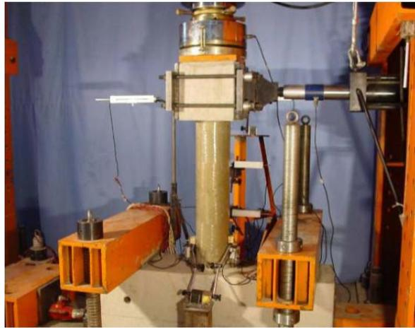
Figure 2.15: Hybrid DSTCs subjected to lateral cyclic loading
