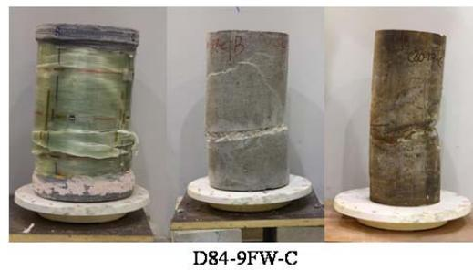
(b) Failed specimens of batch 2
