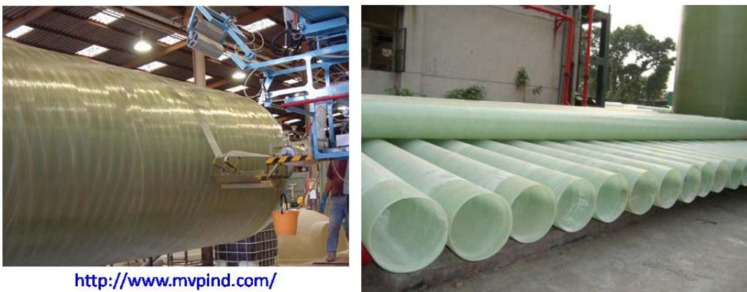
Figure 2.3: FRP tubes fabricated by filament-winding
