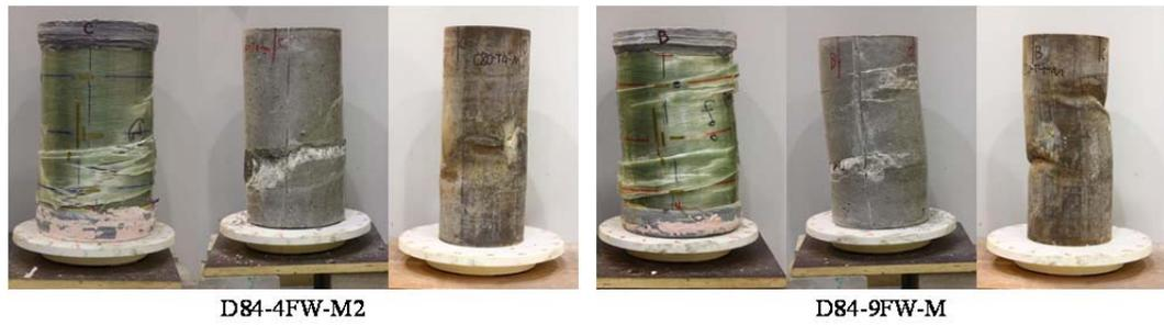
(c) Failed specimens of batch 3
