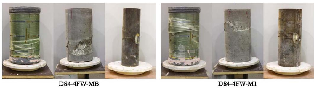
(b) Failed specimens of batch 2
