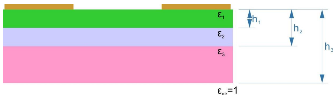
Figure 2-3 The cross-section of two adjacent fingers in IDEs with three-layered structure
