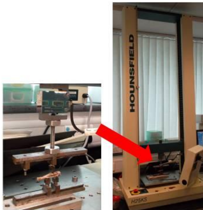
Figure 3.20 Material testing machine and adjustable platform
