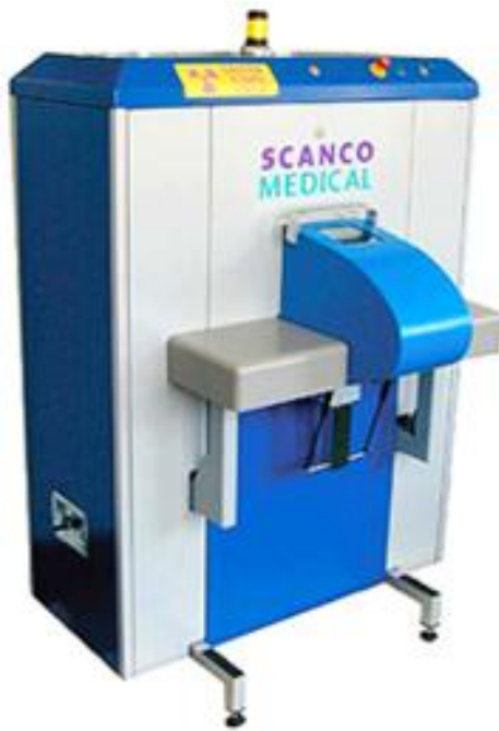
Figure 3.18 High resolution \mu CT scanner and computer system for image analysis
