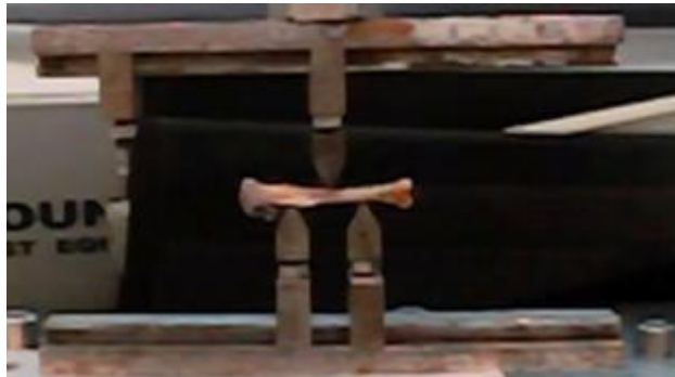
Figure 3.21 Setup and position of tibia for 3-point bending
