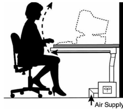
(b) A desk-mounted TAC system [Faulkner et al. 1999]
