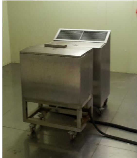
Photo 7 Load Generation Units
