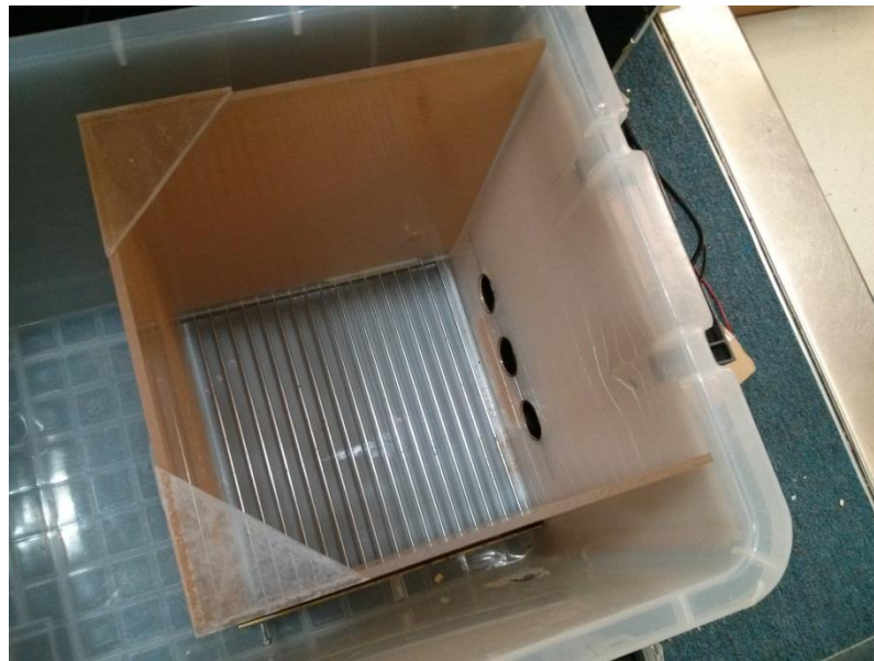
Figure 9. The training box decorated with poking holes and stainless steel grid, for both discrimination task and fear conditioning.
