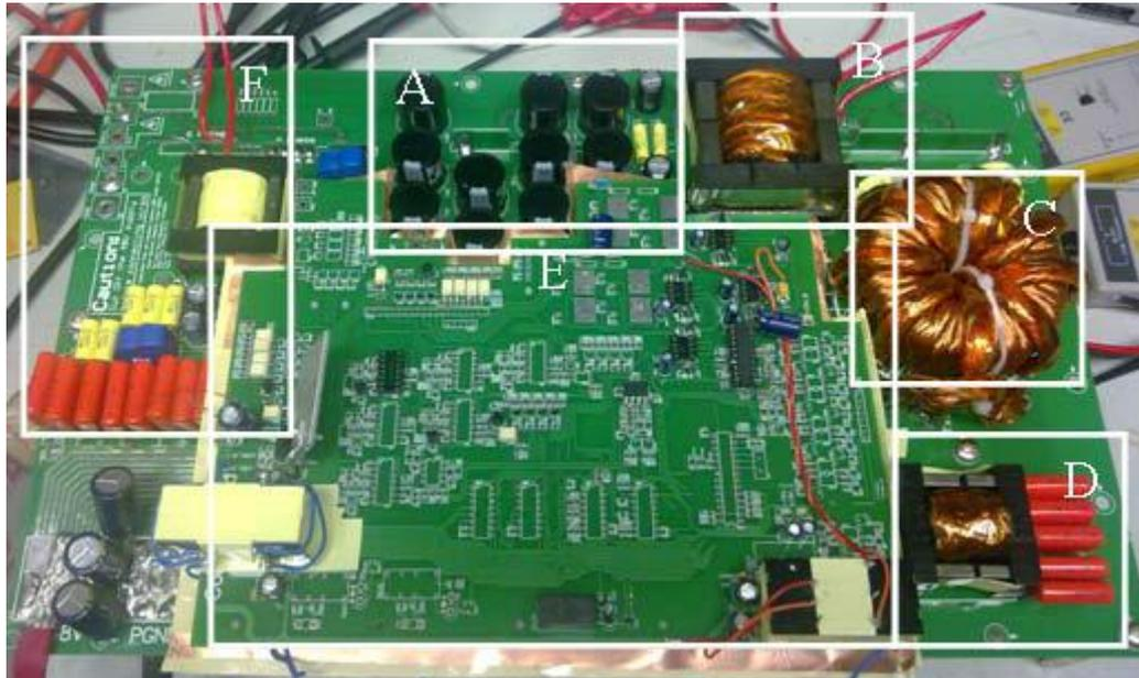
Fig. 2-8 Prototype of the power amplifier
