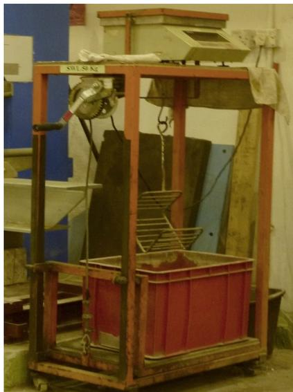
**Figure 3-7 - Equipment for density test**
