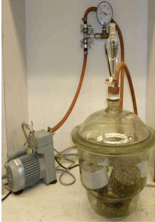
**Figure 3-10 - Desiccator with a vacuum pump**
