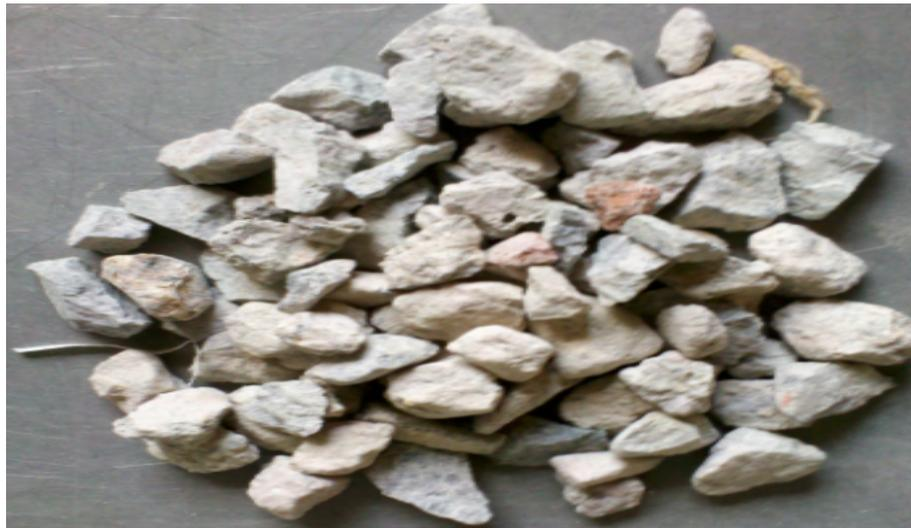
**Figure 2-1 - Recycled aggregate**
