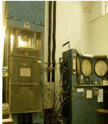
**Figure 3-9 - Specimen and machine used for elastic modulus test**
