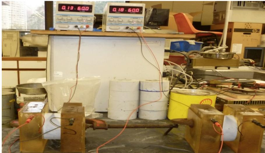
**Figure 3-11 - Apparatus for chloride permeability test**
