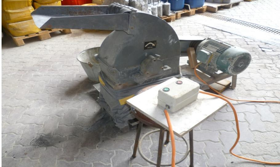
**Figure 3-2 - Laboratory mini-crusher**
