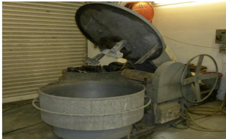
**Figure 3-4 - “Crocker” concrete mixer**
