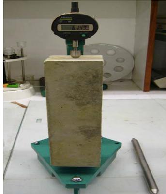
**Figure 3-12 - Apparatus for drying shrinkage test**
