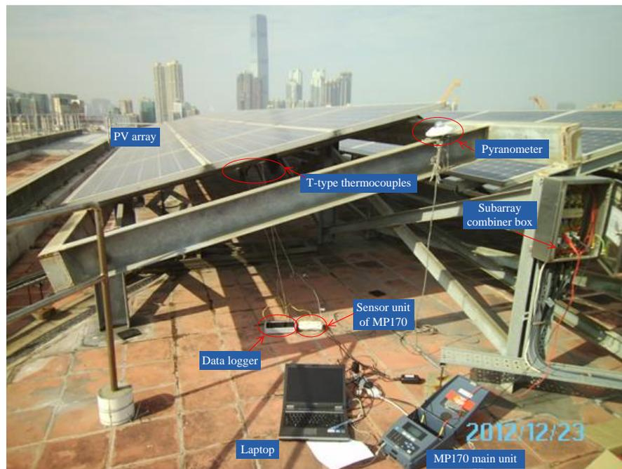
Fig. 3.6 Field measurement instruments and test rig of the 22kWp PV system
