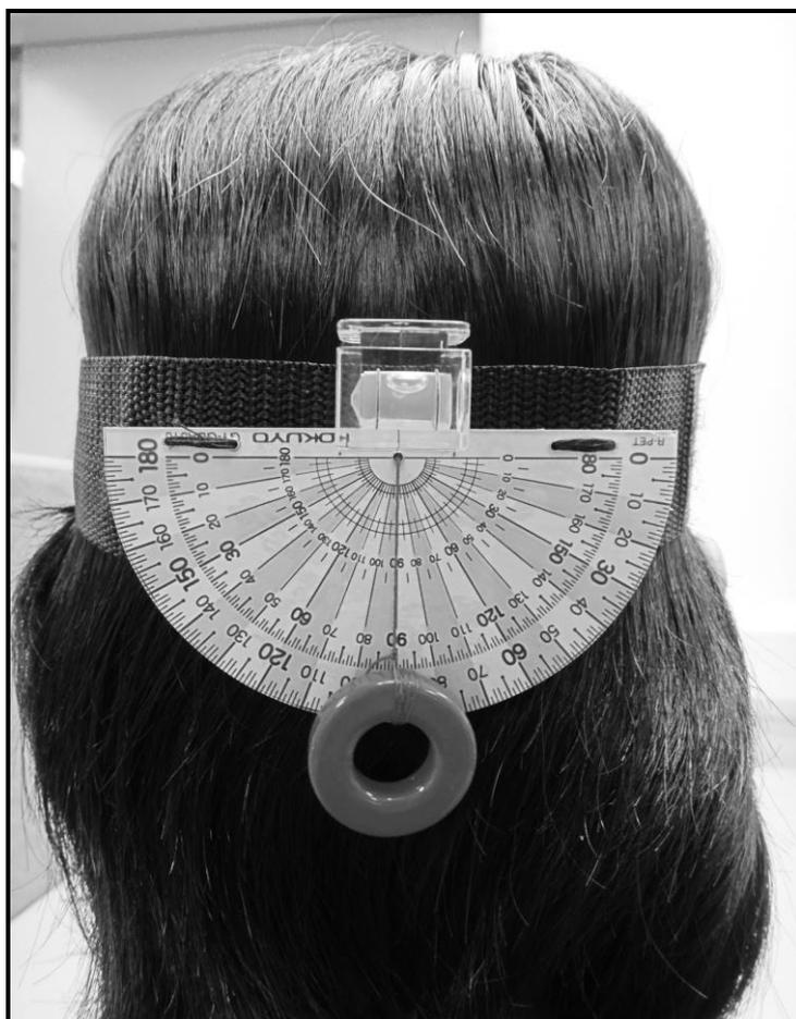
**Figure 3.1** Default head position of a subject, the indicator is aligned with the reading of the protractor at 90°.
