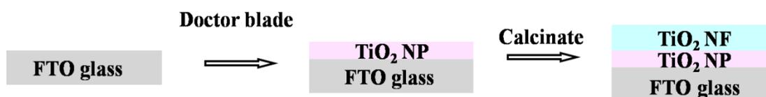
Figure 3.3 Fabrication procedures for EIS test samples.
