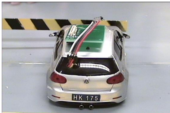
Figure 22 Adapted model car with MicaZ mote.
