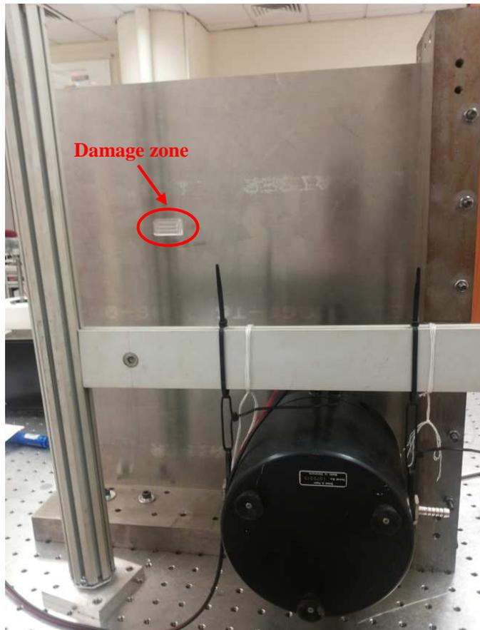
Figure 4.17. Damage zone on the plate
