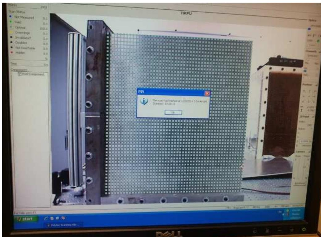
Figure 4.19. Vibration test on the plate with  $49 \times 49$  measurement points
