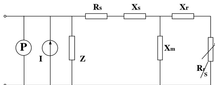
**Figure 5.3** Equivalent circuit of the composite load model
