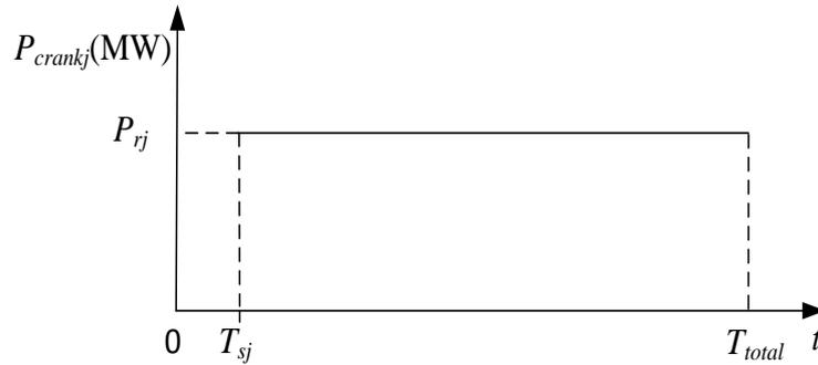
**Figure 3.3** Characteristic of a NBS generator cranking power
