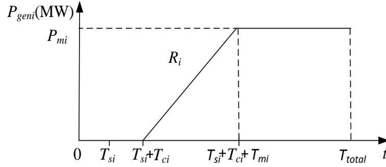
**Figure 3.2** Startup characteristic of a generator
