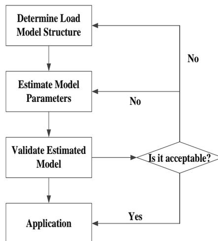
**Figure 5.2** Flow chart of system identification
