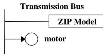
**Figure 6.3** The composite load model at transmission voltage level
