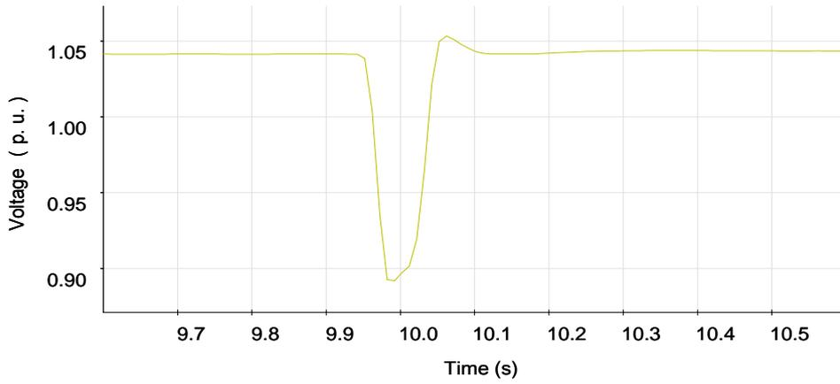
**Figure 6.4** Bus voltage dynamics
