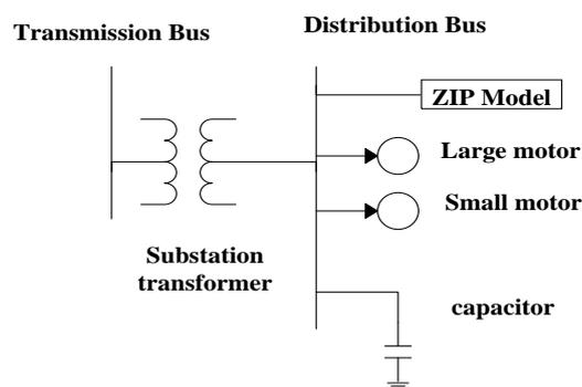
**Figure 6.2** Complete load model at distribution voltage level
