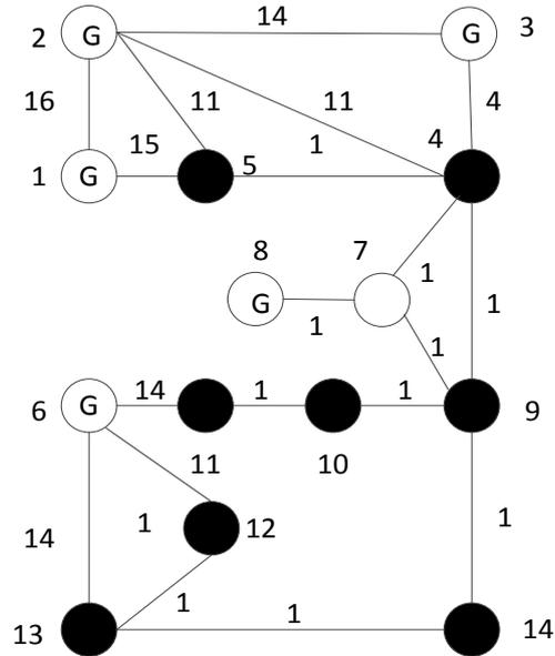
**Figure 4.1** IEEE 14 bus system topology model (where G nodes stand for generators, and black nodes stand for substations)
