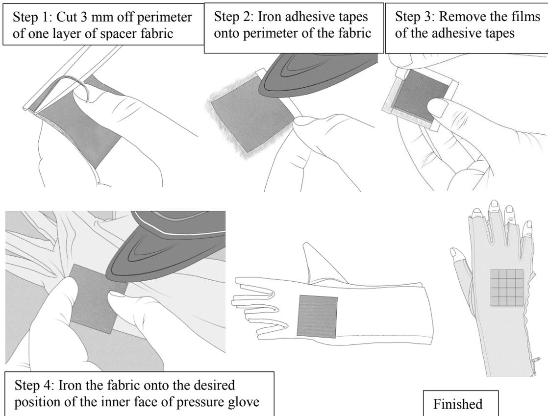
Figure 7.18 Attachment of spacer fabric onto a pressure glove
