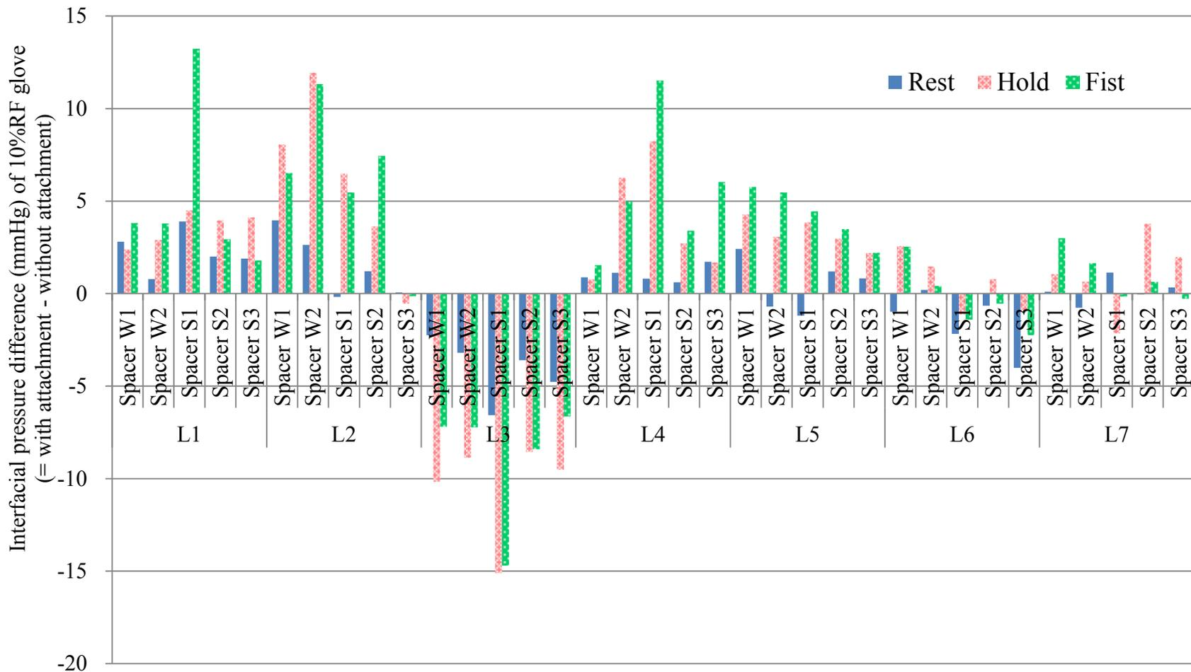
Figure 7.19 Difference between the glove-skin interfacial pressures of a 10% RF glove that has spacer fabric insert attached with adhesive tape and one without insert attachment
