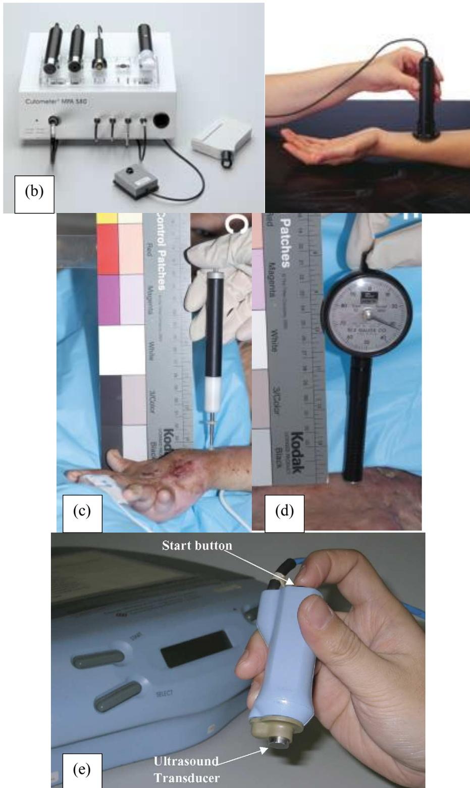
Figure 2.3 Objective scar condition assessment devices: (a) hand-held spectrocoulorimeter [24], (b) cutometer [25], (c) pneumatometer [20], (d) durometer [20] and (e) tissue ultrasound palpation sensor [16]
