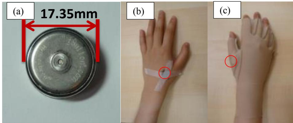
Figure 6.4 (a) Temperature and humidity sensor, (b) placement of the sensor on control hand, (c) placement of the sensor inside gloved hand
