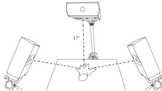
Figure 4.5 Setup for capturing 3 images by 3D scanner with the use of Method IM-III
