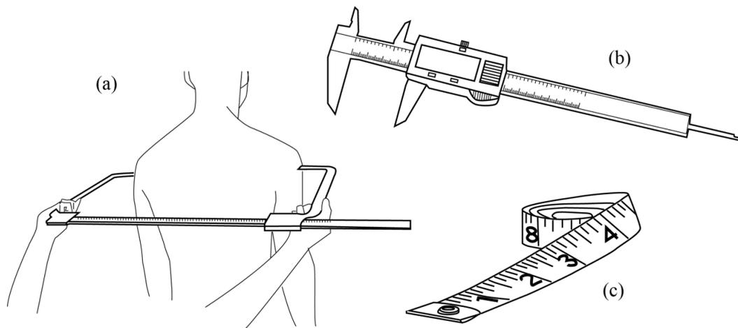
Figure 2.10 (a) Anthropometer, (b) calliper and (c) measuring tape
