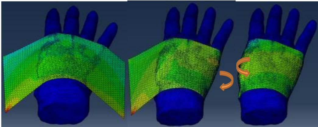
Figure 8.8 Moving the fabric towards and surrounding the hand
