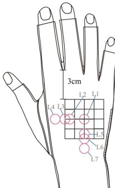
Figure 7.10 Interfacial pressure measurement locations
