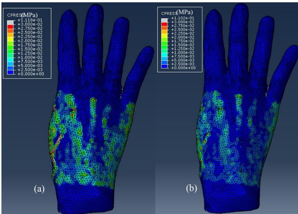
Figure 8.15 Simulation of contact pressure distribution by glove made of Fabric B on hand defined with properties of (a) bone and (b) skin
