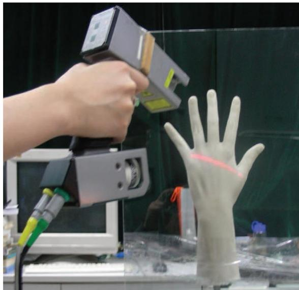
Figure 2.13 Measurement of resin hand model by using a 3D hand-held scanner [134]
