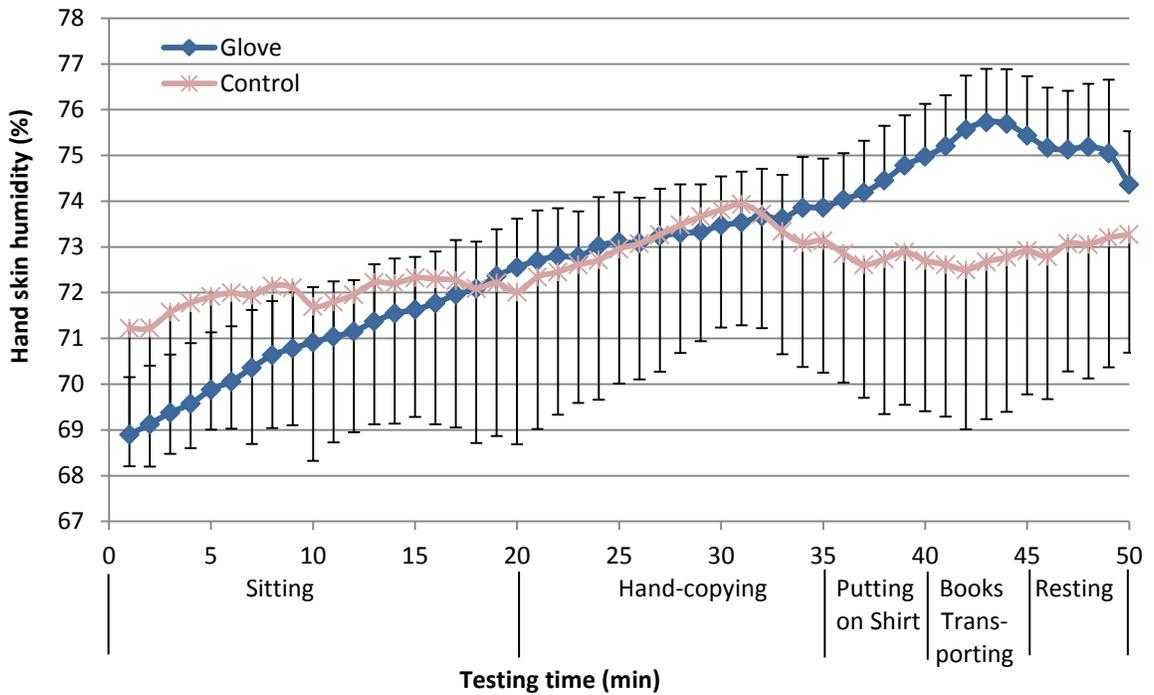
Figure 6.14 Overall hand skin humidity when the pressure gloves are worn in the control condition (n=120, mean  $\pm$  SD)
