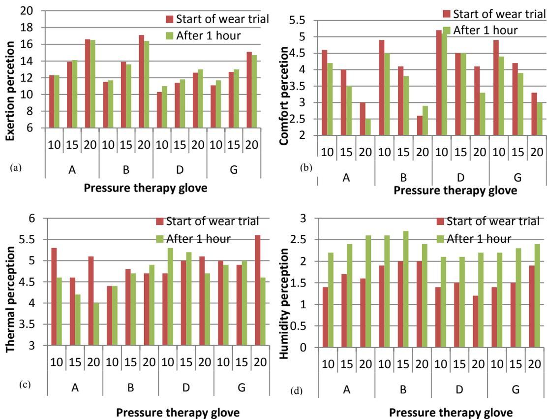
Figure 6.15 Subjective ratings of (a) perceived exertion, (b) comfort perception, (c) thermal perception, (d) humidity perception of pressure gloves made of different fabrics and with different RFs before and after wear trial
