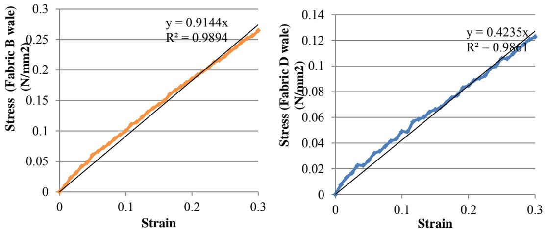
Figure 8.4 Tensile stress-strain curves of wale direction of Fabrics B and D
