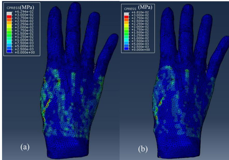
Figure 8.16 Simulation of contact pressure distribution by glove made of Fabric D on hand defined with properties of (a) bone and (b) skin
