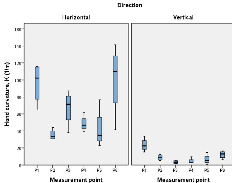
Figure 5.14 Box plots that show hand curvatures of four subjects measured at different points of pressure
