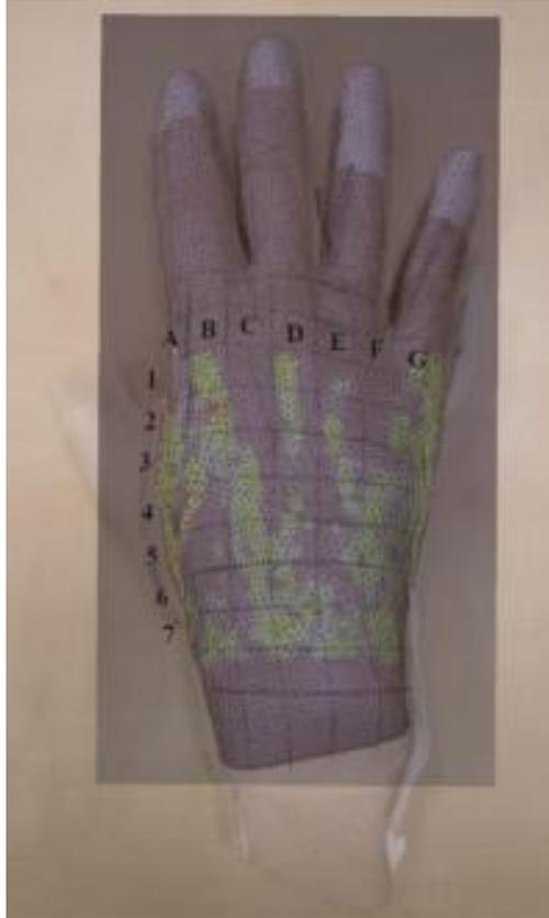
Figure 8.12 Superimposing of the plaster hand with pressure glove and the hand with contact pressure simulation from FEM
