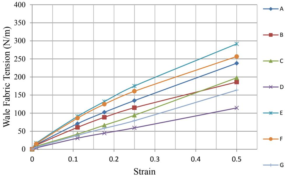
Figure 5.8 Initial fabric tensions in the wale direction of the seven types of fabrics
