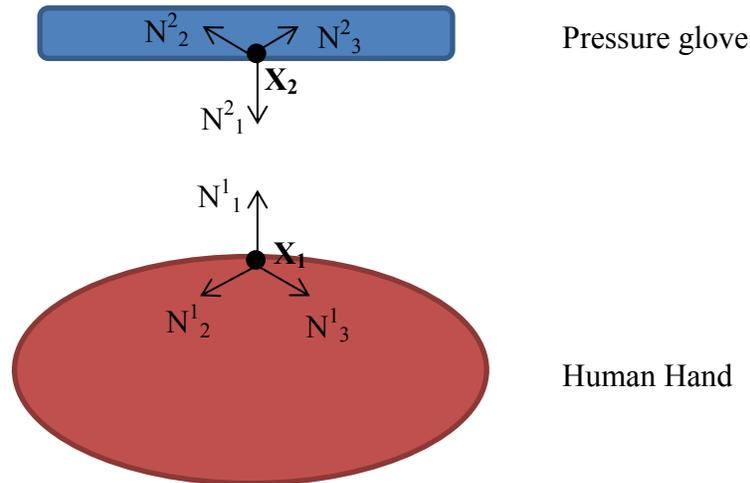
Figure 8.7 Two boundary points and its associated normal and tangential vectors on pressure glove and human hand
