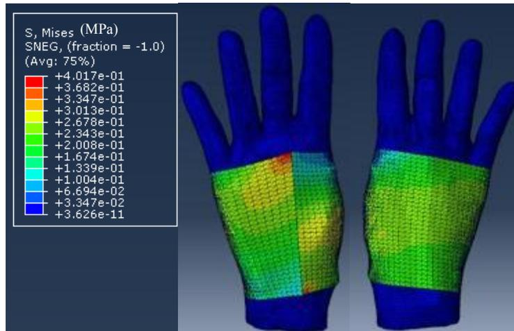
Figure 8.9 Stress distribution on the glove fabric after fully surrounding the hand
