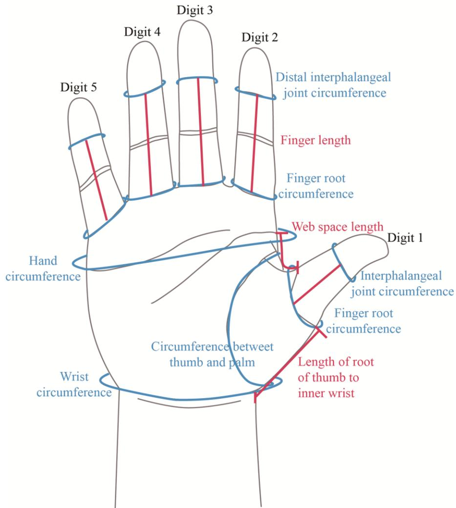
Figure 2.7 Hand dimensions measured by using measuring tape for pressure glove production
