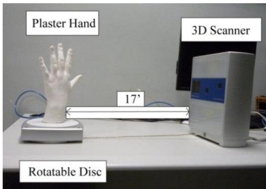
Figure 4.4 Setup for 3D scanning of a plaster hand with the use of Method IM-II
