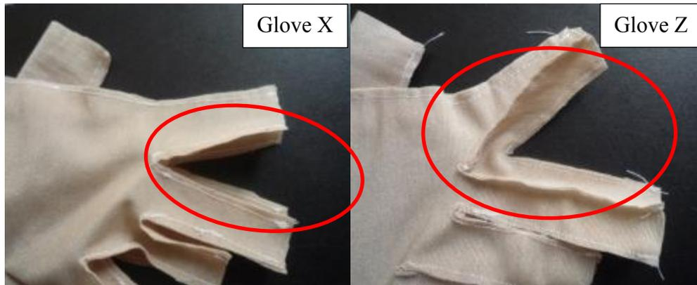
Figure 7.6 Finger web panels of Glove X (with sharp finger web angle) and Glove Z (with widened finger web angle)
