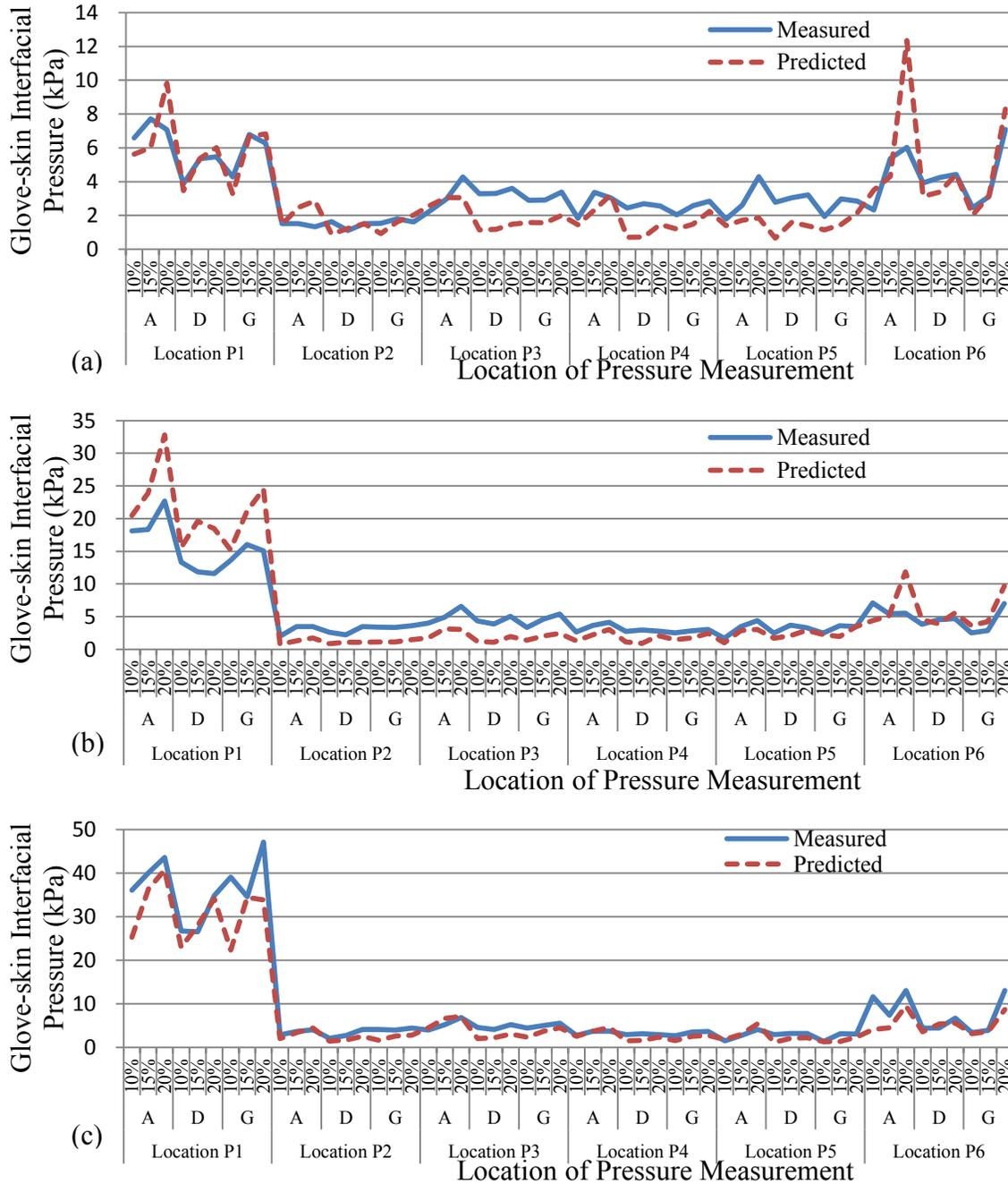
Figure 5.15 Measured and predicted glove skin interfacial pressures (a) when hand is relaxed on table, (b) when hand is holding a cylinder and (c) when hand is made into a clenched fist.
