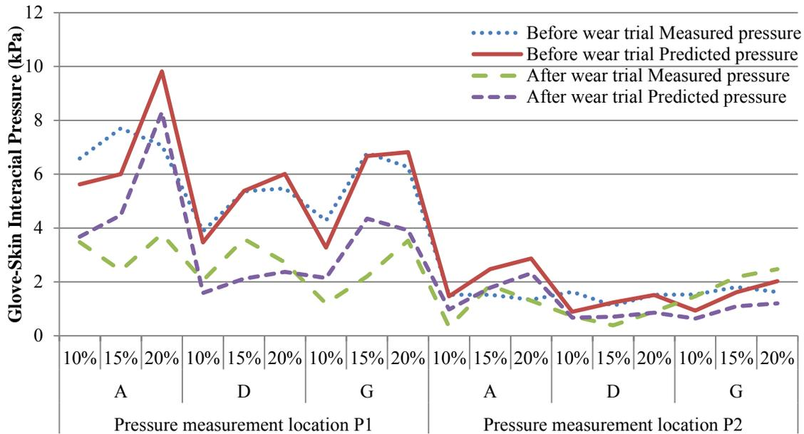
Figure 5.16 Predicted and measured glove-skin interfacial pressures before and after wear trial
