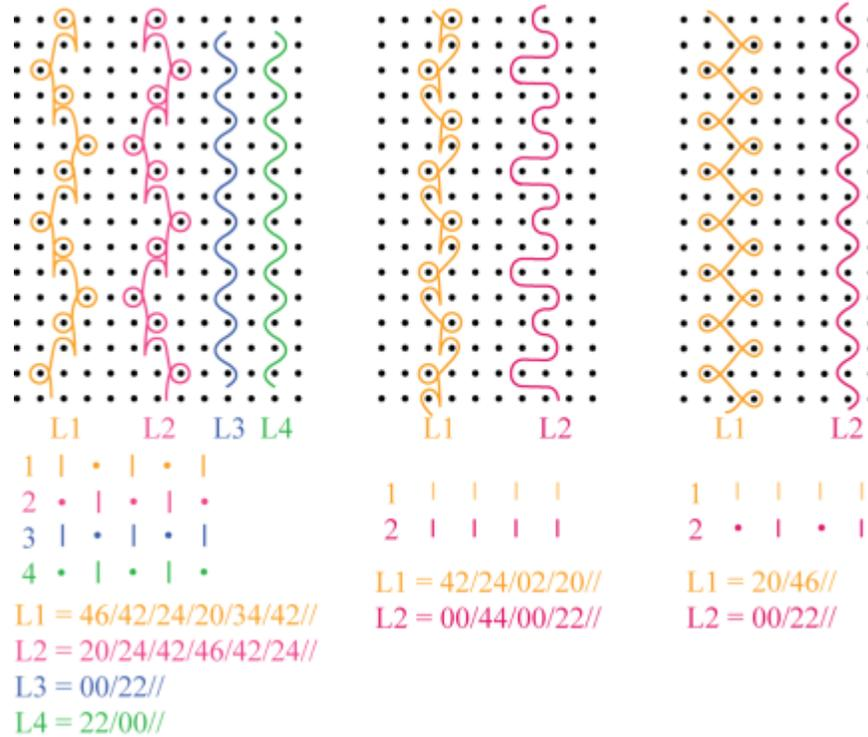
Figure 5.2 Structural diagrams of (a) powernet, (b) satinnet and (c) weftlock fabric
