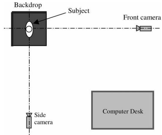
Figure 2.12 Plane view of 2D image capture set up for body anthropometric measurement [130]
