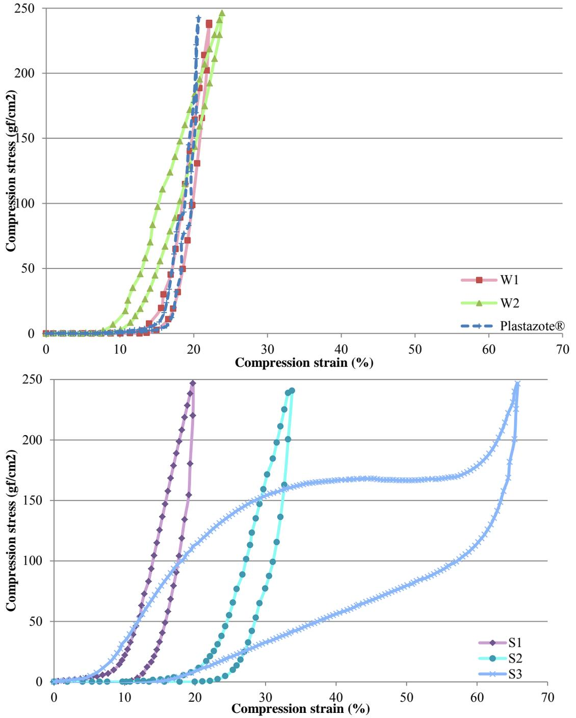
Figure 7.13 Compression stress-strain curves of the five types of spacer fabrics and Plastazote®
