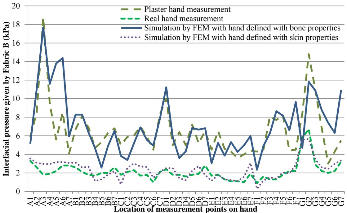
Figure 8.13 Comparison of simulated pressure from FEM and sensor measured pressure on plaster and real hands induced by glove made of Fabric B
