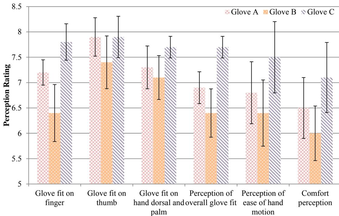
Figure 7.9 Results of the subjective ratings for the three types of pressure gloves (Error bars indicate  $\pm$  SD)
