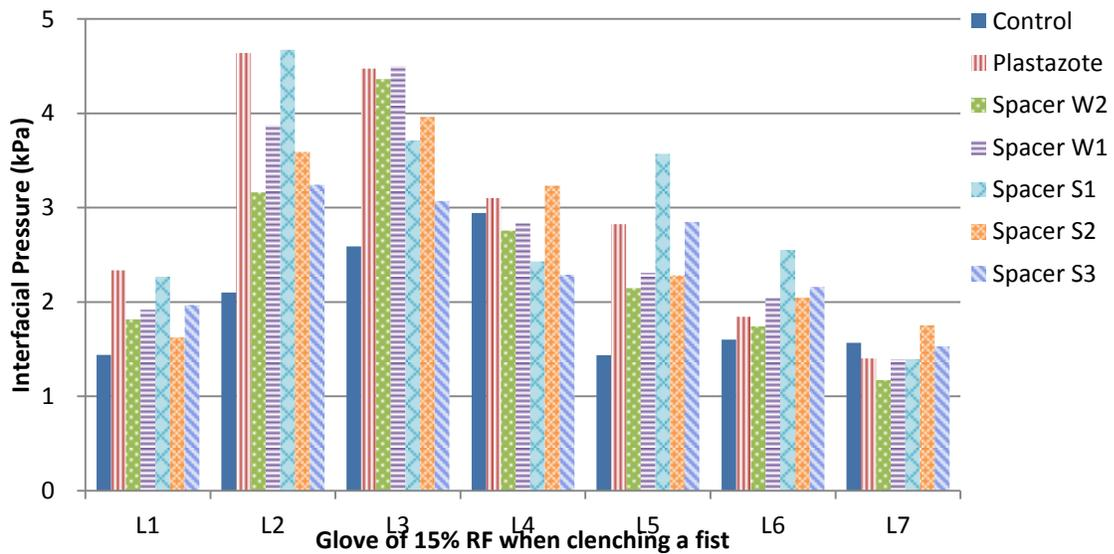
**Appendix VIII** The difference between the glove-skin interfacial pressure given by the spacer fabric attached
