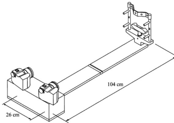
Figure 2.11 Stereophotogrammetric set-up for measuring facial anthropometry [128]
