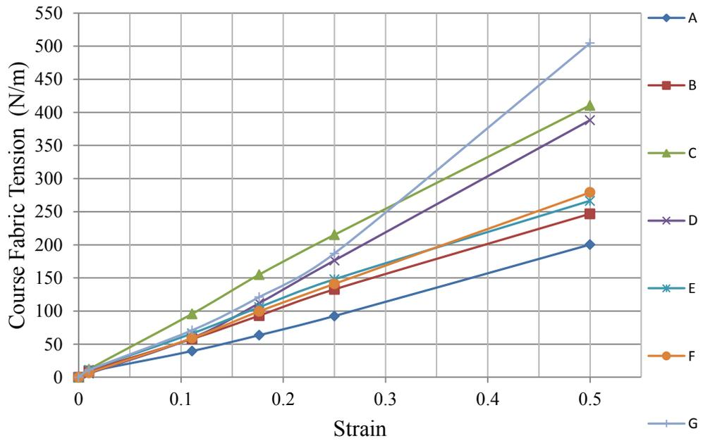
Figure 5.9 Initial fabric tensions in the course direction for the seven types of fabrics
