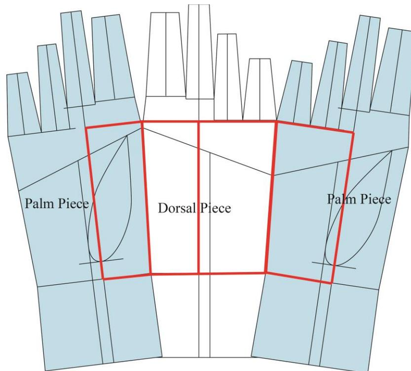
Figure 8.2 Part of glove pattern (red in colour) extracted for finite element analysis
