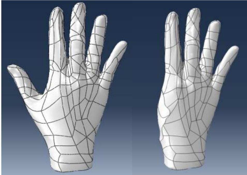
Figure 8.1 (a)Hand geometric model obtained from 3D scanning and (b)hand geometric model with thumb removed for use in pressure prediction model
