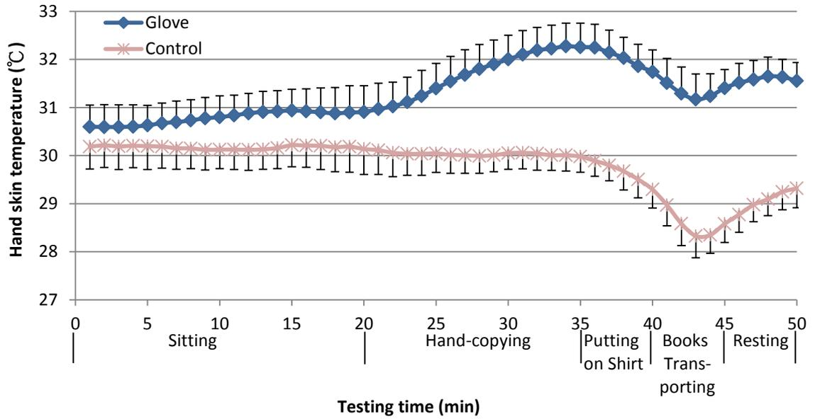
Figure 6.13 Overall hand skin temperature when pressure gloves are worn in the control condition (n=120, mean  $\pm$  SD)
