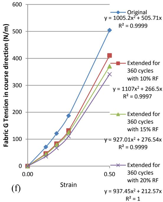
Figure 5.10 Stress/strain curves of (a) Fabric A in the wale direction, (b) Fabric A in the course direction, (c) Fabric D in the wale direction, (d) Fabric D in the course direction, (e) Fabric G in the wale direction, and (f) Fabric G in the course direction.
