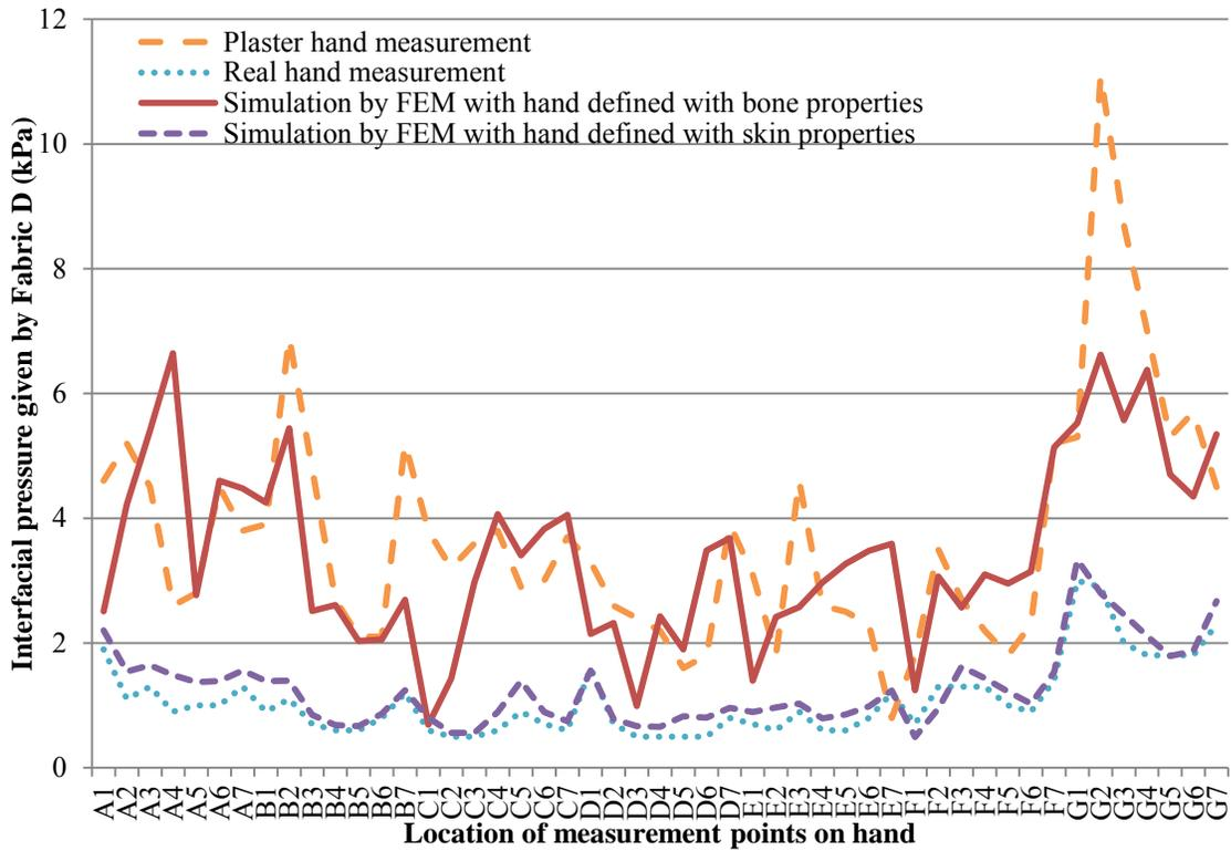
Figure 8.14 Comparison of simulated pressure from FEM and sensor measured pressure on plaster and real hands induced by glove made of Fabric D
