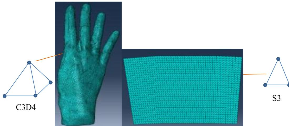
Figure 8.5 Meshed model of (a) hand and (b) glove fabric
