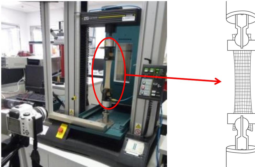
Figure 8.3 Experimental setting for determining the Poisson's ratio of a fabric
