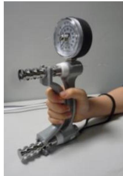
Figure 6.8 Dynamometer for gripping task
