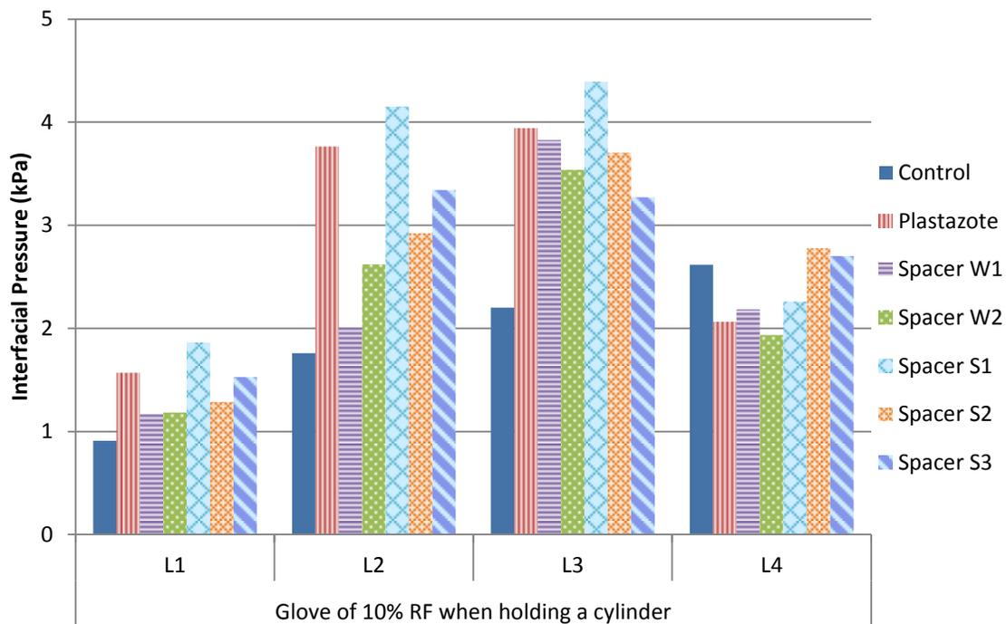
Figure 7.14 Interfacial pressures at 4 locations on the dorsum of the hand between the hand and the pressure gloves with 10% RF that have different inserts when the subject is holding a cylinder
