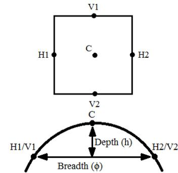
Figure 5.7 Five coordinates on a measured point to be obtained from a 3D image
