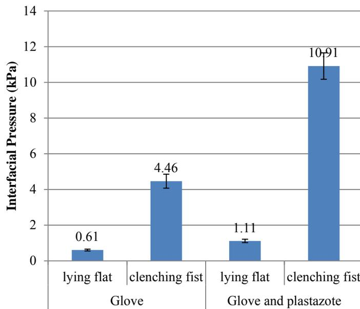
Figure 3.5 Glove-skin interfacial pressure when hand is laid flat and also when clenched. (Error bars indicate  $\pm$  standard errors)
