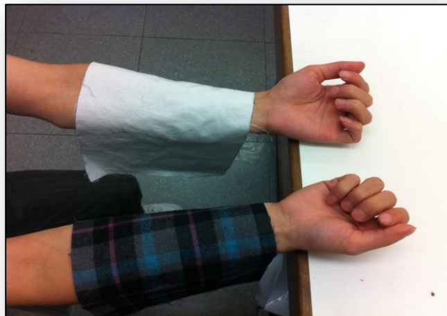
Figure 6-2 Illustration Figure of Passive Forearm Contact for Subjective Measurement
