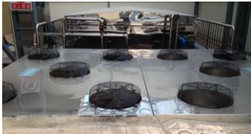
Figure 2-2 Environmental chamber consisting of heated water tanks and air ventilations
