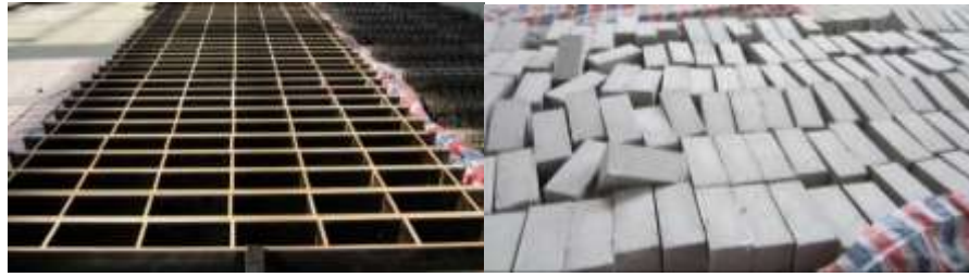
Figure 3-2 Mold frames and concrete prisms for bonded joint tests
