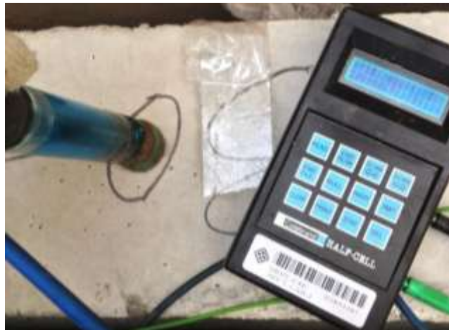
Figure 2-3 Test on half-cell potentials of steel reinforcement in RC beams
